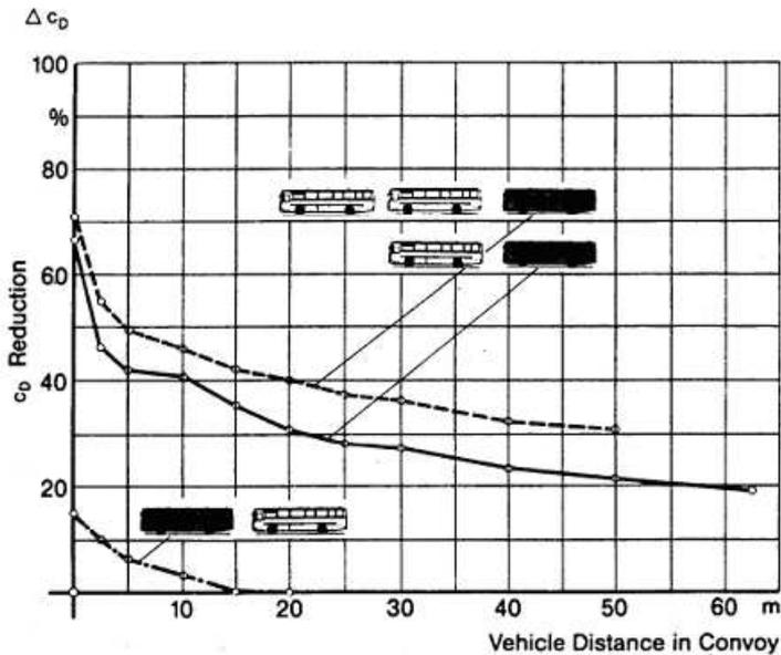
Figure 2.3. Reduction of  $c_D$  depending on the distance to the target,[5].
