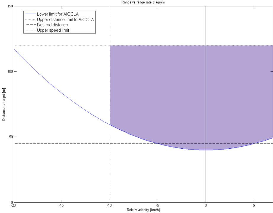
**Figure 3.3.** Range vs. range-rate diagram for time gap 2 seconds and target speed  $80\text{ km/h}$ .
