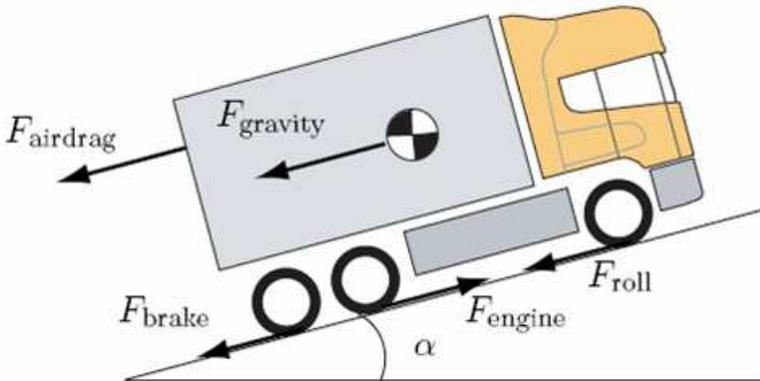
Figure 2.2. The longitudinal forces acting on a heavy vehicle.
