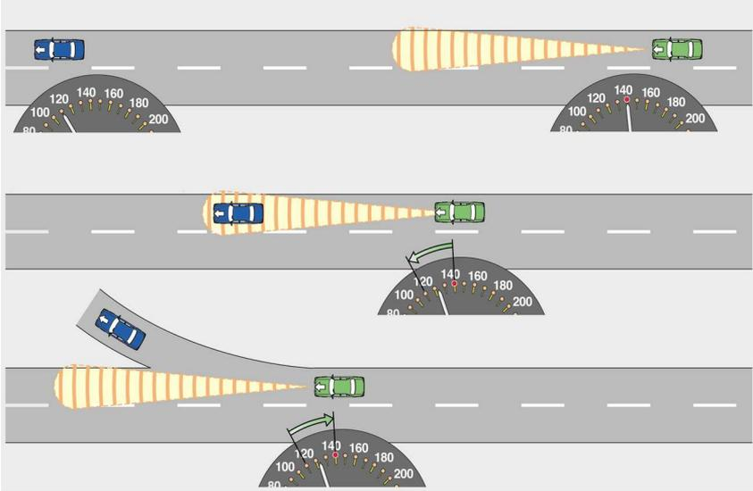
**Figure 1.1.** The function of an adaptive cruise control.
