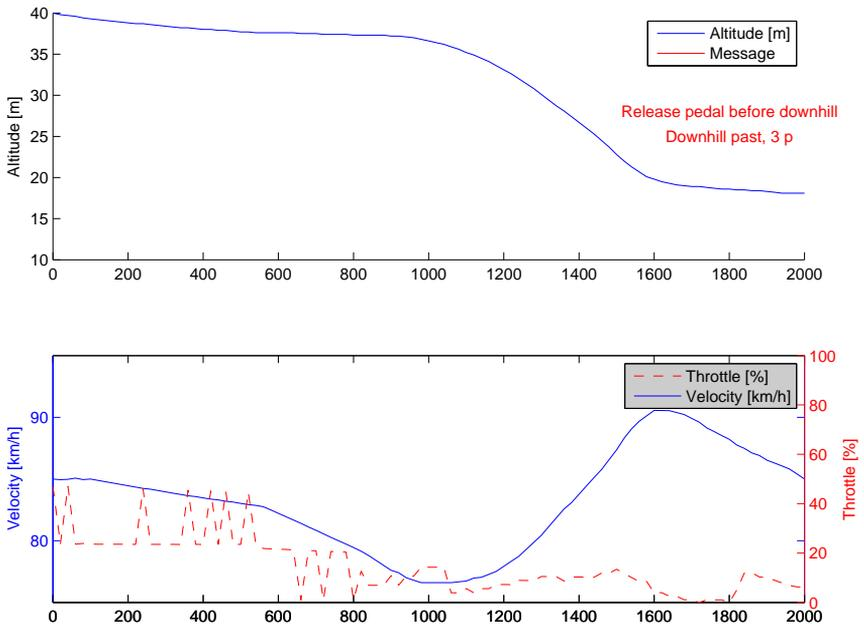
**Figure 6.5.** The IDT evaluation of the speed trajectory suggested by DPtool. The throttle is not released fully during the slowdown so the IDT system grades it lower, it expects a full release of the throttle.
