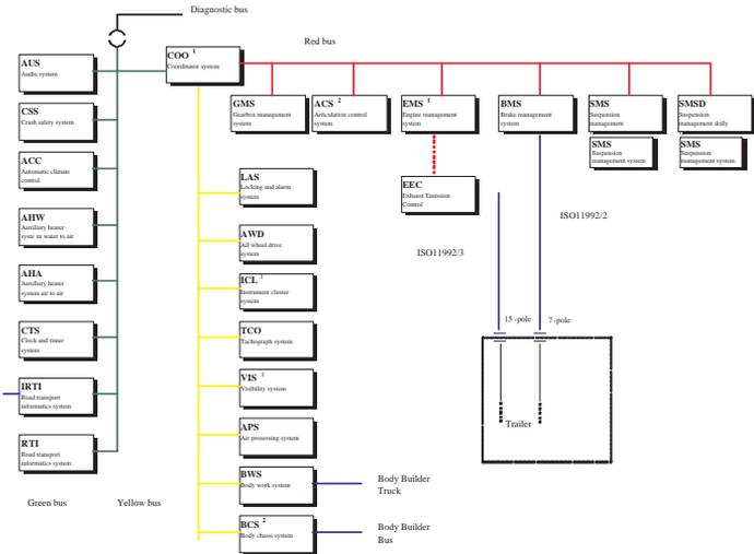
**Figure 5.2.** The ECU architecture of a Scania vehicle. The three busses are clearly separated to reduce the risk of network failure on all three busses but are all connected to the coordinator. Depending on the specification of the truck the number of ECUs change but the coordinator is always present.
