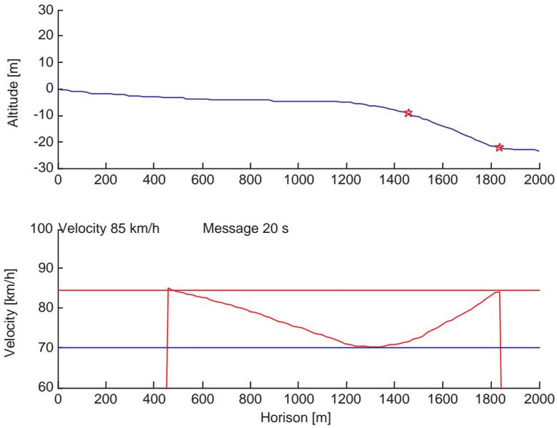
**Figure 4.4.** *The downhill is just long enough for the truck to regain its current speed if it is slowed down to the low set speed.*
