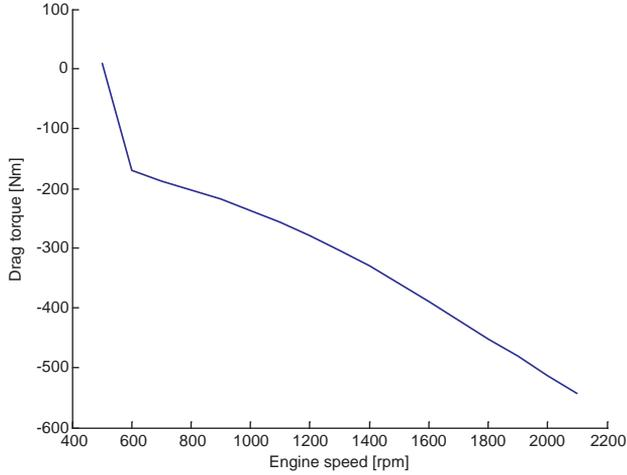
**Figure 3.3.** Drag torque at the flywheel as a function of engine speed. Note that the drag torque is zero at the idling speed (about 500 rpm) and that is when fuel is injected to prevent the engine from stalling.
