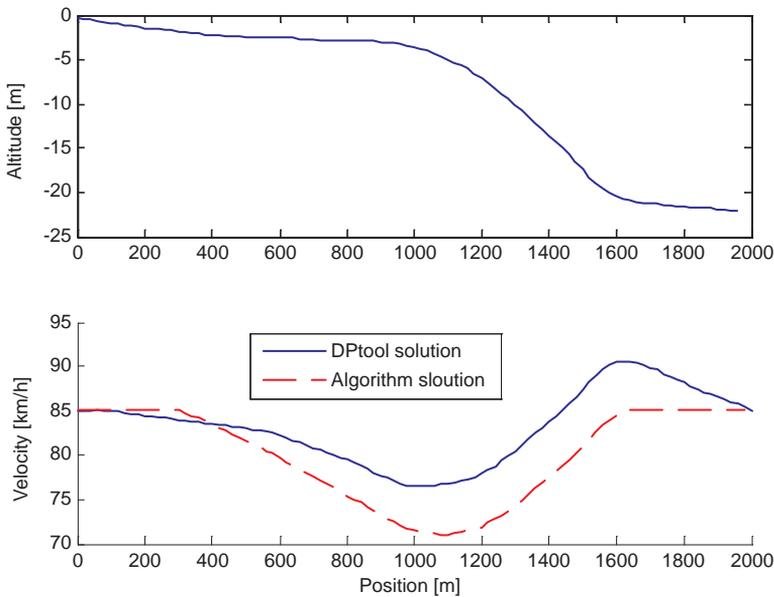
**Figure 6.3.** The trajectories of the DPtool solution and the solution of the algorithm over the same downhill described above. Note that the dynamic programming solution is faster than the solution proposed by the algorithm, 87.6 seconds and 90.4 seconds respectively.
