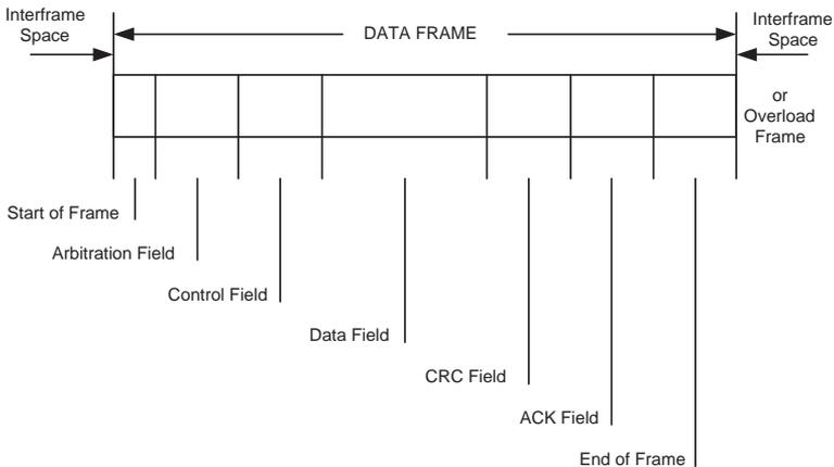
**Figure 5.1.** *The structure of a CAN message.*
