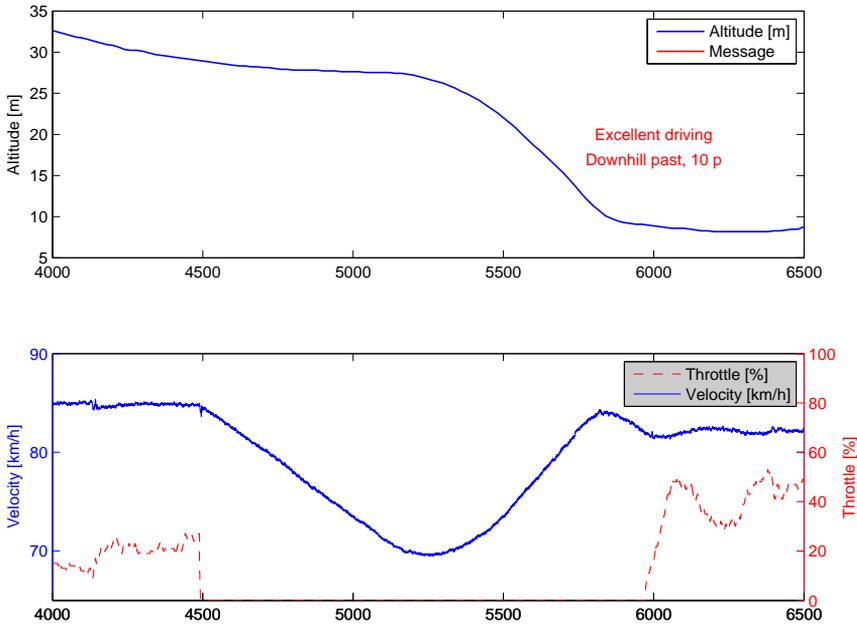
**Figure 6.4.** *The IDT evaluation of the test run. The test run has the same speed trajectory as the algorithm making the evaluation an indirect evaluation of the algorithm. Since the throttle is fully released during the slowdown and the following downhill the IDT system grades it higher.*
