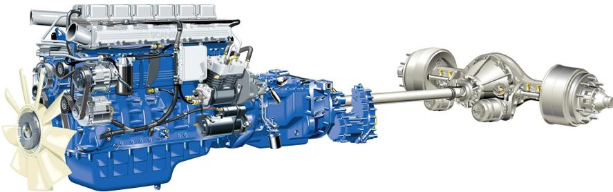
**Figure 3.1.** *Scania 12 litre driveline.*
