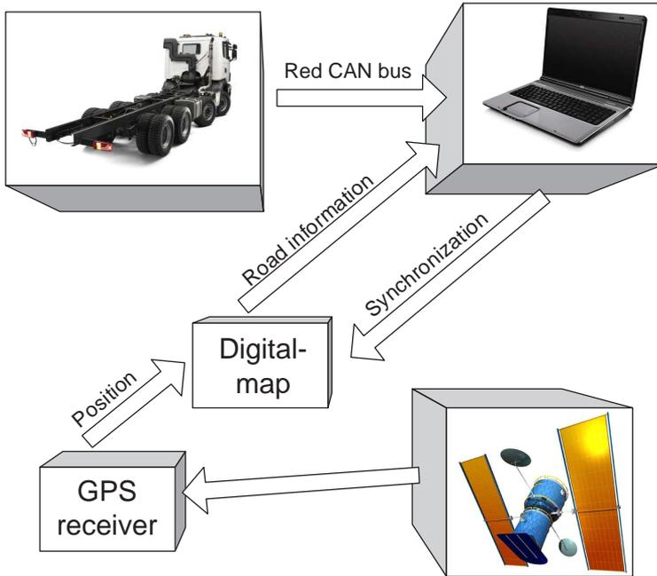
**Figure 5.3.** Architecture of the test. The GPS receiver feeds its position to the digital map unit. The digital map unit sends road information to the PC and the PC sends back how long the horizon is at the present and what road information is needed. The PC listens to the red CAN bus to get information from the vehicle.
