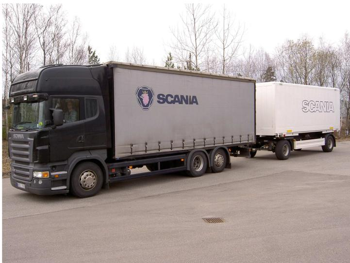
**Figure 5.4.** *Laboration vehicle "Montana" and trailer at the test track after completed testing. Length: 21m. Weight: 36 tonnes.*
