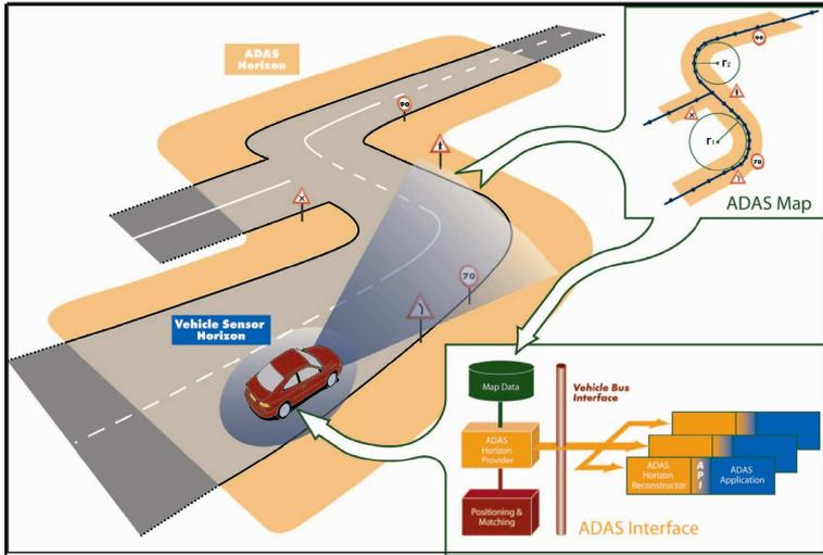
**Figure 1.1.** *The ADAS horizon concept. Note the possibilities represented in the figure, multiple path recognition, curve radius and traffic sign prediction, figure from [8].*
