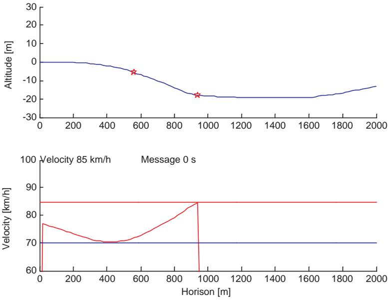
**Figure 4.5.** *The downhill is close enough for the driver to let go of the throttle now and still have more speed than the current speed.*
