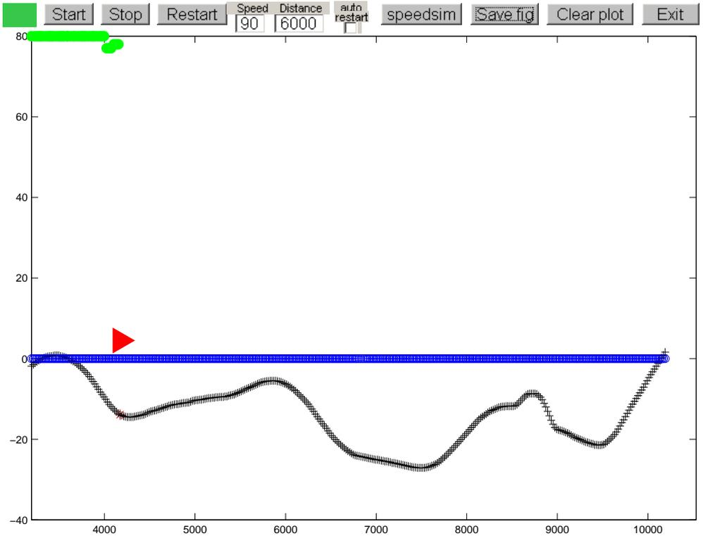
**Figure 5.5.** Screen dump of the program *Horizonviewer*. The arrow represents the position of the heavy truck. The black crosses represent the start and stop positions of the segments. The horizon length is set to 6000 meter in the screen dump, in the algorithm a horizon length of 2000 meter is utilized.
