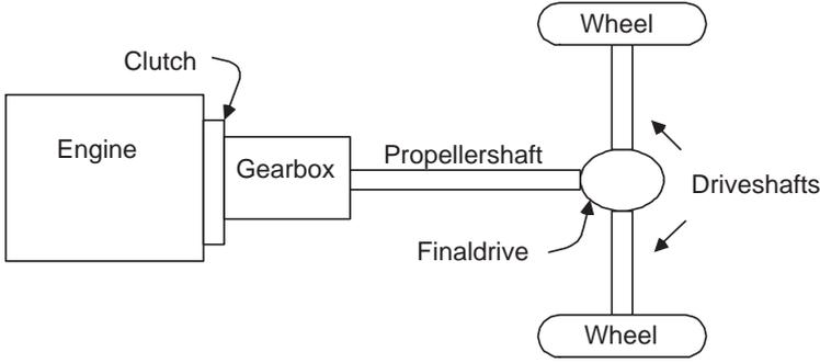
**Figure 3.2.** *The main parts of a heavy duty powertrain, as described by the model in this chapter.*
