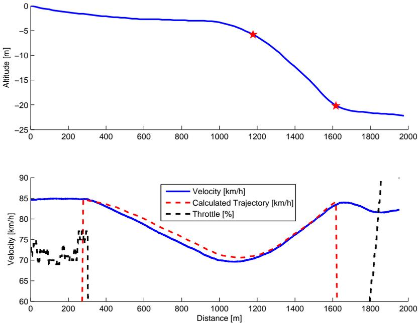
**Figure 6.2.** *The trajectories of the actual test and the suggested trajectories from the algorithm. The algorithms suggested fuel cut off point is 30 meter or 1.3 seconds in front of the test fuel cut off point. Estimation from the detection block is slightly off suggesting  $\alpha_{crit}$  being too big, the error can also come from the low resolution of the road slope in the digital map.*
