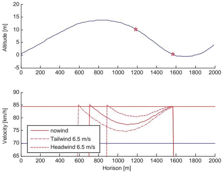
**Figure 6.7.** *Different speed trajectories with different ambient wind conditions calculated over a crest. The difference in time for the headwind and tailwind cases to the no wind case are 13 and -7 seconds respectively. Note that the downhill is not steep or long enough to regain initial speed from more than 77 km/h in the no wind case.*
