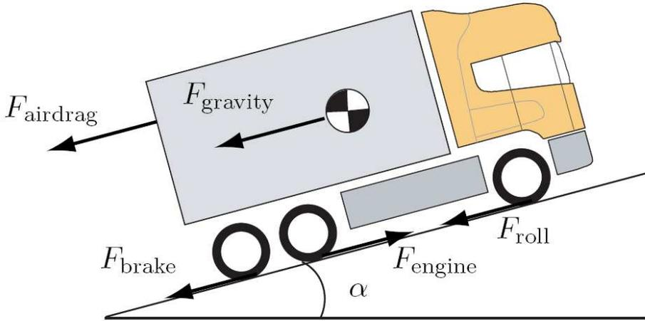
**Figure 3.4.** The longitudinal forces inflicted on a heavy duty vehicle in motion.
