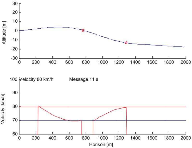
**Figure 4.3.** Note the gap in the calculated speed trajectory, the speed reached the low set speed in the calculation and it is restarted at the start of the slope. This trajectory will let the truck reach the low set speed at the beginning of the slope and the truck will accelerate to over the current speed in the downhill.
