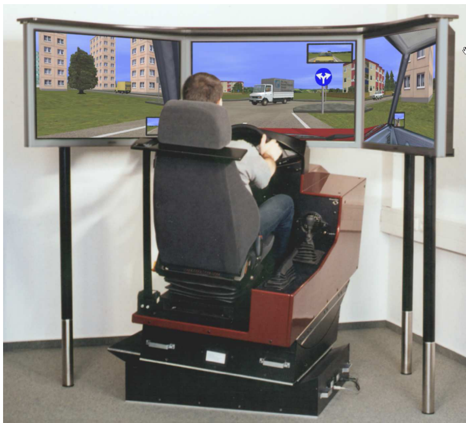
Figure 2.2: Photo of the Foerst Trainer simulator. Photo: Dr.-Ing Foerst GmbH.
