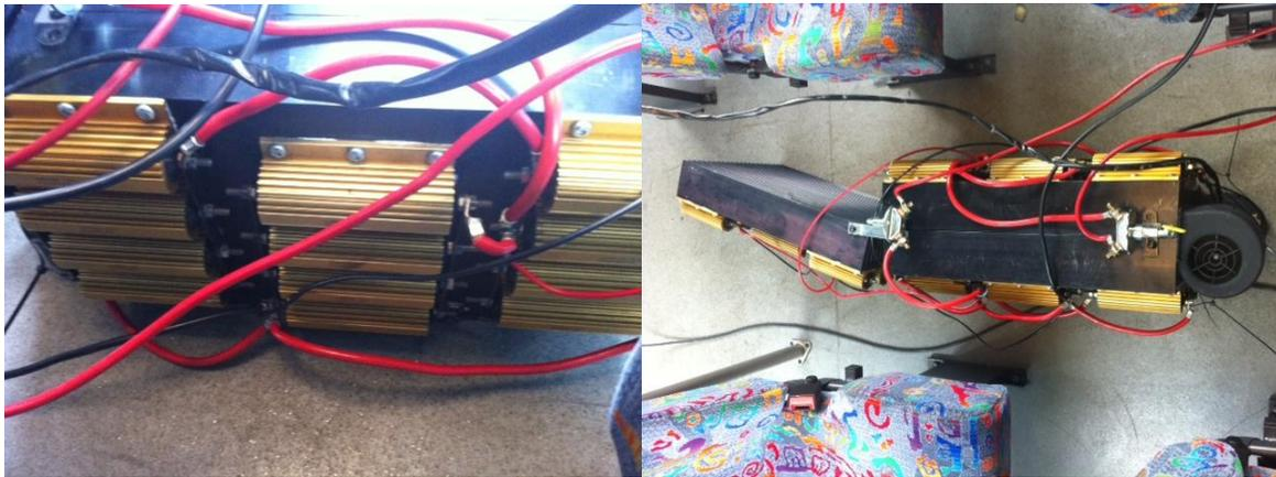
**Figure 6: The simulated air condition units, consisting of plates with power resistances and a fan, cooling the plates.**
