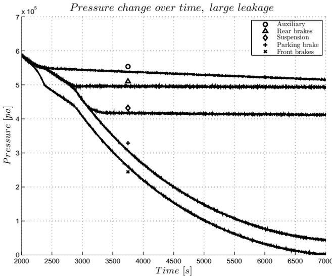
**Figure 4.15.** Pressure drop for a truck with a large leakage in the front brake circuit. The parking brake circuit also loses pressure because the connection with the front brake circuit via a bypass bleed.
