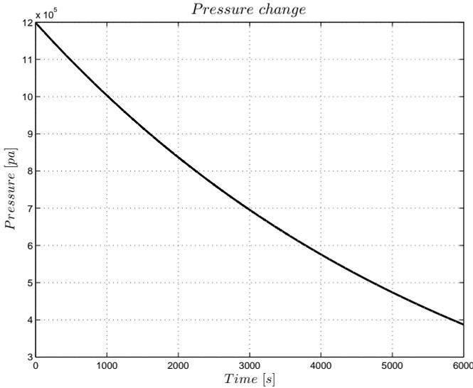
**Figure 4.8.** Simulated pressure drop for a 100 litre tank with a 10 litre/minute leakage. The pressure has decreased to 8 bar after about 2000 seconds. The first estimation in the diagnosis algorithm must be performed before the pressure is below 8 bar.
