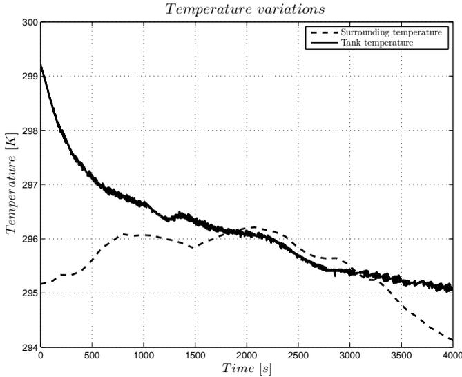
**Figure 5.16.** Temperature measured in the tanks compared to the surrounding temperature, for Leakage 2. The tank temperature drops during the first 2000 seconds while the surrounding temperature increases. This difference affects the result in the estimation if the tank temperature is approximated with the surrounding temperature, compare Figure 5.4 and Figure 5.15.
