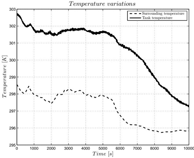
Figure 5.12. Temperature measured in the tanks compared to the surrounding temperature, for no implemented leakage. The temperatures look similar except for an offset.
