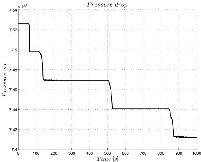
**Figure 4.19.** Pressure on CAN given by pressure sensors on the APS. The signal is limited to discrete levels which gives a signal with the shape of a step function.
