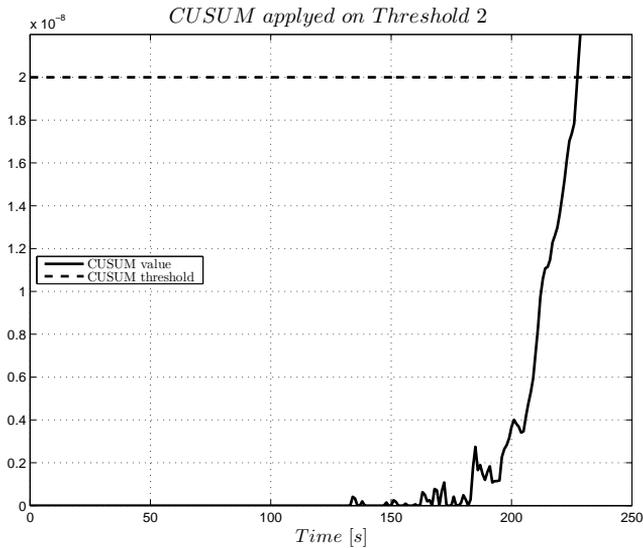
**Figure 4.14.** CUSUM applied to the estimated area and threshold 2 in Figure 4.12 by creating a residual as described by (4.5). Since the estimated area is larger than the threshold most of the time, the CUSUM gives the desired results with an alarm since the CUSUM gets larger over time and the CUSUM threshold in this example is exceeded after a short period of time.
