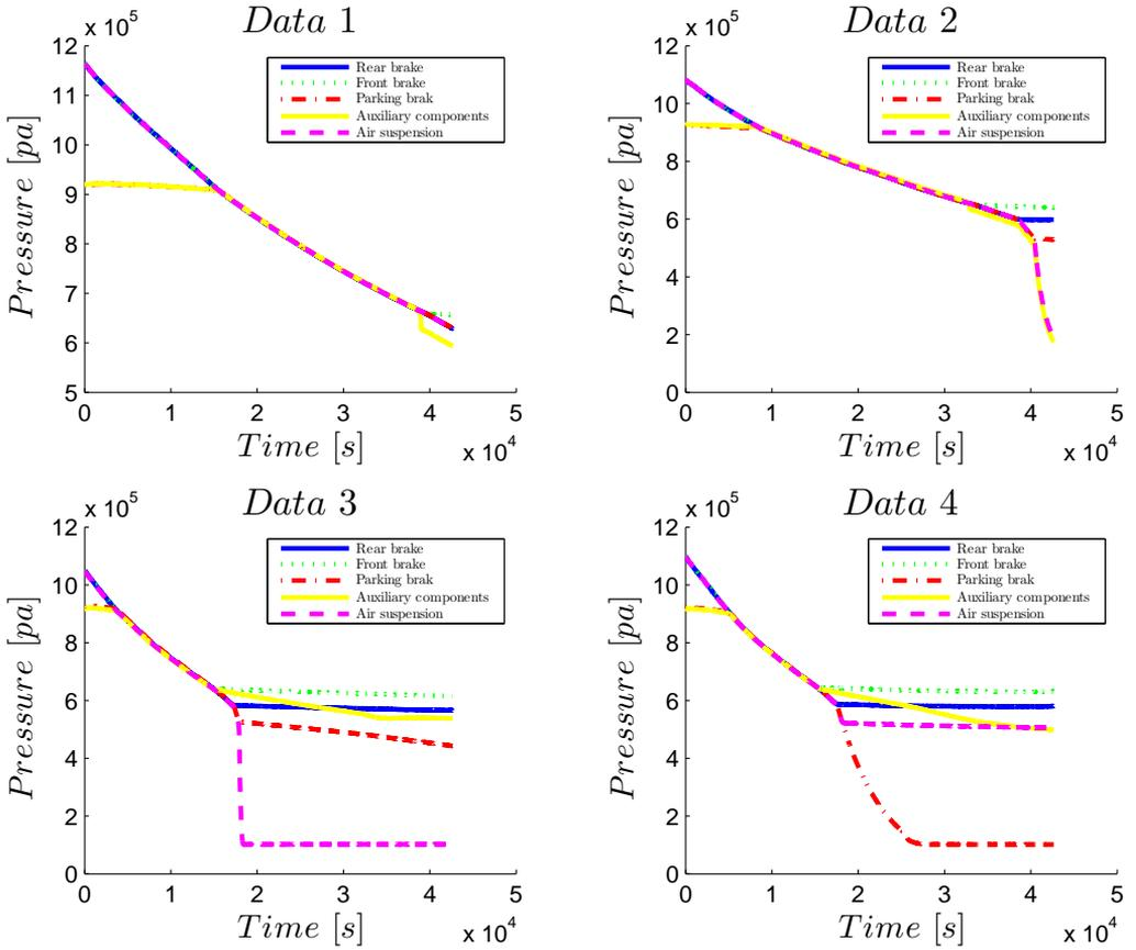
Figure A.1. Pressure drops corresponding to Data 1-4 used in Table 4.2 and Table 4.3.
