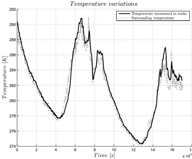
**Figure 3.2.** Temperature measured in the pressure tanks and the surrounding temperature.
