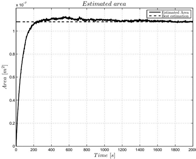
**Figure 5.17.** Estimated leakage area, using the surrounding temperature, for Leakage 3. There is a small overshoot in the beginning of the estimation compared to Figure 5.7. This is because the temperature in the tanks is decreasing in the beginning which the surrounding temperature does not, see Figure 5.18.
