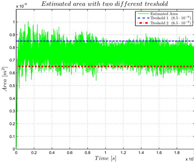
**Figure 4.12.** Estimated leakage area and two different possible thresholds. The estimation is most of the time over the lower threshold but under the higher threshold. If the lower threshold is used it is desired that the alarm is set since the estimated area in general is above the threshold. If the higher threshold is used the alarm should not be given since the estimation in general is below the threshold.
