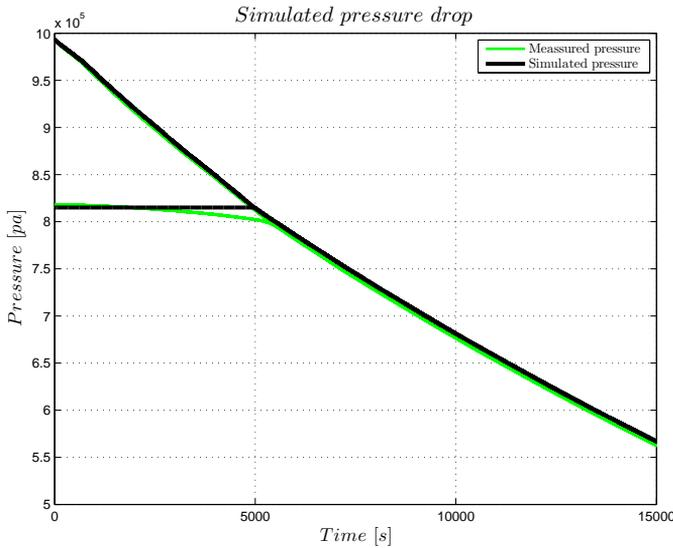
**Figure 5.3.** Simulated pressure drop using the estimated area, Leakage 1. The simulated pressure drop is close to the measurements which indicate that the model and estimation of the leakage area are good.
