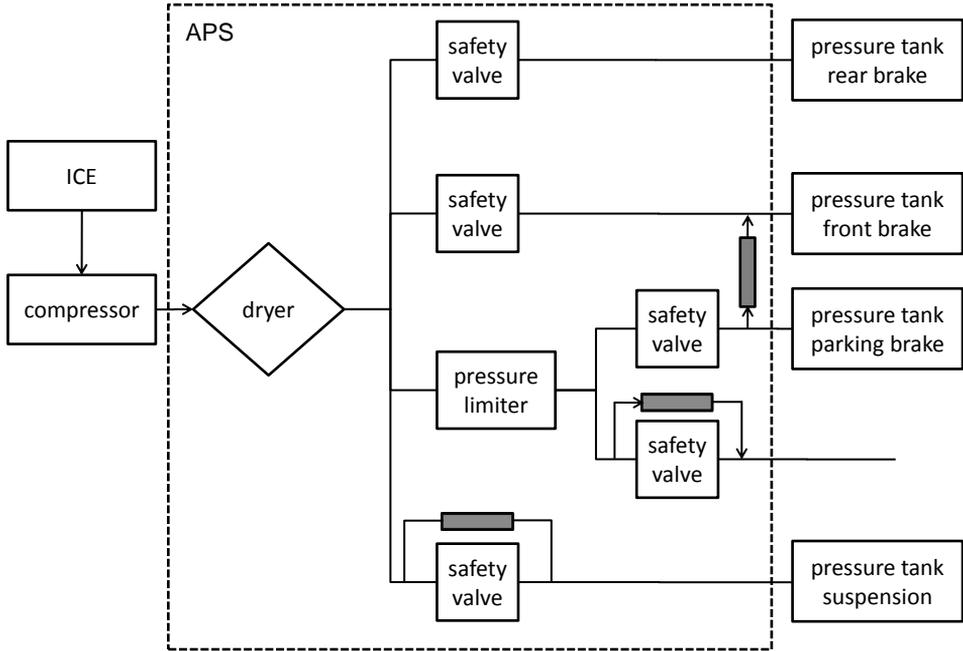
**Figure 1.1.** Circuit diagram for the APS with compressor, attached to the internal combustion engine, and connected pressure tanks. The filled blocks without text represents bypass bleeds and the arrows indicates the flow direction. Bypass bleeds without arrows allow air to flow in both directions. The circuit without pressure tank is the auxiliary circuit.
