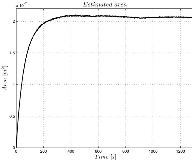
**Figure 5.19.** Estimated leakage area, using the surrounding temperature, for Unknown leakage. The estimation is similar to the estimation in Figure 5.9. There is a difference between the surrounding temperature and the tank temperature in the beginning of the estimation, see Figure 5.20. However, the temperatures are almost the same after 400 seconds which is when the filter has reached its maximum value.
