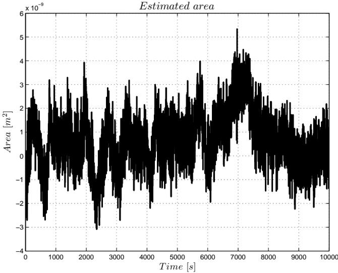
**Figure 5.1.** Estimated leakage area without any implemented leakage. The estimated leakage area is always below the threshold value of  $8.5 \cdot 10^{-9} \text{ m}^2$  which is the size of a 1 litre/minute leakage.
