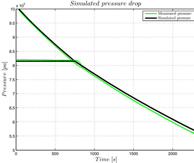
**Figure 5.8.** Simulated pressure drop using the estimated area, Leakage 3. The simulated pressure drop is a little slower than the measurements. The reason can be that the estimated area is a little too small.
