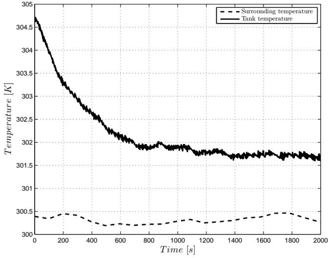
**Figure 5.18.** Temperature measured in the tanks compared to the surrounding temperature, for Leakage 3.
