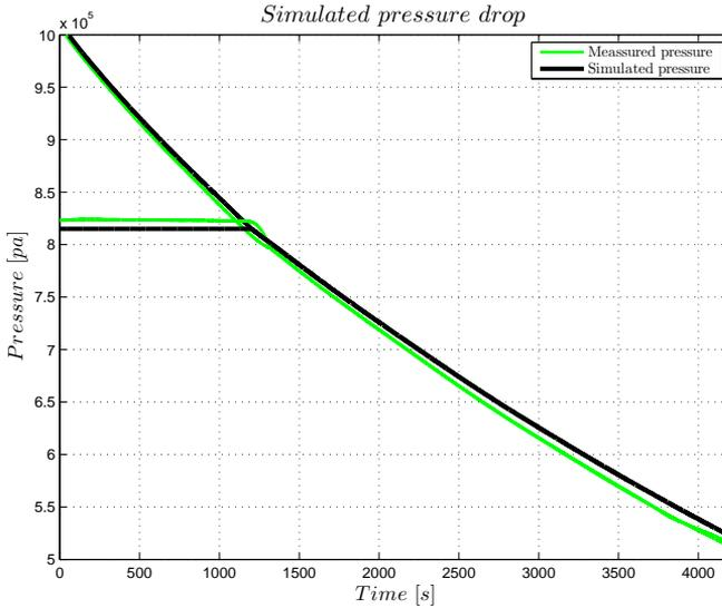
**Figure 5.5.** Simulated pressure drop using the estimated area, Leakage 2. The simulated pressure drop is a little slower than the measured pressure. One explanation is that the estimated leakage area is a little too small.
