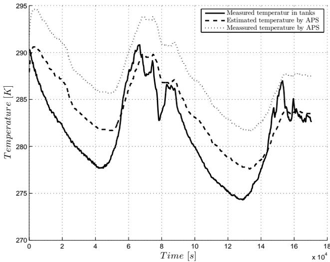
**Figure 4.21.** Temperature measured with sensors in pressure tanks, temperature sensor on APS and estimated temperature for the regeneration valve.
