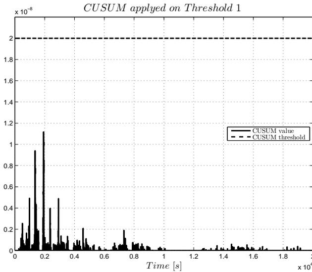
**Figure 4.13.** CUSUM applied to the estimated area and threshold 1 in Figure 4.12 by creating a residual as described by (4.5). Since the estimated area is lower than the threshold most of the time, the CUSUM gives the desired results with no alarm since the CUSUM threshold is not exceeded.
