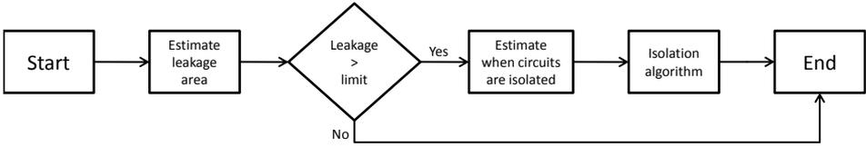
**Figure 4.1.** Overview flow chart for the diagnosis algorithm. The algorithm starts after the APS has regenerated. First an estimation of the total leakage area in the system is performed. If the leakage size is larger than a predetermined limit the algorithm estimates when the safety valves have closed. When the safety valves have closed, it is possible for the isolation algorithm to point out which circuit that leaks the most.
