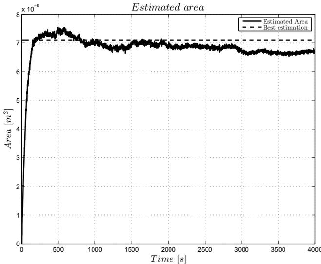
**Figure 5.15.** Estimated leakage area, using the surrounding temperature, for Leakage 2. There is an overshoot in the beginning in the estimations because of the use of surrounding temperature as approximation of the temperature in the tanks. The estimation is close to the estimation in Figure 5.4 after 2000 seconds. This is the time for when the surrounding and tank temperature has the same value, see Figure 5.16.
