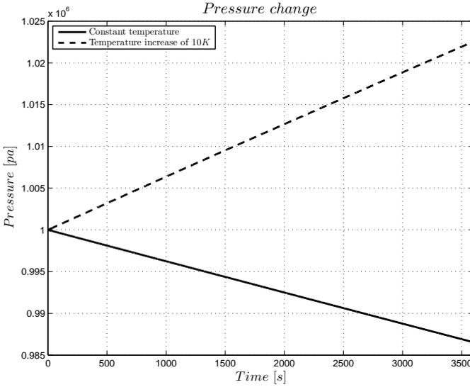
**Figure 3.5.** Simulated pressure change for a  $100dm^3$  tank with a hole of  $0.05mm\varnothing$ . The temperature increases linear over time.
