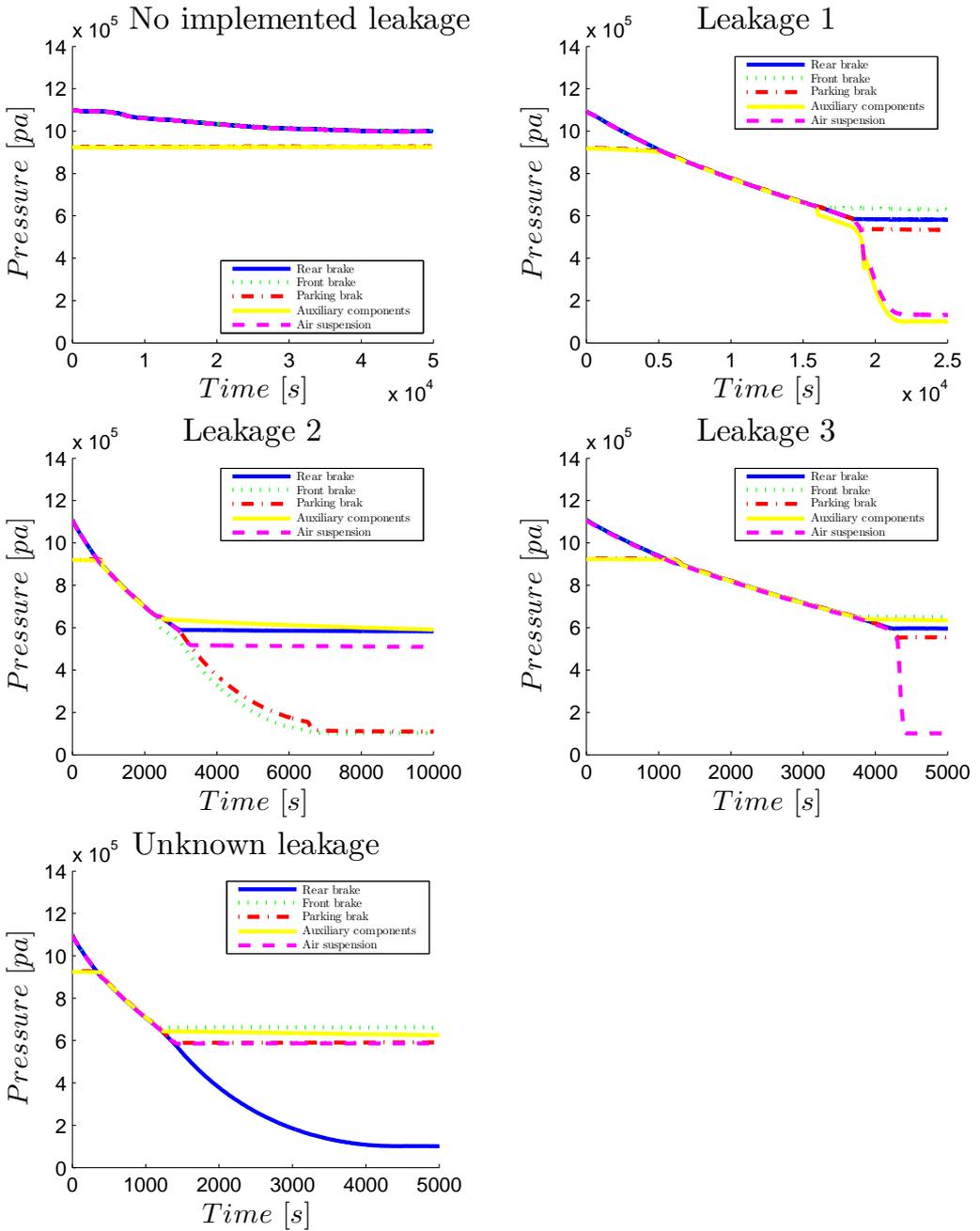
Figure A.3. Pressure drops for data used in the validation.
