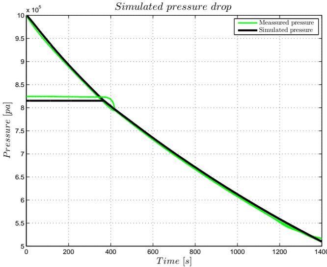
**Figure 5.10.** Simulated pressure drop using the estimated area, Unknown leakage. The simulated pressure drop is similar to the measured pressure. This shows that the model and estimation of the area works good also for a little larger leakages.
