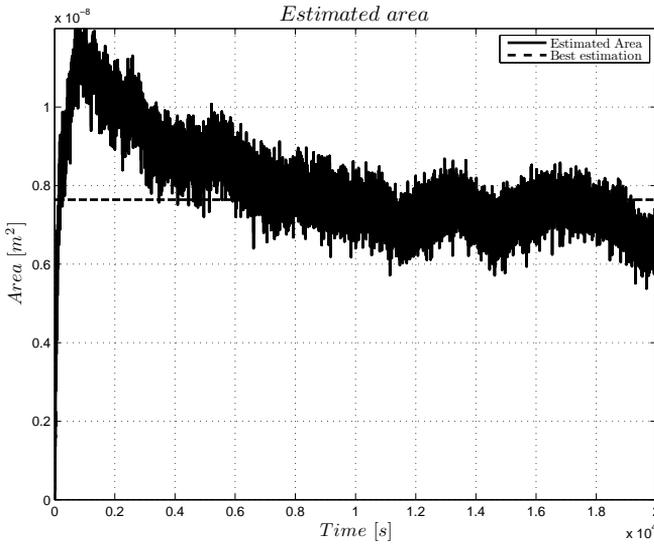
Figure 4.2. Estimated leakage area without temperature compensation. The estimation deviates from the best estimation in the beginning because of the constant temperature assumption.
