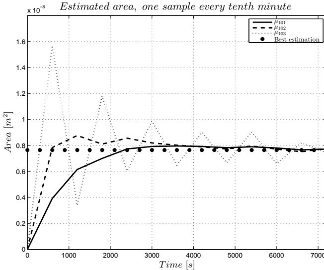
**Figure 4.9.** Estimated leakage area taking one sample every tenth minute. The magnitude of the leakage is around 1 litre/minute. The largest filter constant  $\mu_{103}$ , gives an oscillating estimation. The smallest filter constant  $\mu_{101}$ , seems to give a stable estimation but takes long time to reach its final value. The medium size of the filter parameter  $\mu_{102}$ , gives a fast estimation with only small oscillations.
