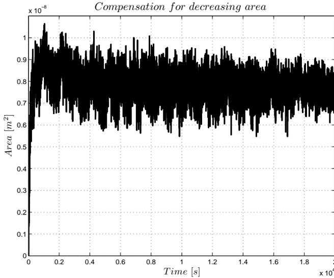
**Figure 4.18.** The estimated leakage area with compensation for decreasing area when the pressure in the system drops. The same estimation without compensation is shown in Figure 4.4.
