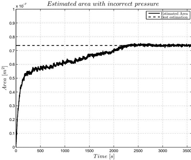
**Figure 4.5.** Estimated leakage area using the incorrect pressure. The error in the estimation decreases when the pressure in the high pressure tanks decreases. At 2300 seconds the pressure is the same in the high and low pressure circuits.
