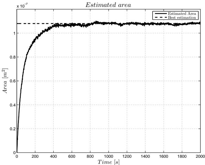
**Figure 5.7.** Estimated leakage area with implemented leakage and expected result, Leakage 3. The estimation is very close to the expected result which indicates that the estimation algorithm is good.
