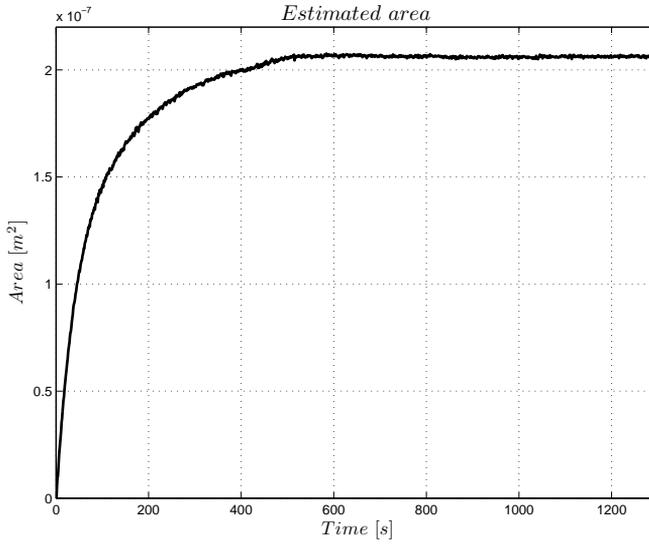
**Figure 5.9.** Estimated leakage area with implemented leakage and expected result, Unknown leakage. The estimation is stable after the settling time and does not have any oscillations or drift.
