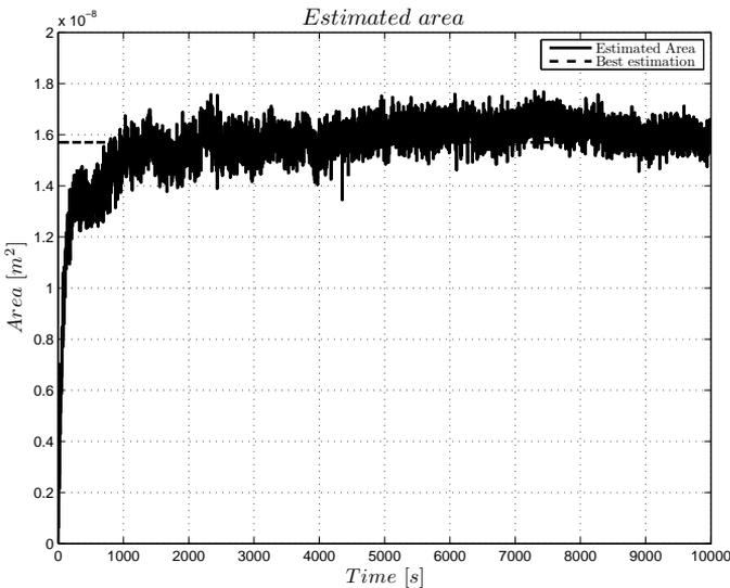
Figure 5.13. Estimated leakage area, using the surrounding temperature, for Leakage 1. The estimated area has a small positive drift because the leakage is in a low pressure circuit. The estimation is similar to the estimation in Figure 5.2.
