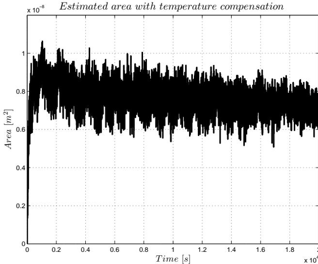
**Figure 4.4.** Estimated leakage area with temperature compensation. The estimation is better during the change of the temperature (Figure 4.3), compared to Figure 4.2.
