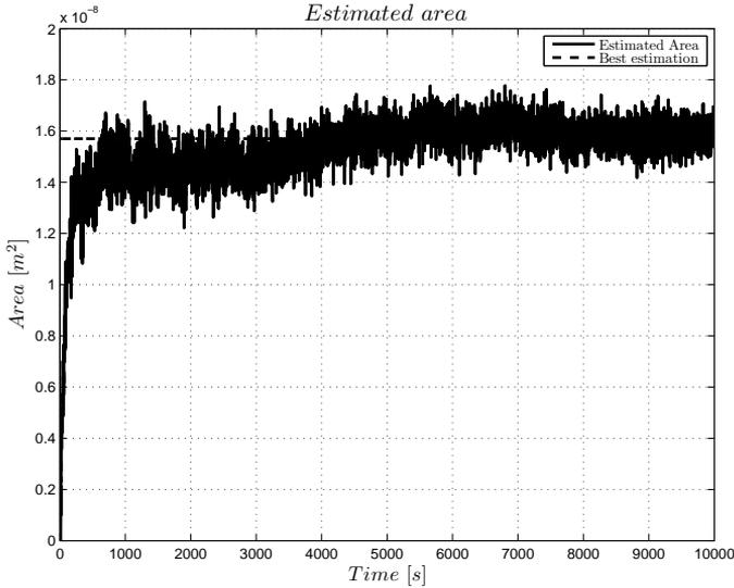
**Figure 5.2.** Estimated leakage area with implemented leakage and expected result, Leakage 1. A small drift can be seen in the estimation. The drift in this case indicates that the leakage is in a low pressure circuit, since the pressure in the high pressure circuits has been used in the estimation. The drift stops after 6000 seconds since the pressure in the high pressure circuits have decreased below 8 bar.
