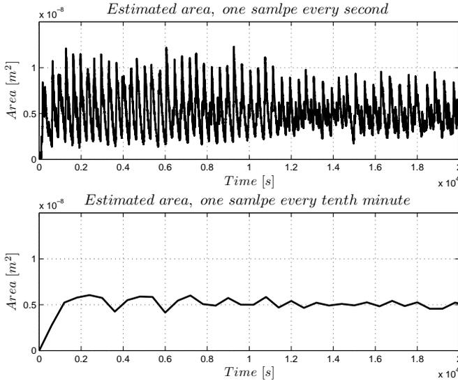
**Figure 4.20.** Estimated leakage area using the pressure sensors of the APS. The estimation on the top is from using a sample time of 1Hz which gives large spikes every time the signal in Figure 4.19 makes a step. The estimation below is made with the same signal but with taking one sample every tenth minute. By spreading out the samples the spikes in the estimation is decreased.
