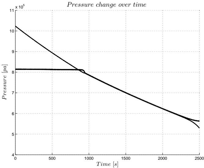
**Figure 4.11.** Pressure drop for a truck with an implemented leakage with the size of about 10 litre/minute. The pressure has decreased to 8 bar after 1000 seconds and the circuits starts isolating after 2500 seconds. The slowest filter constant that can be used must reach its final value within 2500 seconds to give the correct result. To be able to do the isolation between the high and low pressure circuits the first estimation must be within the first 800 seconds.
