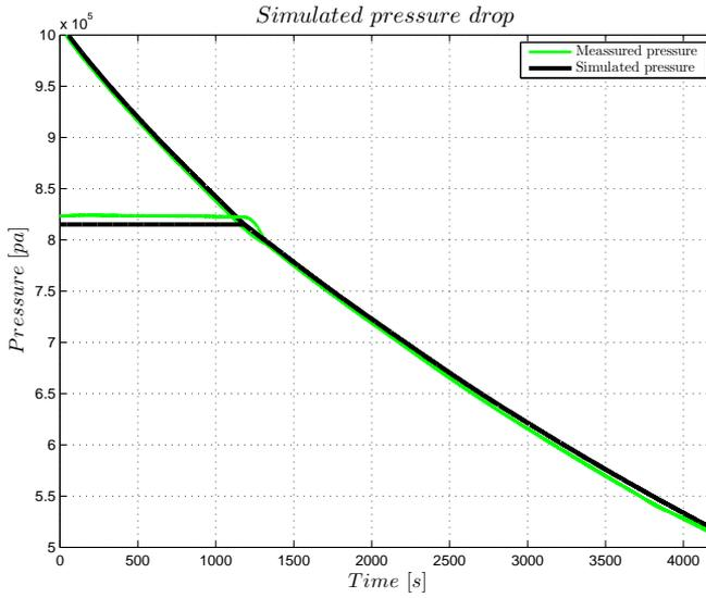
**Figure 5.6.** Simulated pressure drop using the estimated area from the first estimation  $A_1$ , Leakage 2. The simulated pressure drop is almost identical with the measurements. This indicates that  $A_1$  is a better estimation of the leakage area than  $A_2$ , see Figure 5.5.
