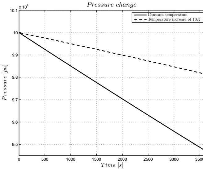
**Figure 3.4.** Simulated pressure change for a  $100dm^3$  tank with a hole of  $0.1mm\varnothing$ . The temperature increases linear over time.
