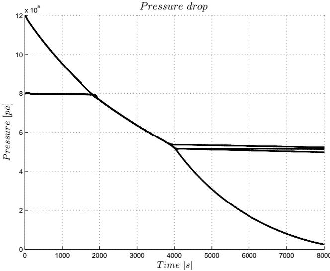
**Figure 3.1.** A common air pressure change for a leaking heavy truck. In the start the pressure is higher in the high pressure circuits than in the low pressure circuits. When the air leaks out, the pressure in the high pressure circuits decreases. After a while the pressure is the same in all circuits. When the safety valves closes the pressure remains in the non-leaking circuits, and decreases in the leaking circuits.
