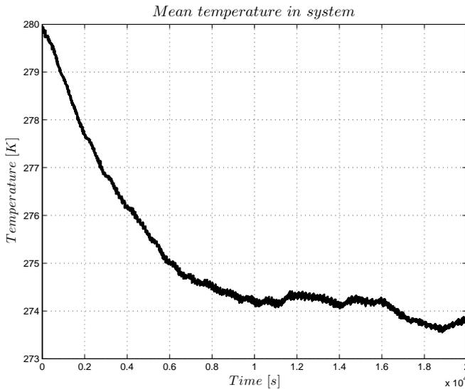
Figure 4.3. Measured temperature in tanks. In the beginning of the test the surrounding temperature decreases, causing the air temperature in the tanks to decrease.
