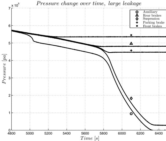
**Figure 4.16.** Pressure drop for a truck with a large leakage in the auxiliary circuit. The suspension circuit also loses pressure because the connection with the auxiliary circuit with bypass bleeds.
