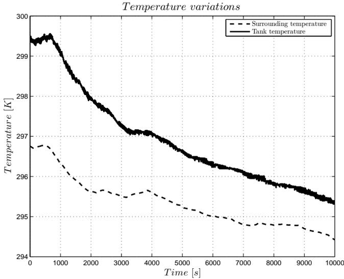
**Figure 5.14.** Temperature measured in the tanks compared to the surrounding temperature, for Leakage 1. The temperatures are similar except for an offset.
