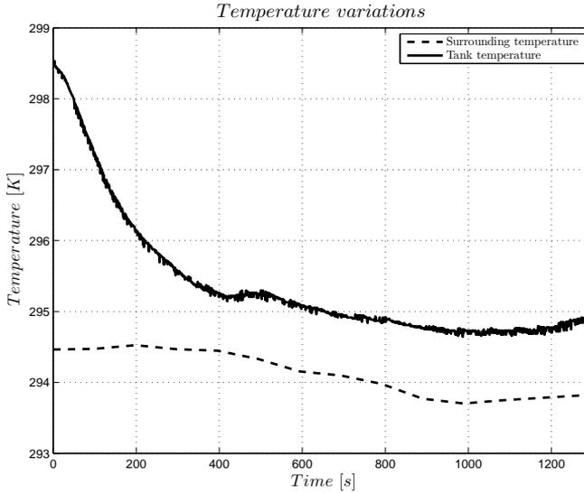
**Figure 5.20.** Temperature measured in the tanks compared to the surrounding temperature, for Unknown leakage. There is a difference in the beginning between the surrounding temperature and the air temperature in the tanks. The temperatures are almost equal after 400 seconds.
