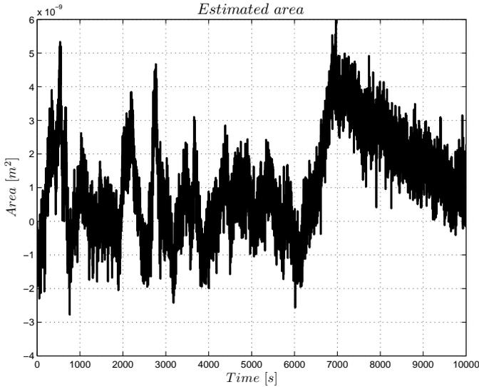
**Figure 5.11.** Estimated leakage area, using the surrounding temperature, without any implemented leakage. The estimated leakage area is always below the threshold value of  $8.5 \cdot 10^{-9} \text{ m}^2$ , which is the size of a 1 litre/minute leakage.
