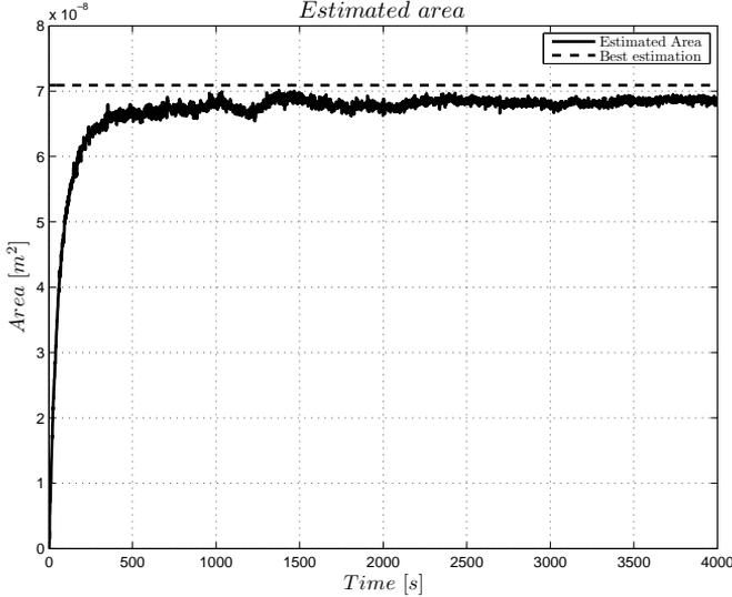
**Figure 5.4.** Estimated leakage area with implemented leakage and expected result, Leakage 2. The estimation is below the expected value which tells that the leakage seems to give a little less air leakage than expected.
