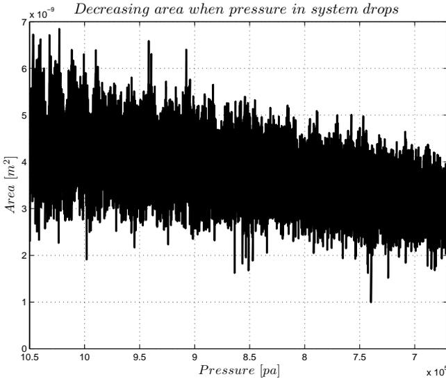
**Figure 4.17.** The estimated area decreases when the pressure in the system drops.
