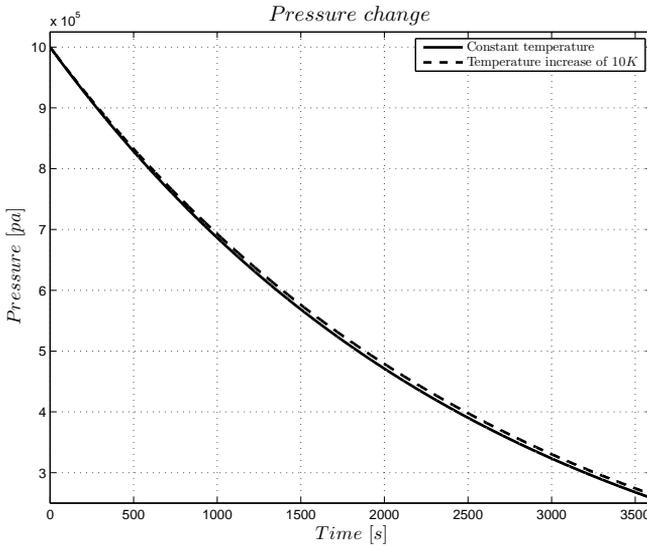
**Figure 3.6.** Simulated pressure change for a  $100dm^3$  tank with a hole of  $0.5mm\varnothing$ . The temperature increases linear over time.
