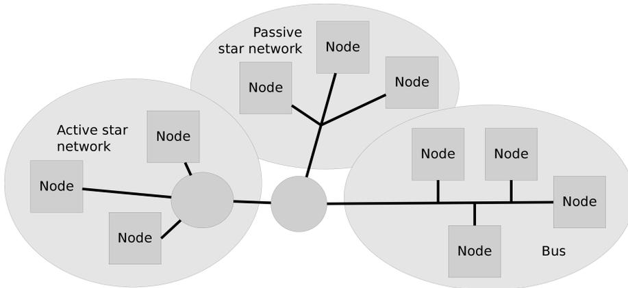
**Figure 2.6:** A hybrid network consisting of an active star network, a passive star network and a linear bus. What makes it a hybrid network is that its characteristics differs from that of a standard topology.
