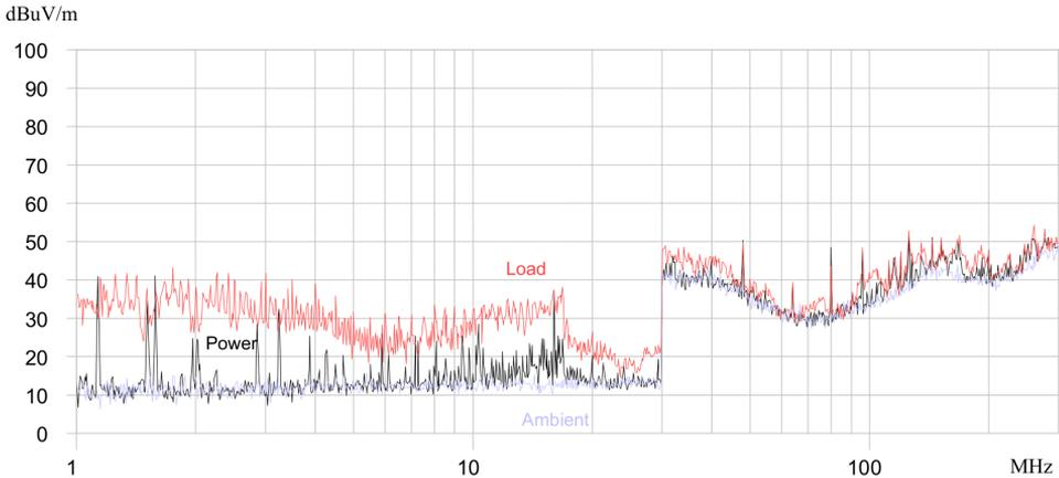
**Figure 5.4:** Emission spectrum from a Scania ECU using J1939, 1-300 MHz. The step is due to the change in resolution bandwidth. The increase in emission is relatively evenly distributed for lower frequencies. Power feeding the unit or sending data does not affect the spectra to any greater extent for frequencies over 30 MHz.
