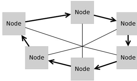
**Figure 3.14:** D2B ring network with wake-up lines controlling the wake-up and sleep state of the nodes. This is used because of the high current usage of the optic transceivers.
