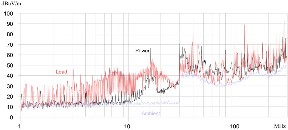
**Figure 5.7:** Emission spectrum from high-speed CAN measurements on the SofTec evaluation board, 1-300 MHz. The step is due to the change in resolution bandwidth. The low-speed and high-speed CAN spectra shows some similarities, the spikes at lower frequencies among others.
