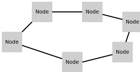
**Figure 2.7:** A ring network consisting of six nodes resulting in five interconnections. A node is said to be active if it modifies the received data and passive if it just passes it on to the next node.
