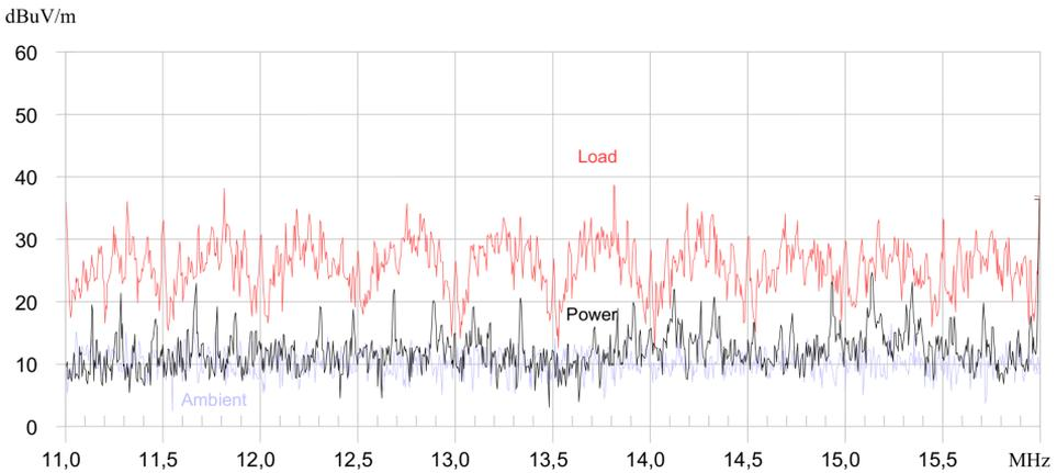
**Figure 5.5:** Emission spectrum from a Scania ECU using J1939, 11-16 MHz. The resonance frequencies can be seen in this plot in the pattern repeated every 500 Hz.
