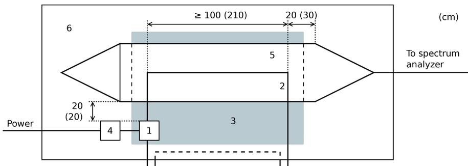
**Figure 5.6:** Test setup for CAN and LIN tests. The return wire is routed under the ground plane to prevent it from affecting the measurements. (1) Evaluation board, (2) Wire, (3) Insulating base, (4) LISN, (5) Stripline antenna, (6) Ground plane
