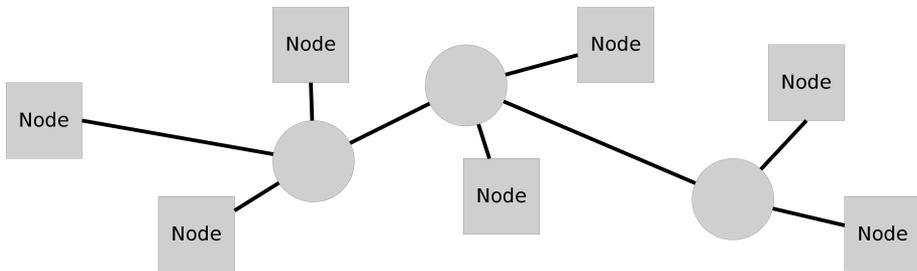
**Figure 2.5:** Three cascaded active stars with a total of seven nodes. The active star nodes can act as repeaters over long distances. This does however add extra propagation delay throughout the network.
