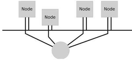
**Figure 3.2:** Example of a FlexRay two-channel layout. The channels are connected using a linear bus and an active star network respectively.
