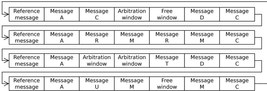
**Figure 3.7:** Four TTCAN basic cycles, each one of them starting with a reference message containing timing information and cycle count. The first cycle starts again as soon as the last one finishes.
