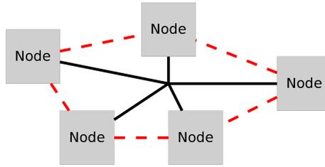
*Figure 3.12: A logical ring network implemented on a physical star network.*
