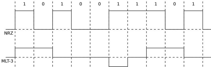
**Figure 3.9:** MLT-3 encoding based on three voltage levels. A logical one is represented by a change in voltage and a logical zero by a constant signal level.
