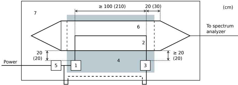
**Figure 5.10:** Test setup for FlexRay test. Two evaluation boards has been used in this test, both power fed through the LISN.
