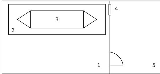
**Figure 5.1:** The test environment at Scania consisting of two shielded rooms connected by a cable duct. The stripline antenna is located in the left chamber in the figure and the power supply, spectrum analyzer and computers in the right.
