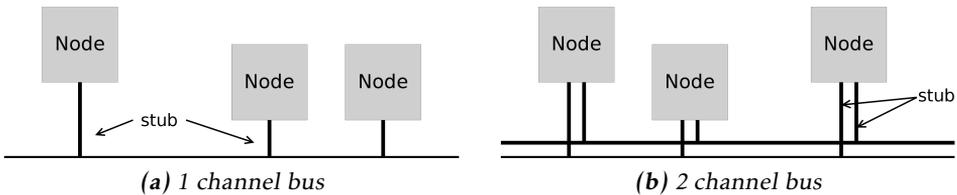
**Figure 2.3:** Example of bus networks. These are small, cheap and easy to extend by just adding a node to the shared wire. The stubs can give rise to signal reflections and should be kept to a minimum.
