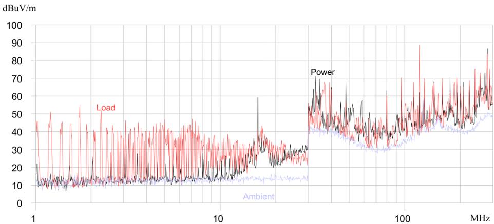
**Figure 5.8:** Emission spectrum from low-speed CAN measurements on the SofTec evaluation board, 1-300 MHz. The step is due to the change in resolution bandwidth. The spectrum, especially the spikes at lower frequencies, reassembles that of high-speed CAN except for the signal levels.
