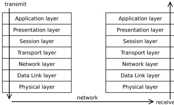
**Figure 2.1:** The Open Systems Interconnect (OSI) model. The seven hierarchical levels can be clearly seen with the application layer closest to the end user. The transmission and reception of a message can also be seen in the figure.
