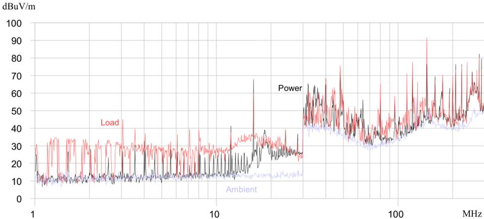
**Figure 5.9:** Emission spectrum from LIN measurements on the SofTec evaluation board, 1-300 MHz. The step is due to the change in resolution bandwidth. A difference to the tested CAN interfaces can be seen at lower frequencies where the spikes are broader. The emission levels are also more even over the whole spectrum.
