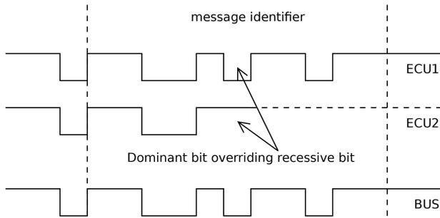
**Figure 2.11:** CSMA/CR and CSMA/CA arbitration. ECU 1 has a lower valued message identifier and thereby a higher priority on the network. As soon as one of its dominant bit overrides a bit sent by ECU 2 the latter stops transmitting.
