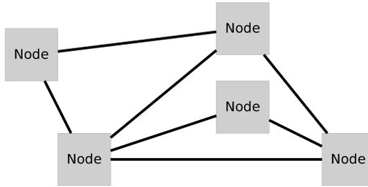
**Figure 2.2:** Point-to-point interconnections between five nodes. The wiring grows rapidly when the number of nodes increases. This led to the use of other network topologies such as the bus.
