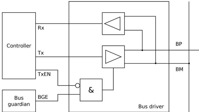
**Figure 2.14:** Schematic figure of a local bus guardian. The TX enable signal reaching the transceiver is controlled by the Bus Guardian Enable signal to prevent the node from becoming a “babbling idiot”.
