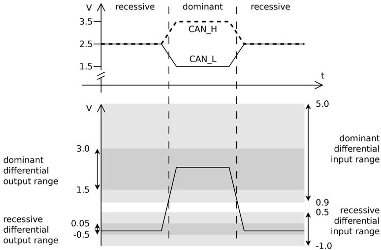
**Figure 3.1:** CAN signal showing two recessive and one dominant bit on its two wires, CAN\_L and CAN\_H. The ranges of the voltage on the output and input of each node can be seen in the lower section.
