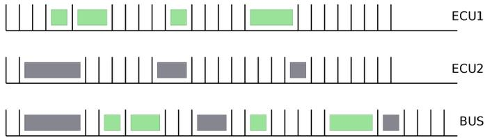
**Figure 2.12:** Two nodes sending data to a bus using minislotted. The size of the slots is adjusted to fit the data being sent by one of the nodes. Slots in which no data is sent are not extended.
