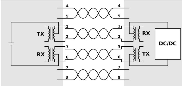
**Figure 3.10:** Phantom powering, also known as mode A, in which the voltage is fed over the same wires as the signals. Only two of the four cable pairs in a standard CAT5 or CAT6 cable are used. The PSE can be seen to the left and the PD to the right.
