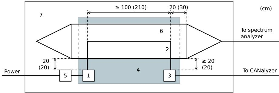
**Figure 5.2:** J1939 test setup with distances given by ISO 11452-5. Values within parentheses are the actual distances used during the tests.
