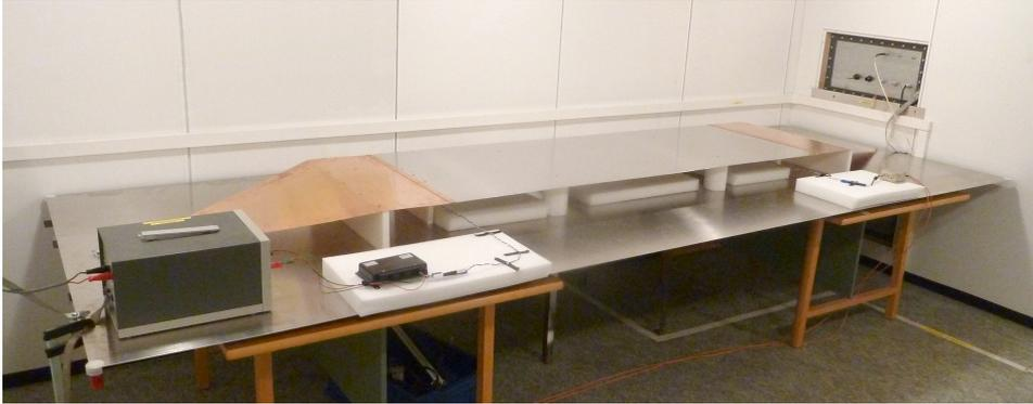
**Figure 5.3:** EMC chamber during J1939 test. The LISN can be seen standing on the ground plane to the left, the ECU on the insulating base to the left, the fiber optics receiver on the insulation to the right and the cable duct in the background to the right.
