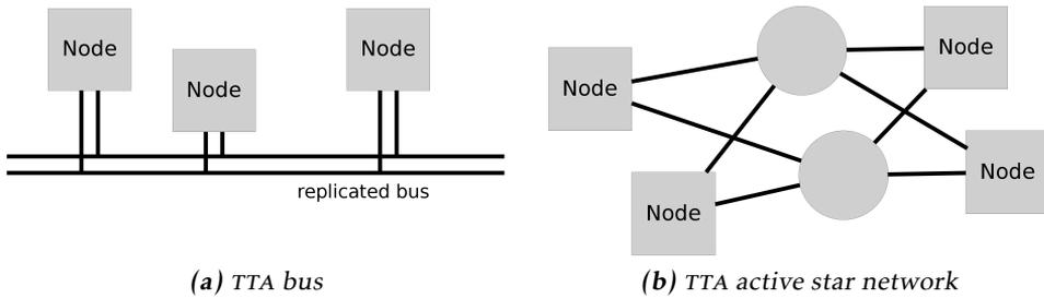
**Figure 3.8:** Example of TTA networks showing the two supported network topologies, the linear bus and the active star network.
