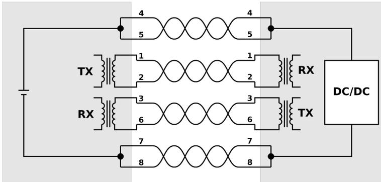
**Figure 3.11:** Spare-pair powering using the spare wires in a standard CAT5 or CAT6 cable. This is also known as power over Ethernet mode B. The PSE can be seen to the left and the PD to the right.
