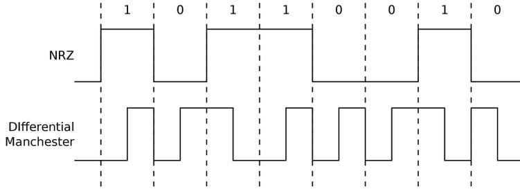
**Figure 3.13:** Differential Manchester encoding compared to non-return-to-zero encoding. Every bit is represented by a signal level change.
