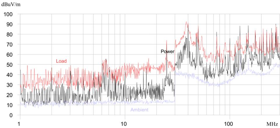
**Figure 5.11:** Emission spectrum from FlexRay EVB, 1-300 MHz. The step is due to the change in resolution bandwidth. Note the increase in emission levels over the whole spectrum after power feeding the evaluation boards.
