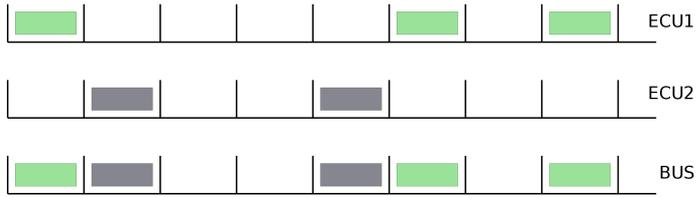
**Figure 2.10:** Example of a TDMA network. The nodes are assigned slots in which no other node can transmit to the network. This is illustrated by messages sent by two nodes and the resulting traffic on the network.
