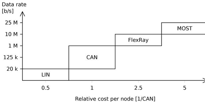
**Figure 2.9:** Trade off between cost and bandwidth for LIN, CAN, FlexRay and MOST. Interfaces supporting a higher bandwidth generally cost more. The cost in the figure is set in relation to the cost of CAN for comparative reasons.
