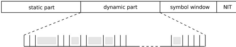
**Figure 3.6:** The dynamic part of a FlexRay cycle utilizes minislotted a network access model. Slots in which data is sent are extended to fit the data, otherwise their size are kept to a minimum.
