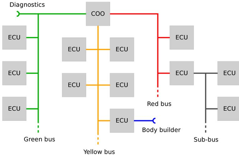
**Figure 2.15:** Layout of the J1939 bus network in Scania's vehicles. The buses (red, yellow and green) roughly corresponds to the functional domains defined in automotive applications.
