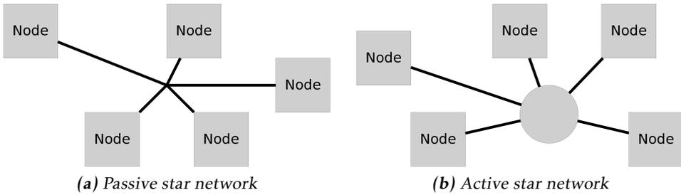
**Figure 2.4:** The passive star network to the left connects the nodes together in one single point. No amplification or routing is performed here. This can however be done in the star network to the right because of the centrally positioned active star node.
