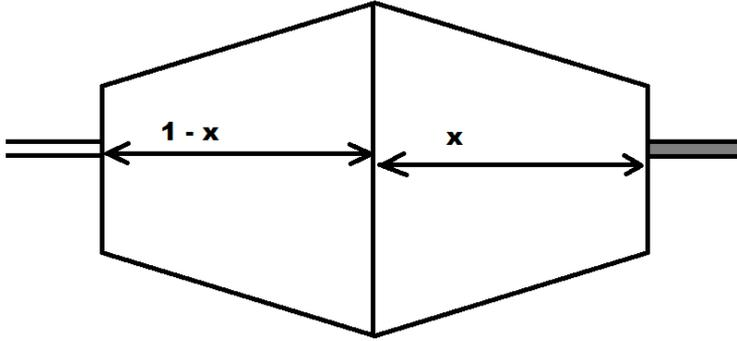
**Figure 2.7.** A heat exchanger containing working fluid. The working fluid enters the heat exchanger in liquid state and leaves as gas. The variable  $x$  indicates how much of the working fluid that has changed state from liquid to gas. One of the biggest challenges with the modeling is to handle the differences in temperature and pressure caused by different values of  $x$ .
