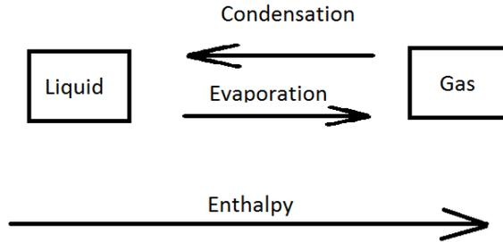
**Figure 2.6.** Liquid, gas and the two phase state that exist during evaporation and condensation are states the working fluid appears in during the heat exchange. The state of the working fluid depends on enthalpy. Increasing enthalpy leads to evaporation if the fluid is a liquid.
