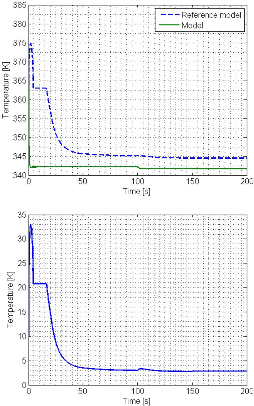
**Figure 2.21.** Temperature of the working fluid after the condenser is seen in the upper figure. The working fluid enters the condenser as gas and leaves as liquid. There is a step in mass flow for the cooling refrigerant at time  $t = 100$ s. The working fluid mass flow is constant. Difference in temperature of the working fluid is seen in the lower figure. The difference is at its largest at the first 50 seconds, and then decreases to about 1 percent
