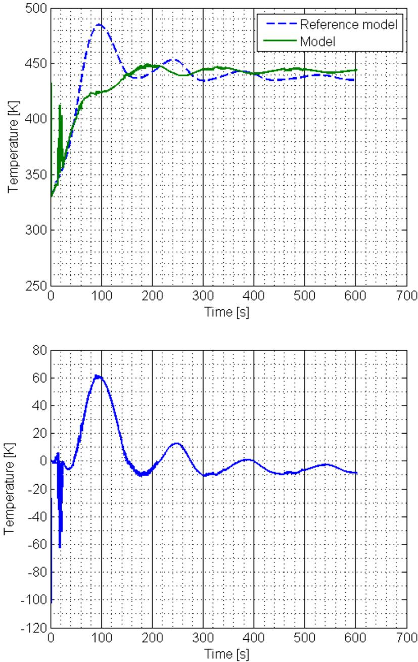
**Figure 3.3.** Temperature after last heat exchanger is seen in the upper figure and the difference between the in the lower figure. The working fluid in both models are completely evaporated. The simulation is made during start of the system and when the system is stationary operating after the start. The working fluid is completely condensed for both models. The behavior of the models agree but with a time difference and a difference in temperature of about 2.5 percent.
