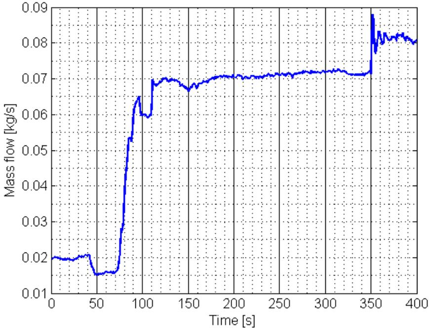
**Figure 2.14.** Measured input hot gas mass flow to the heat exchanger in Figure 2.13. There is a step in mass flow between time  $t = 75$ s and time  $t = 100$  s.
