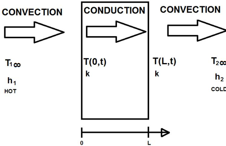
**Figure 2.5.** Heat transfer between a gas with high temperature and the working fluid through walls of the heat exchanger. This is the heat transfer that occurs in Figure 2.4. Forced convection from the hot gas to the metal plate heats up the metal plate. Conduction in the metal plate transfers heat from the hot side of the metal plate to its other side. Forced convection from the metal plate to the working fluid heats up the working fluid.
