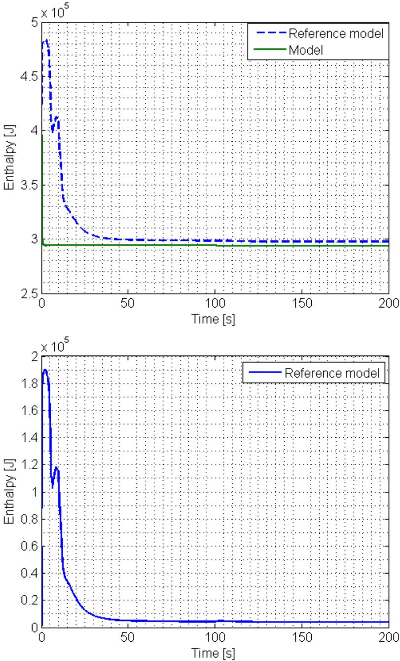
**Figure 2.20.** Enthalpy of the working fluid after the condenser is seen in the upper figure. The working fluid enters the condenser as gas and leaves as liquid. There is a step in mass flow for the cooling refrigerant at time  $t = 100$ s. The working fluid mass flow is constant. The difference, seen in the lower figure, is at its largest at the first 50 seconds, and then decreases to about 3 percent.
