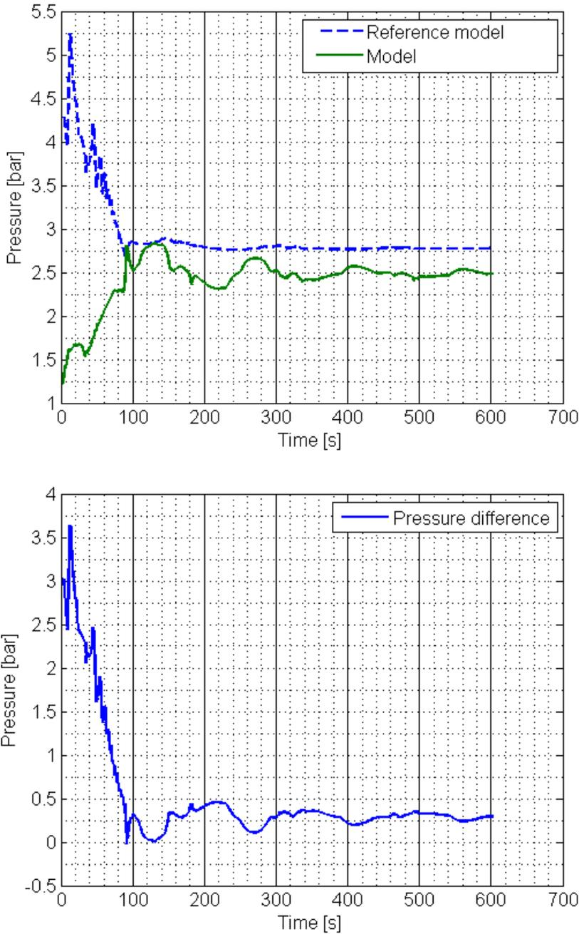
**Figure 3.5.** Pressure in working fluid after the turbine expander is seen in the upper figure and the difference between them in the lower figure. The simulation is made during start of the system and when the system is stationary operating after the start. The behavior of the working fluid in the reference model is seen in the developed model, but with a larger amplitude.
