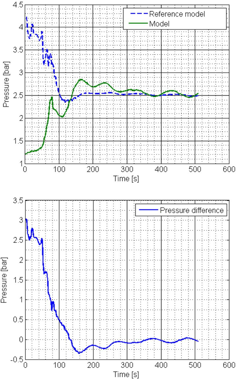
**Figure 2.17.** Pressure after the turbine is seen in the upper figure and the difference between the models in the lower figure. The working fluid entering both models has the same properties. In the turbine expander, the volumetric flow changes that causes a change in pressure. The comparison is made during start of the system and when the system is stationary operating after the start.
