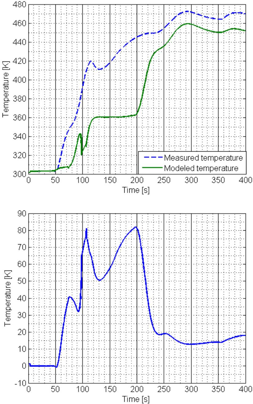
**Figure 2.13.** Output temperature from a heat exchanger is shown in the upper figure. The input working fluid is liquid during the first second and then gas. There is a step in mass flow between time  $t = 75$  s and time  $t = 100$  s. The developed model is compared to measurement data from cell. The difference can be seen in the lower figure.
