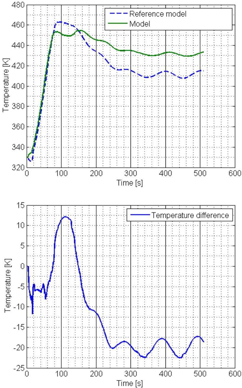
**Figure 2.18.** Temperature after the turbine is seen in the upper figure, and the difference between the models in the lower figure. The working fluid entering both models has the same properties. In the turbine expander, the volumetric flow changes that causes a change in pressure. The comparison is made during start of the system and when the system is stationary operating after the start.
