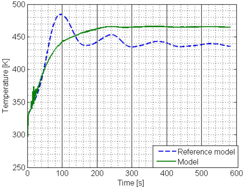
**Figure 3.1.** Temperature after the last heat exchanger. The simulation is made during start of the system and when the system is stabilized after the start. The working fluid is completely evaporated for both models. There is a difference in the model which might be explained by the mass flow modeling. A comparison with the same mass flow as the reference model can be seen in Figure 3.3.
