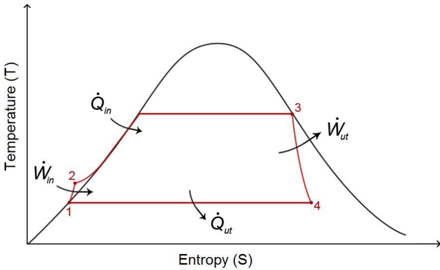
**Figure 1.2.** Entropy versus temperature diagram for the Rankine cycle. The curve shows the relationship between temperature and entropy. The Rankine cycle converts heat into work. The figure also shows where work and heat are put in and taken out. The picture is downloaded from Wikipedia 2012-05-06.
