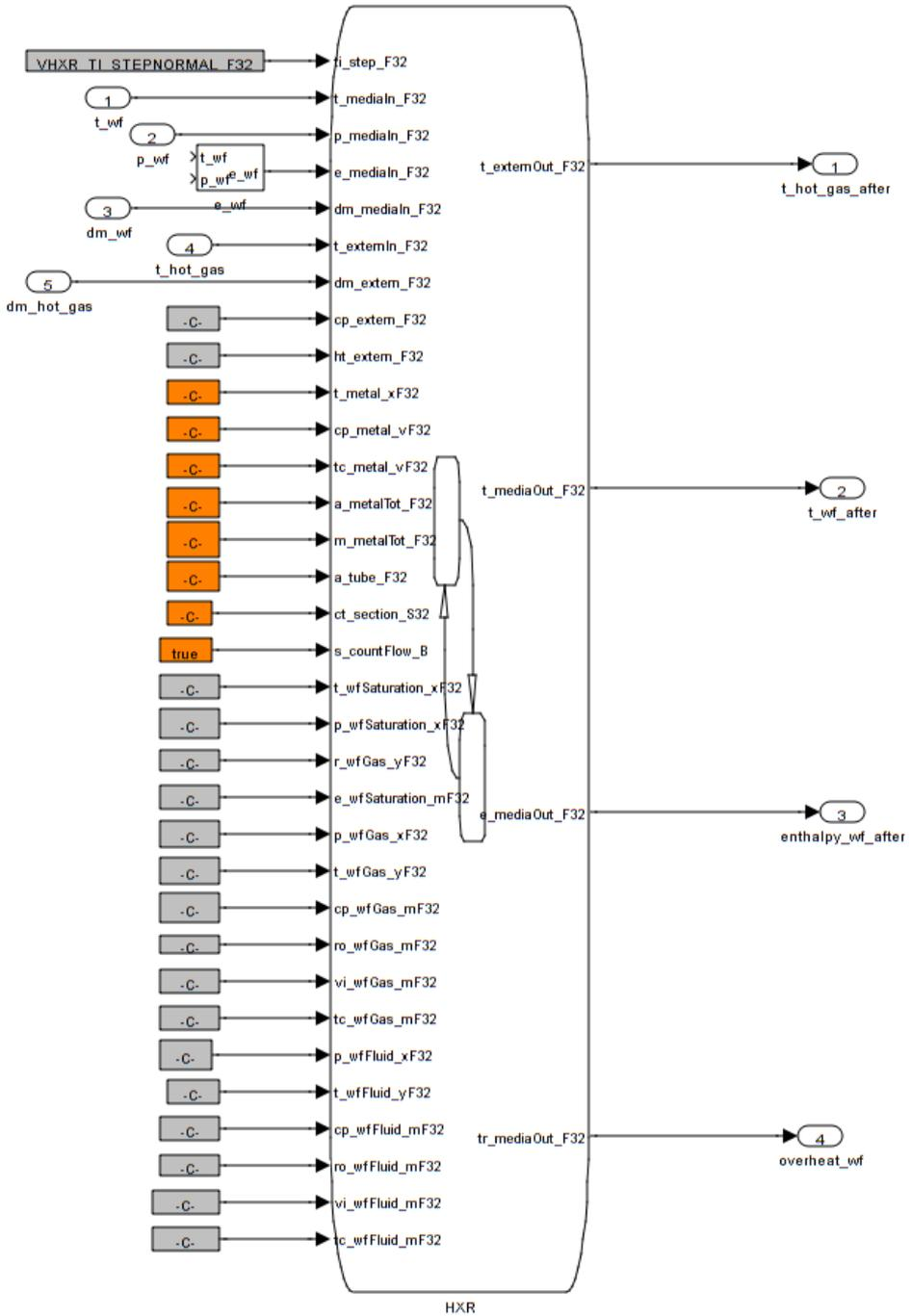
**Figure 2.16.** The heat exchanger model. Input variables are the temperature, pressure, mass flow and enthalpy of the working fluid and the temperature and mass flow of the hot gas. Output variables are the temperature, enthalpy and degrees of overheating of the working fluid and the temperature of the hot gas.
