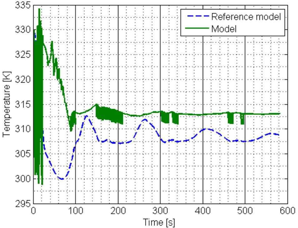
**Figure 3.2.** Temperature after condenser. The simulation is made during start of the system and when the system is stabilized after the start. The working fluid is completely condensed for both models. There is a difference in the model which might be explained by the mass flow modeling. A comparison with the same mass flow as the reference model can be seen in Figure 3.4
