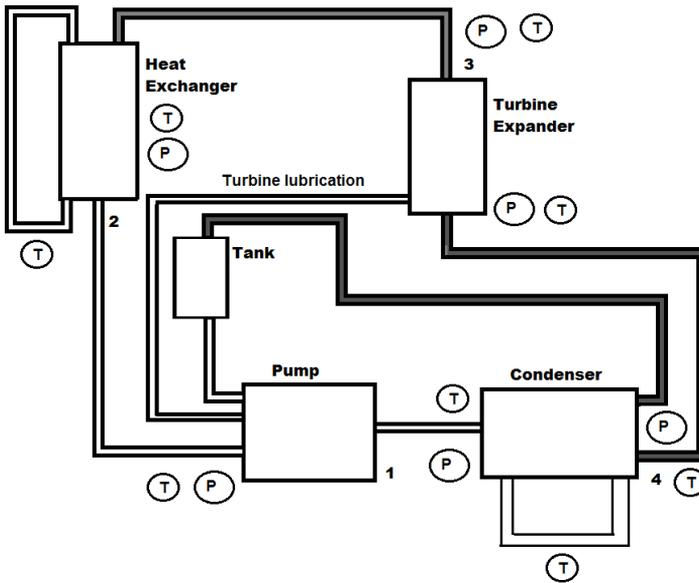
**Figure 1.3.** A schematic of the system installed in the engine test cell. The temperature sensors and pressure sensors used for validation are marked with  $T$  and  $P$ . The three heat exchangers are schematically shown as one and the same is for the condenser and subcooler.
