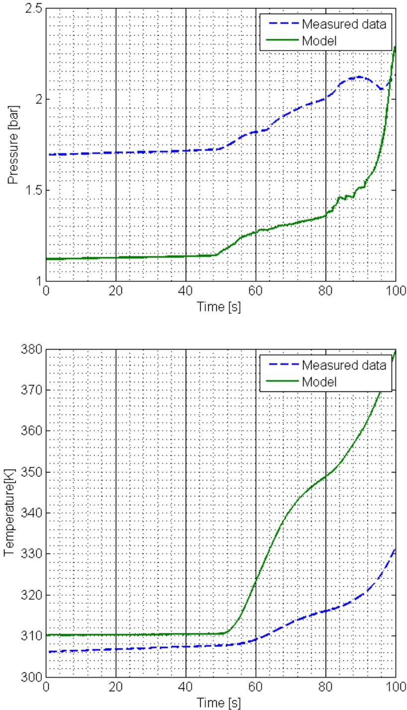
**Figure 2.19.** Pressure difference between measurement data and the developed model after the turbine is seen in the upper figure and temperature difference in the lower. The working fluid entering both models has the same properties. In the turbine expander, the volumetric flow changes that causes a change in pressure. The comparison is made during start of the system and when the system is stationary operating after the start.
