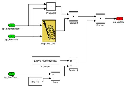
Figure 2.5: Simulink scheme of sub-model Pressure to AirFlow, corresponding to Equation (2.8). Uses the density of the inlet air, the swept volume and a efficiency map to estimate air mass flow in to the cylinder.
