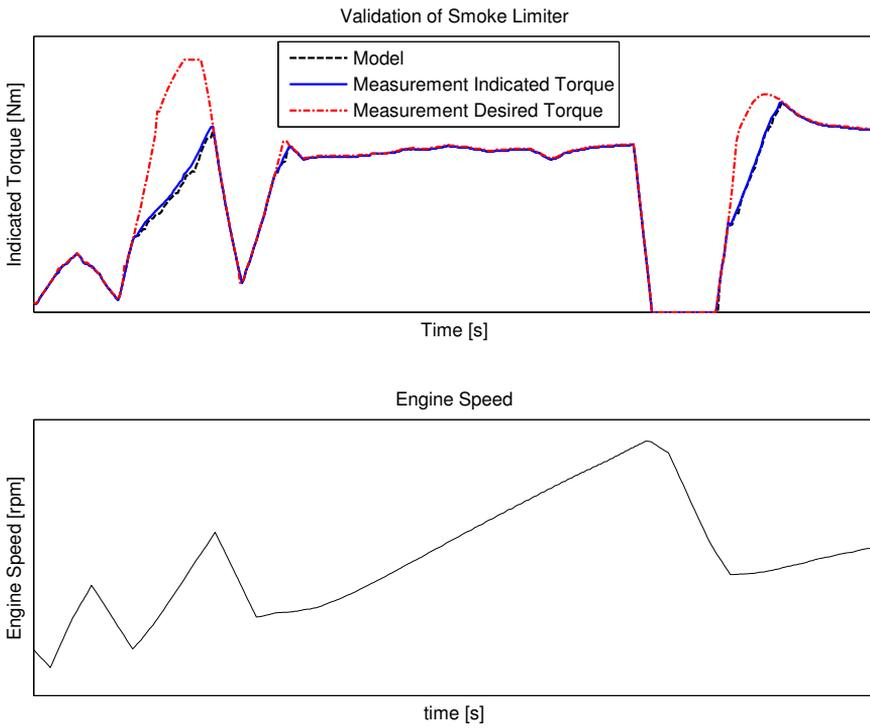
Figure 2.9: Comparison between measured and modelled indicated torque. Desired torque is what the driver demands with the pedal. In heavy load transients the desired torque is limited to keep the soot production down.
