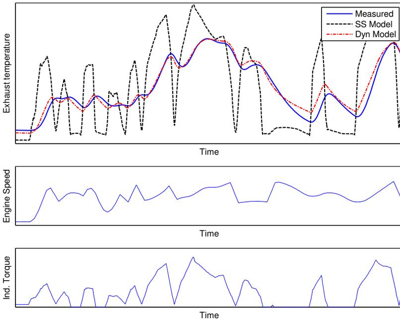
Figure 2.19: Simulated compared to measured exhaust temperature
