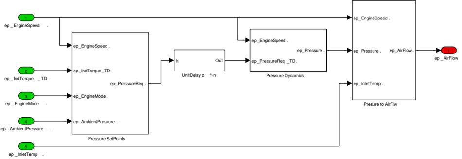
Figure 2.3: Simulink scheme of the sub-model Air Dynamics. Consists of three sub-models, inlet pressure set-point, inlet pressure dynamics and air mass flow.
