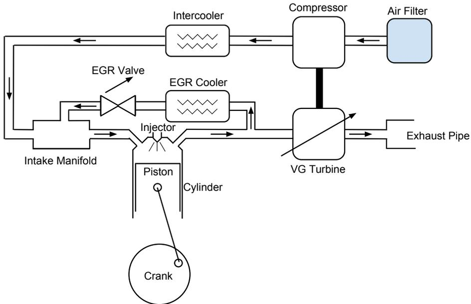
Figure 1.1: Schematic view of a diesel engine
