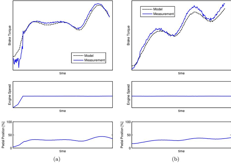
Figure 3.1: Brake torque transients in the BLB-cycle where the smoke limiter is active during the transients
