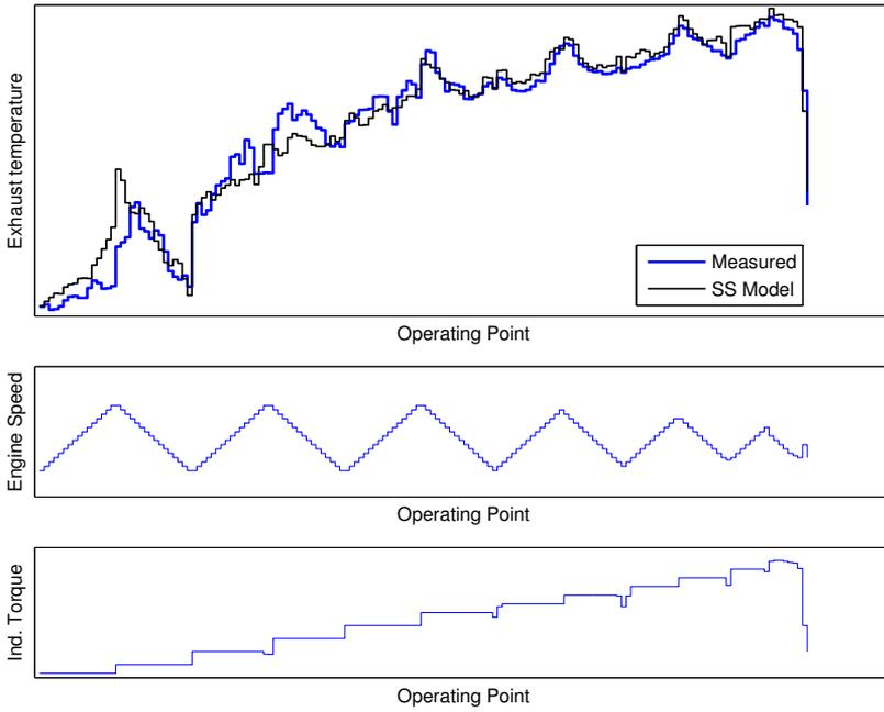
Figure 2.20: Simulated compared to measured steady state exhaust temperature.
