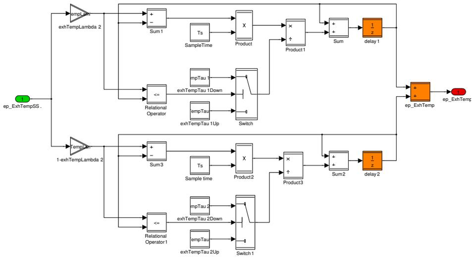
Figure 2.18: Simulink scheme of the dynamic exhaust temperature, implementation of Equation (2.15)-(2.17). A sum of two first order systems that filters the steady state exhaust temperature from the Simulink scheme in Figure 2.16.
