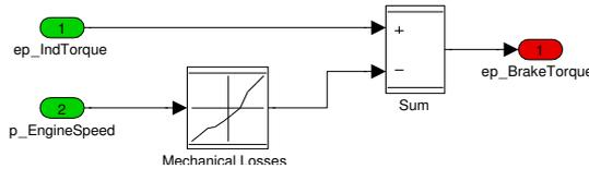
Figure 2.14: Simulink scheme of sub-model Brake Torque, corresponds to Equation (2.12). Subtracts losses from indicated torque and returns brake torque.
