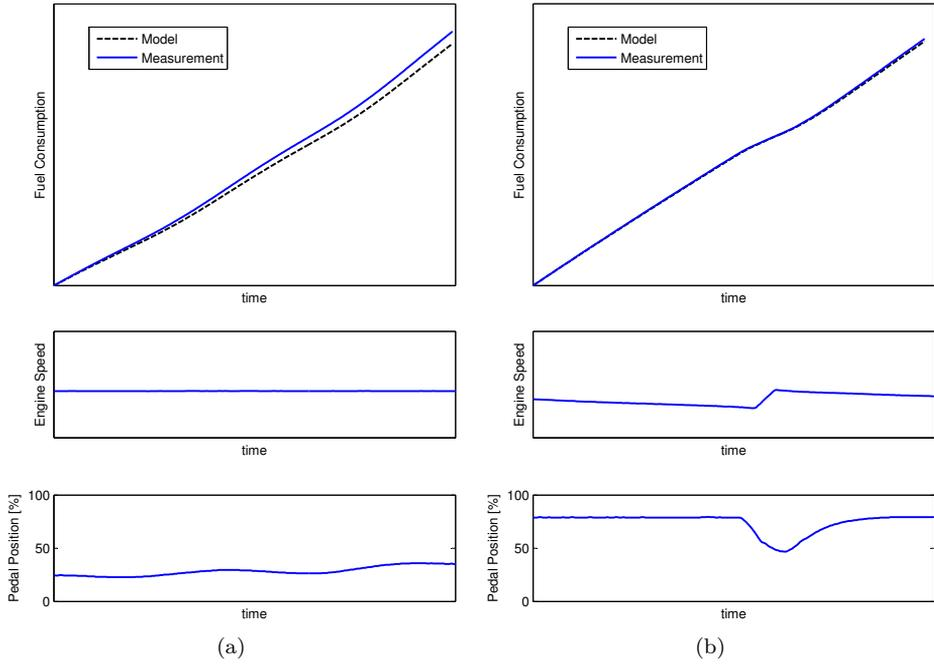
Figure 3.4: Fuel consumption in two sections of the BLB-cycle
