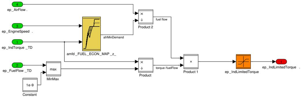
Figure 2.8: Simulink scheme of SmokeLimiter. Limits the desired torque, considering the current air-flow, so the engine doesn't produce as much soot in the exhausts.
