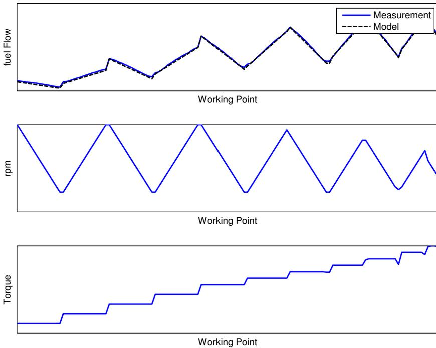
Figure 2.12: Comparison between measured and modelled fuel flow at steady state operation. The model is more accurate at higher torque where the engine works at accelerations.
