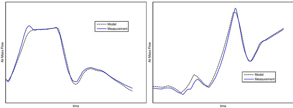
Figure 2.7: Comparison between measured and modelled air mass flow in two different time intervals. The MARE is 3.2%.
