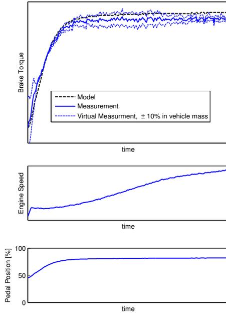
Figure 3.3: Shows how  $\pm 10\%$  in mass affects the brake torque with given acceleration.
