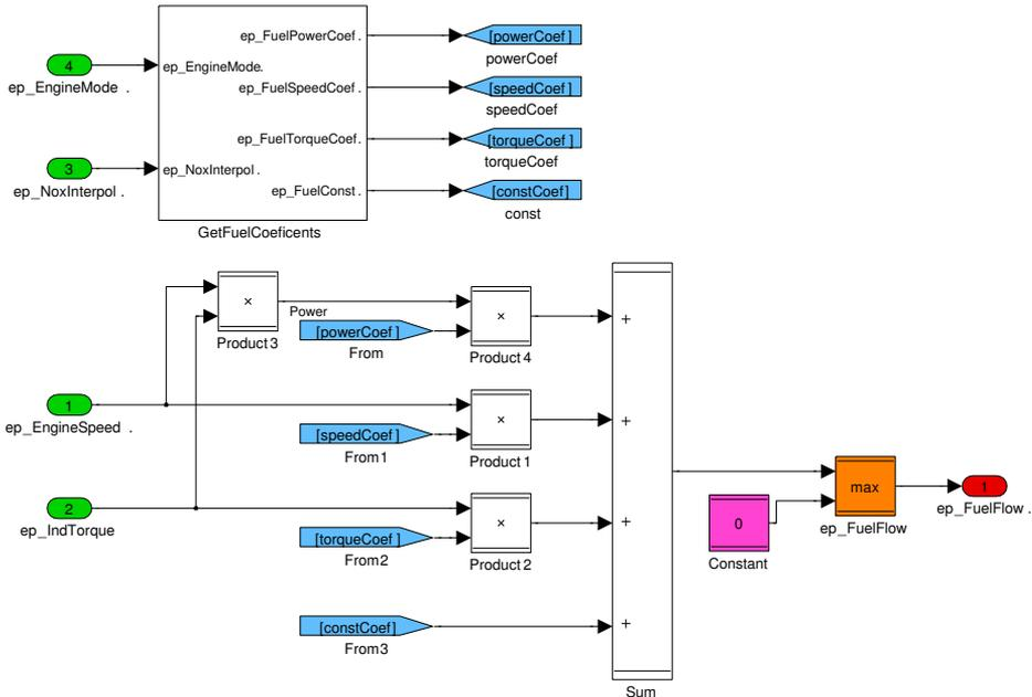
Figure 2.10: Simulink scheme of FuelFlow, The fuel flow is modelled as a linear function of indicated power, indicated torque and engine speed, equation (2.10).
