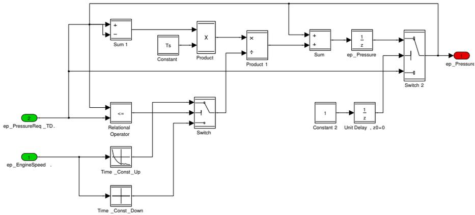
Figure 2.4: Simulink scheme of sub-model Pressure Dynamics, a first order system with varying time constant, corresponding to Equation (2.7).
