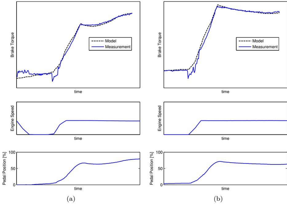
Figure 3.2: Brake torque transients in the BLB-cycle where the smoke limiter is active during the transients
