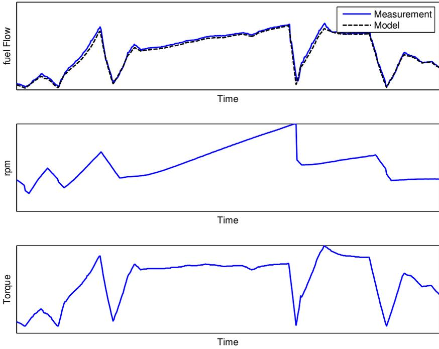
Figure 2.13: Comparison between measured and modelled fuel flow at transient operation, in a part of the WHTC.
