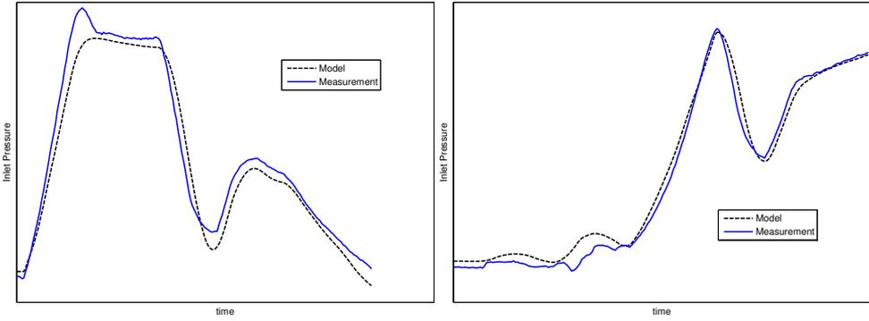
Figure 2.6: Comparison between measured and modelled inlet pressure in two different time intervals. The MARE is 3.5%.
