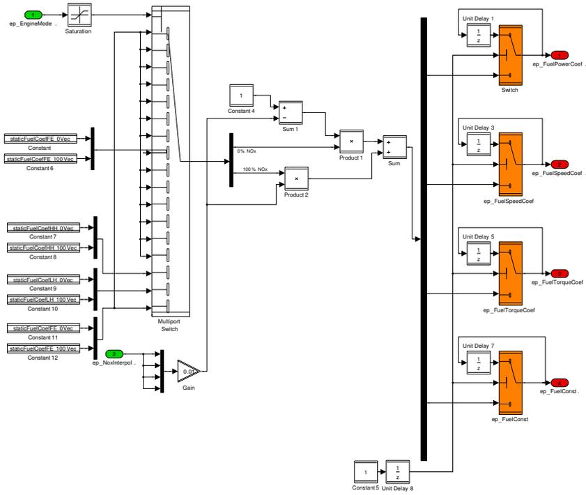
Figure 2.11: Simulink scheme of the sub-model GetFuelCoefficients in Figure 2.10. Initializes the model coefficients depending on  $NO_x$  production and engine mode.
