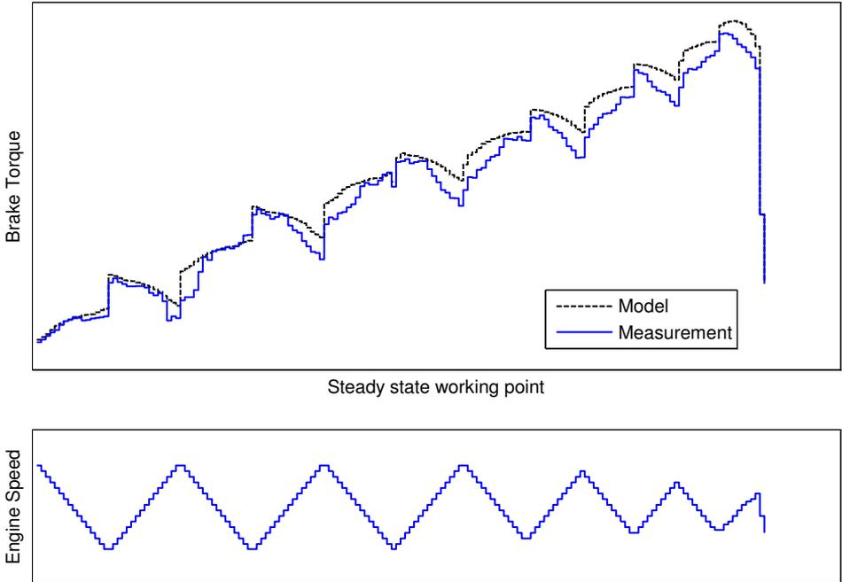
Figure 2.15: Modelled and measured brake torque
