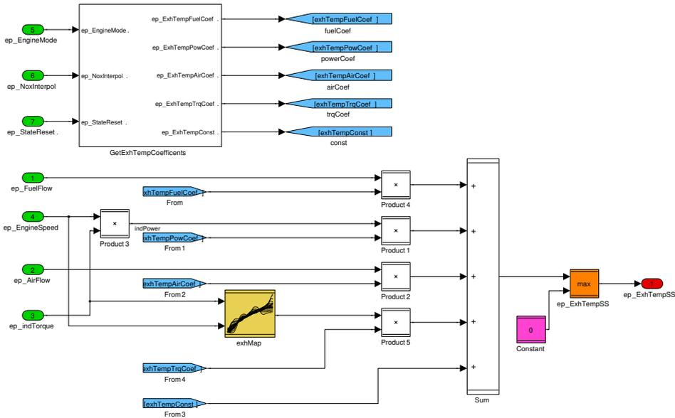
Figure 2.16: Simulink scheme of the steady state exhaust temperature, implementation of Equation (2.14). The output is input to the Simulink scheme in Figure 2.18.
