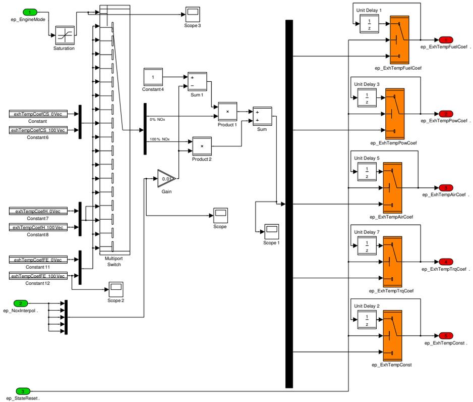
Figure 2.17: Simulink scheme of the block GetExhTempCoefficients in Figure 2.16. Initializes the model coefficients depending on  $NO_x$  production and engine mode.
