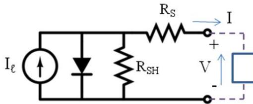
**Figure 2.1:** Circuit diagram of the PV single diode.
