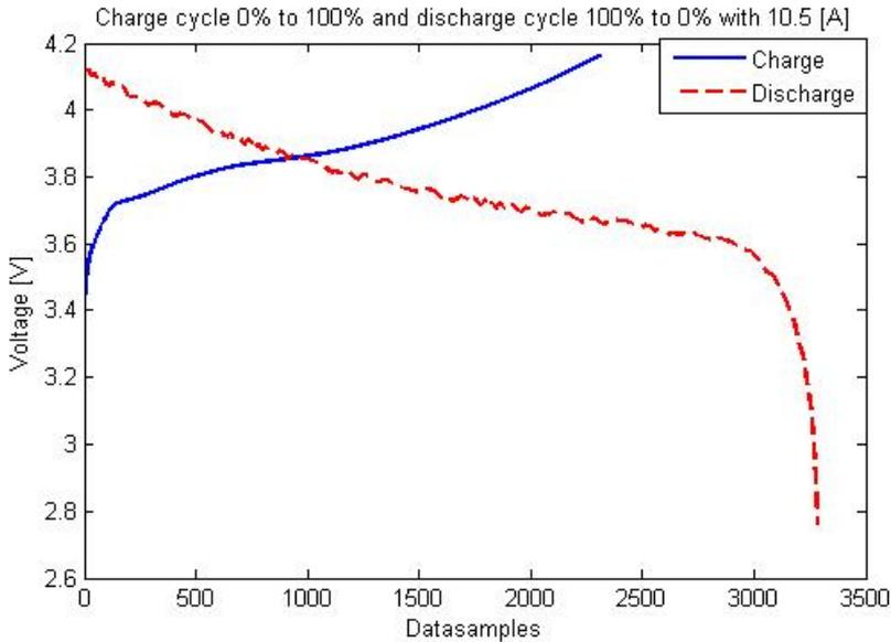
**Figure 2.3:** Charge and discharge cycle of one cell battery with current 10.5 [A].
