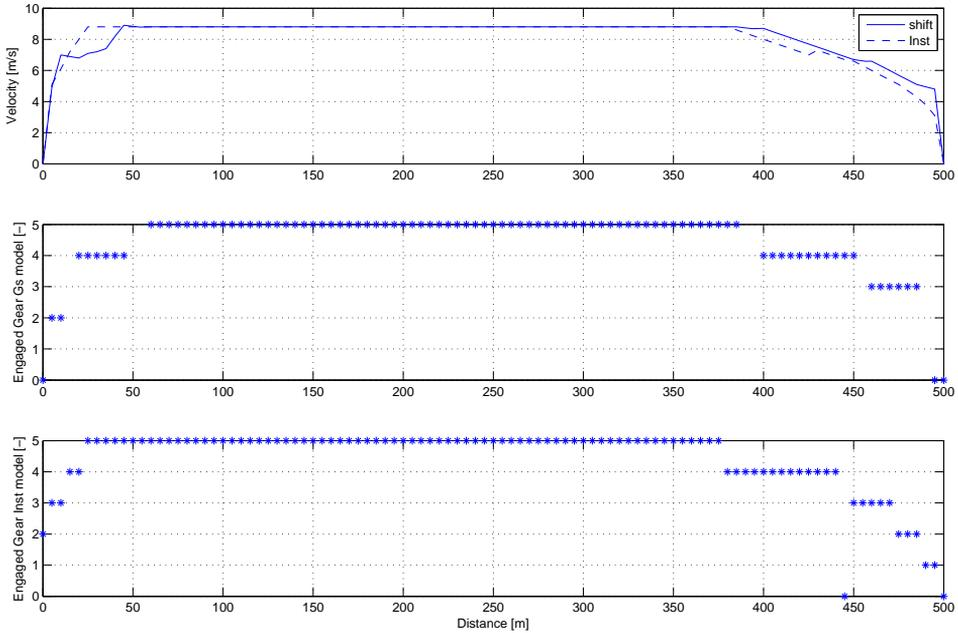
**Figure 5.4.** Optimal speed profiles and gear selection comparison between the gearshift model and the instantaneously model for 500m. The map based engine model is used.
