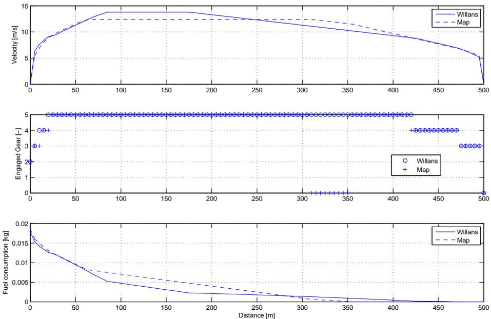
**Figure 5.9.** Optimal speed profiles and gear selection comparison between the Willans engine model and the map based engine model. Results for 500m with a time constraint of 50s and using the instantaneously gear shift model.
