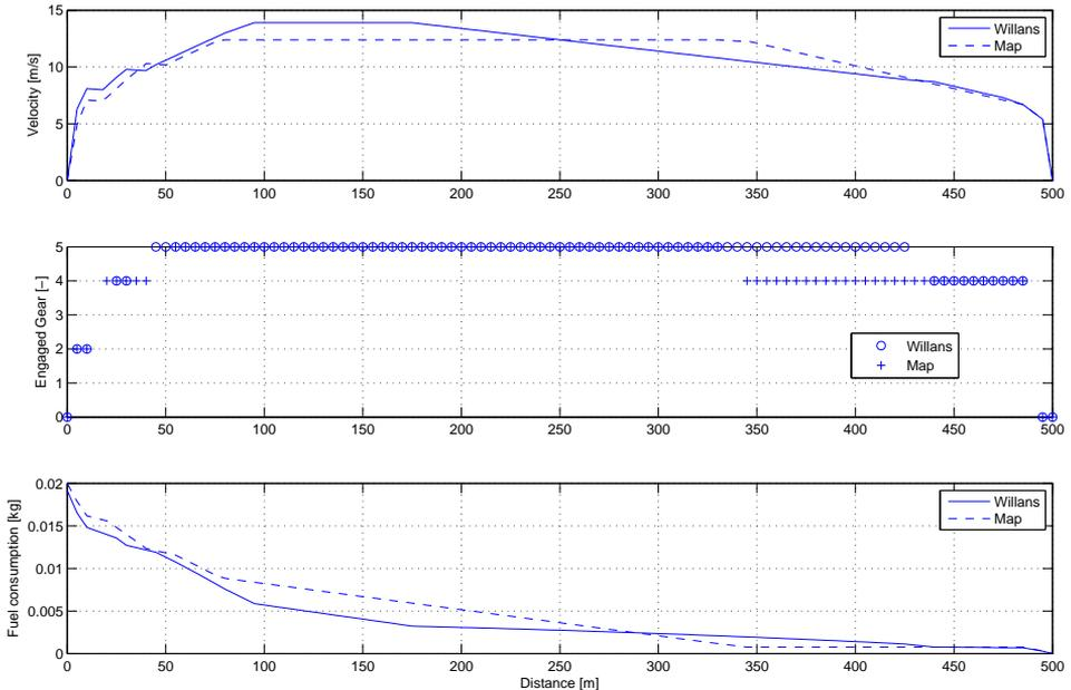
**Figure 5.10.** Optimal speed profiles and gear selection comparison between the Willans engine model and the map based engine model. Results for 500m with a time constraint of 50s and using the gear shift model.
