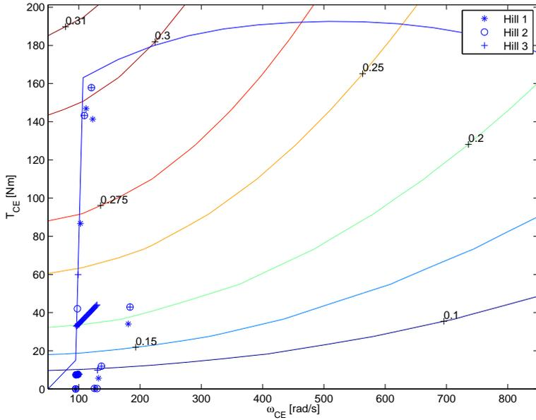
Figure 5.21. Engine operating points for every hill height.
