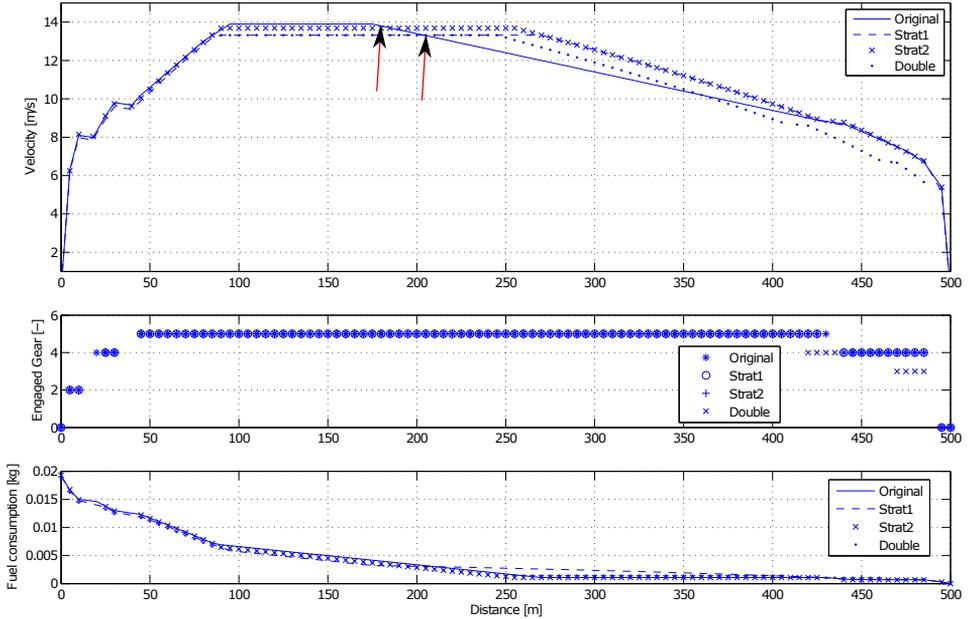
**Figure 5.15.** Optimal profiles comparison between the original solution, the solutions with both coasting strategies, and the solution of merging the speed grids for both strategies. The gear shift model with Willans approximation is used.
