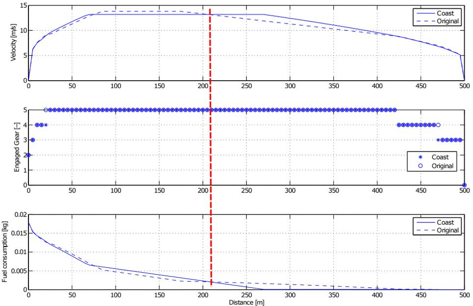
**Figure 5.14.** Optimal profiles comparison between the original solution and the solution with the coasting strategy one for the instantaneously gear shift model. Willans engine model.
