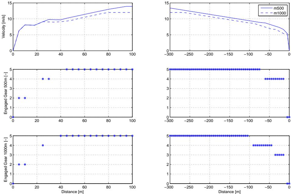
**Figure 5.12.** Optimal speed profiles and gear selection in the acceleration and deceleration phases, comparison between 500m trip in 50s and 1000m trip in 100s i.e. the same average speed. Willans engine model is used.
