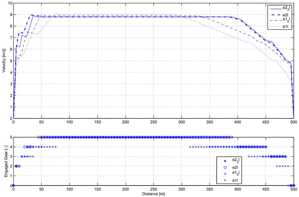
**Figure 5.24.** Optimal speed profiles and gear selection for several engine sizes. Willans engine model.
