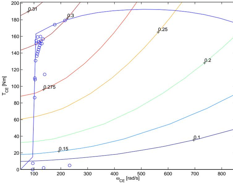
Figure 5.17. Engine operating points for the acceleration phase with the dense grid.
