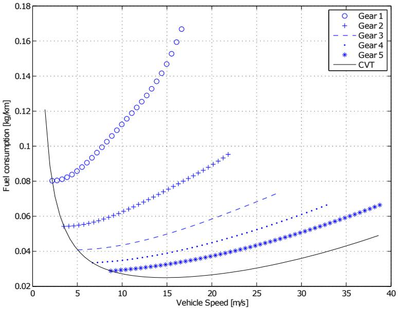
Figure 5.2. Fuel consumption for constant vehicle speed and different gears. The map based engine model is used.
