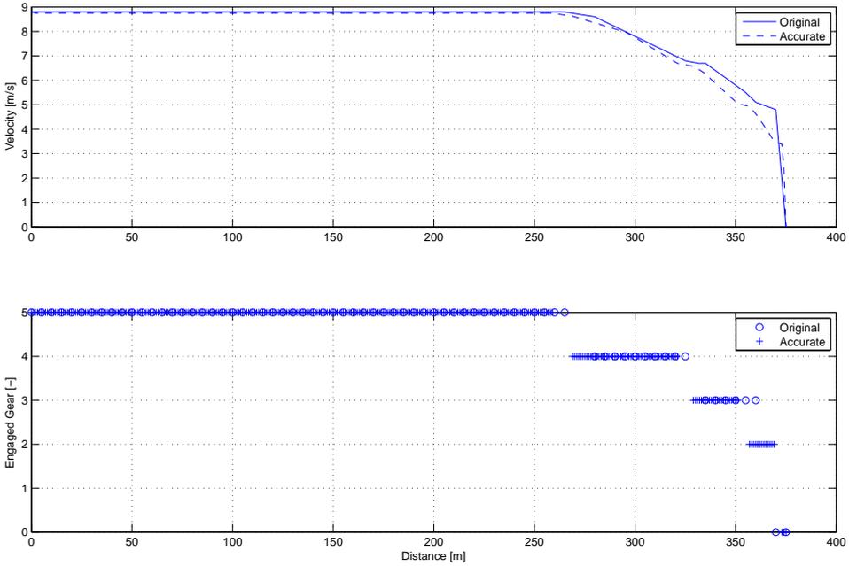
Figure 5.18. Comparison of the optimal deceleration profiles between the original solution and the solution obtained with the dense grid.
