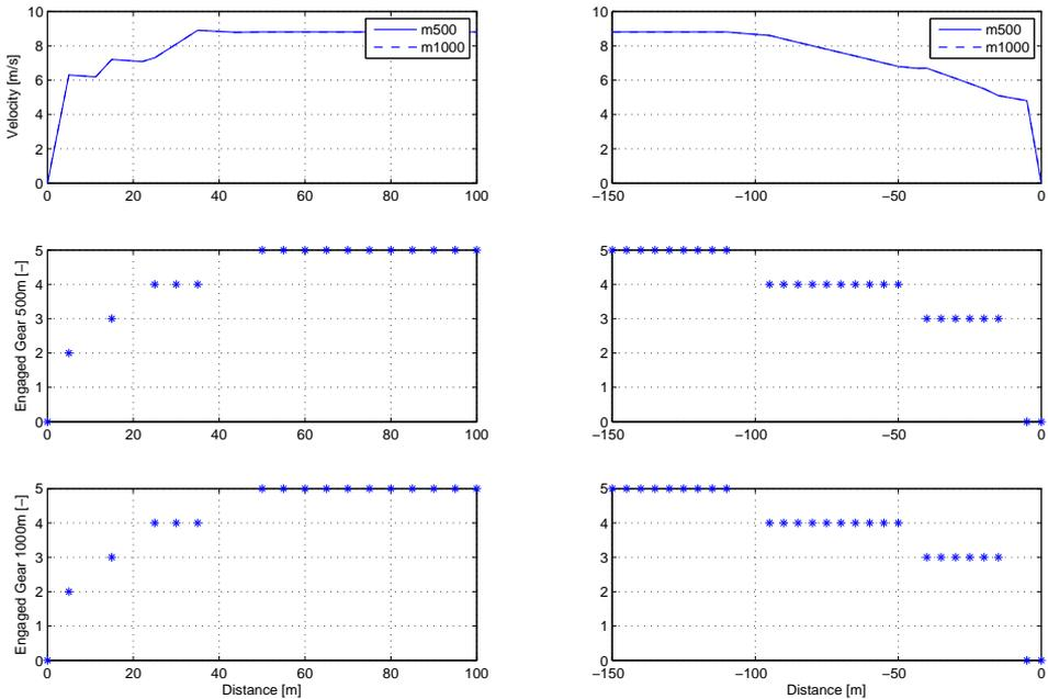
**Figure 5.11.** Optimal speed profiles and gear selection in the acceleration and deceleration phases, comparison between 500m trip and 1000m trip. Results using the Willans engine model.
