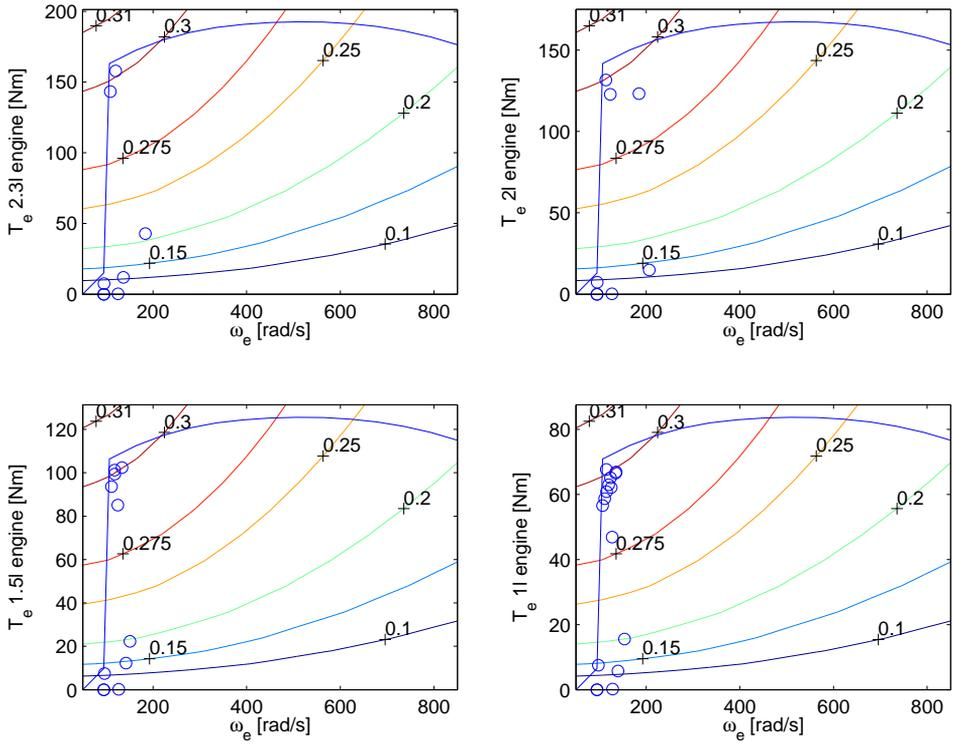
Figure 5.25. Engine operating points for several engine sizes. Willans engine model.
