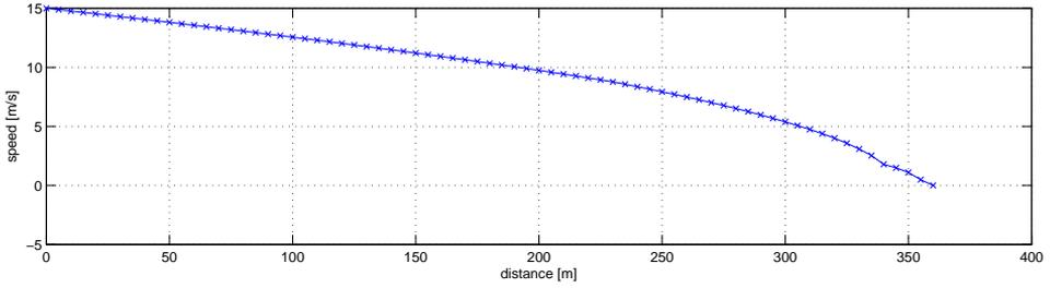
**Figure 5.13.** Coasting profile with  $15\text{m/s}$  as initial speed. The change in the curve is because the engine is disengaged at low speeds.
