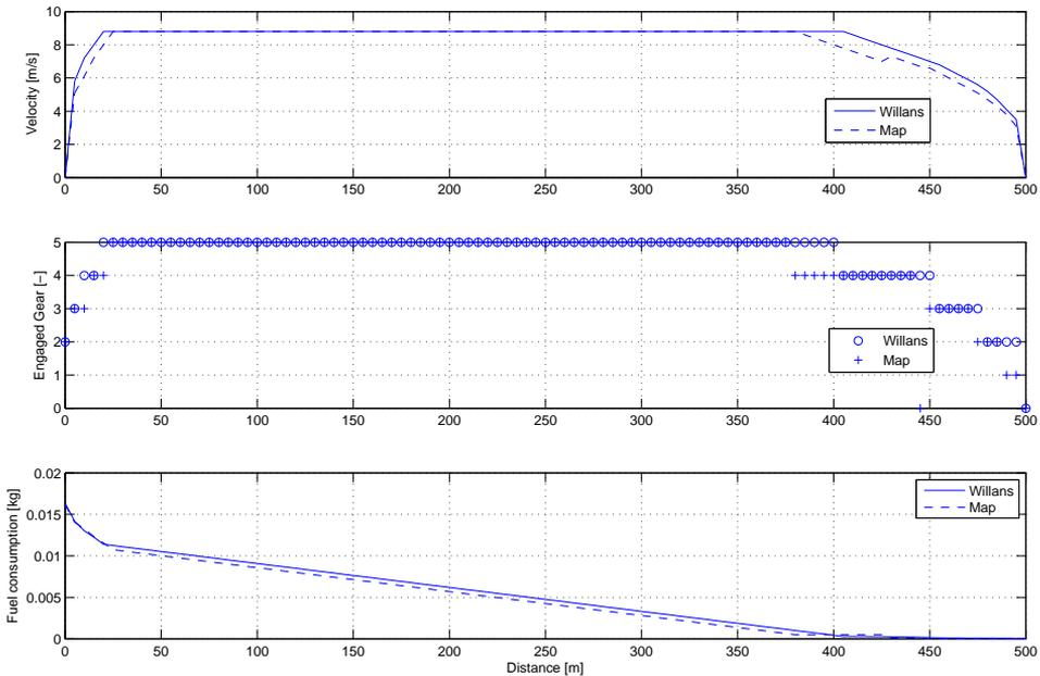
**Figure 5.7.** Optimal speed profiles and gear selection between the Willans engine model and the map based engine model are compared. Results for 500m without time constraint and using the instantaneously gear shift model.
