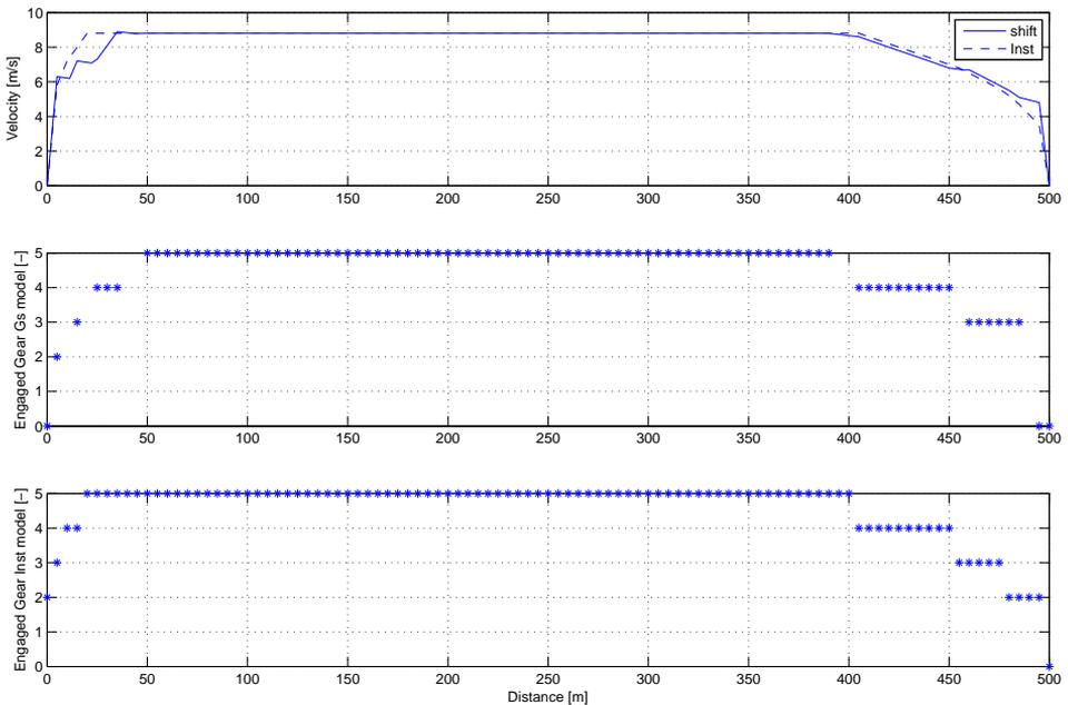
**Figure 5.3.** Optimal speed profiles and gear selection comparison between the gearshift model and the instantaneously model for 500m. Willans engine model is used.
