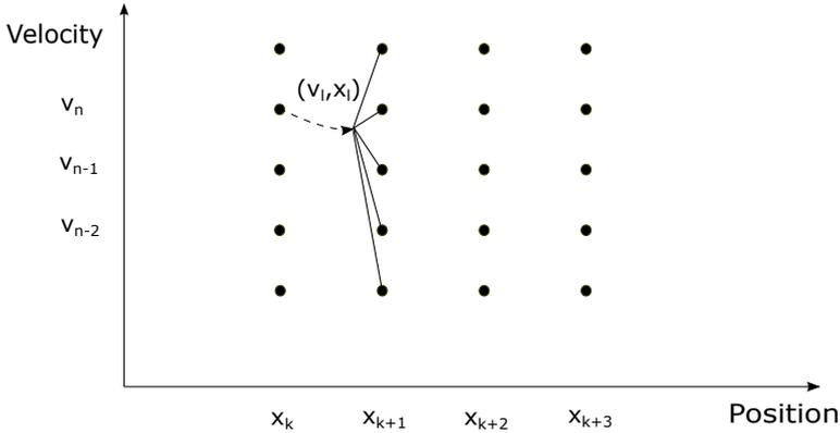
**Figure 4.1.** Computation of the cost to go from  $v_n, x_k$  to the states in  $x_{k+1}$  with a gear shift maneuver.
