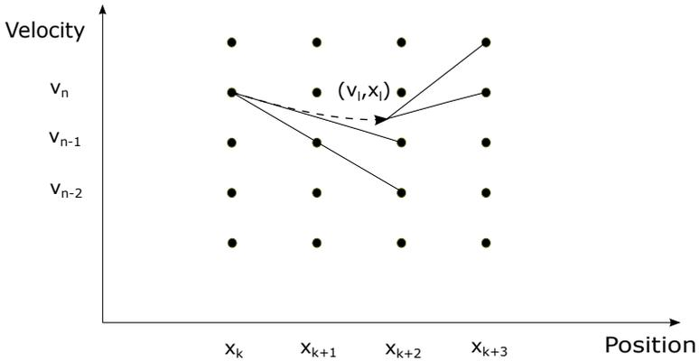
**Figure 4.2.** Skipping grid points strategy from  $(v_n, x_k)$  during a gear shift maneuver. In the figure,  $(v_l, x_l)$  is the point where the gear shift maneuver ends.
