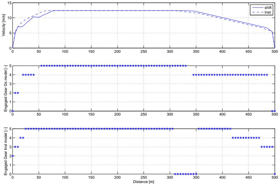
**Figure 5.6.** Optimal speed profiles and gear selection comparison between the gearshift model and the instantaneously model. Results for 500m, a time constraint of 50s, and using a map based engine mode.l
