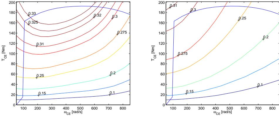
**Figure 2.2.** Efficiency maps and maximum torque curves for the map based model (left) and the Willans engine model (right).
