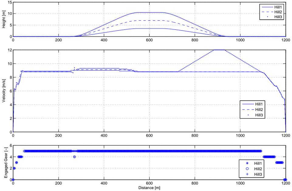
**Figure 5.20.** Comparison between three different hill heights with the gearshift model without time constraints. The Willans based engine is used.
