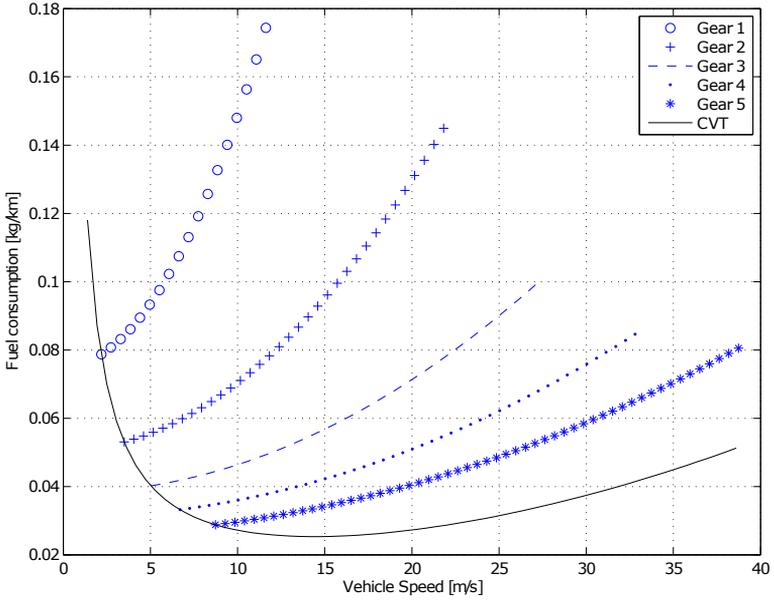
Figure 5.1. Fuel consumption for constant vehicle speed and different gears. Willans engine model is used.
