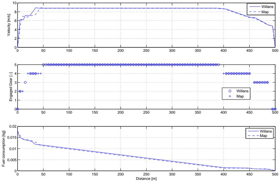
**Figure 5.8.** Optimal speed profiles and gear selection between the Willans engine model and the map based engine model are compared. Results for 500m without time constraint and using the gear shift model.
