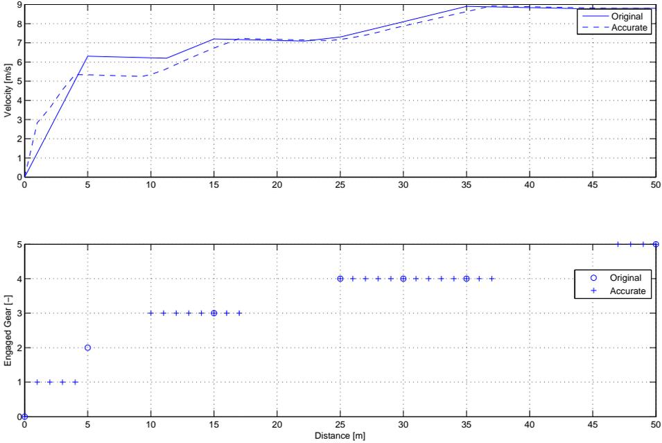
**Figure 5.16.** Comparison of the optimal acceleration profiles between the original solution and the solution obtained with the dense grid. The points where there is no gear is due to the gear shift maneuver, the gear used to compute the cost to go is the one which the maneuver has finished.
