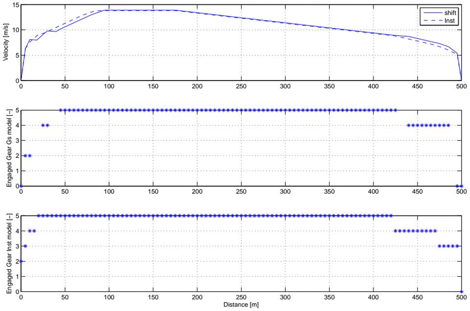
**Figure 5.5.** Optimal speed profiles and gear selection comparison between the gearshift model and the instantaneously model. Results for 500m, a time constraint of 50s, and using Willans engine model.
