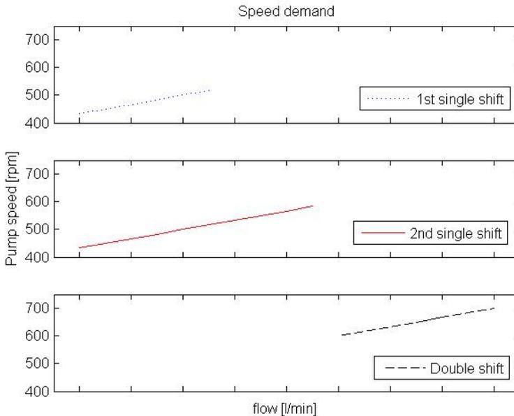
**Figure 4.7:** Speed demand for fixed displacement pump during shift
