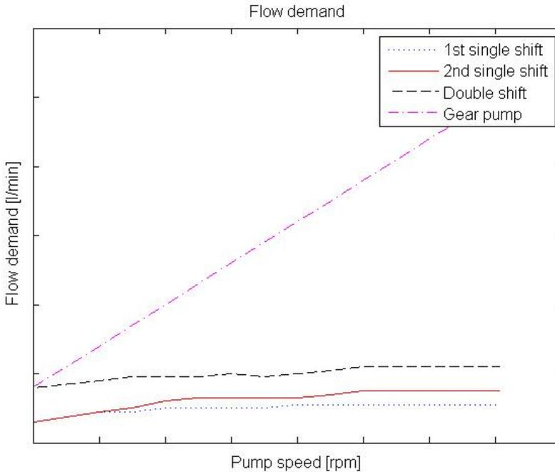
**Figure 4.4:** Demands of flow compared and flow from a gear pump with fixed displacement 0.06 l/rev
