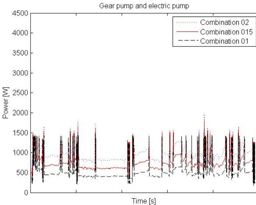
**Figure 6.5:** Power for combinations of gear pump and electric pump against time during the drive cycle
