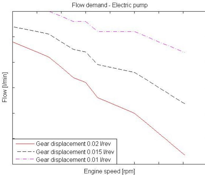
**Figure 4.9:** Flow demands on electric pump when the gear pumps have displacement of 0.02, 0.015 and 0.01 l/rev
