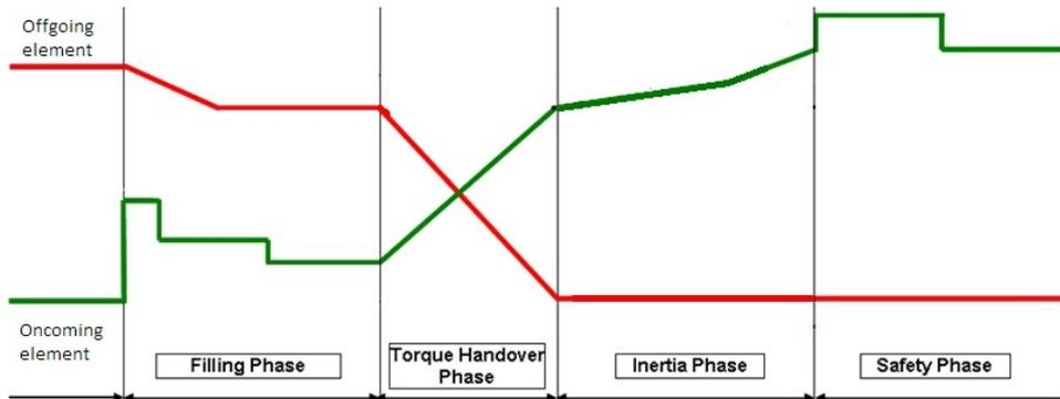
*Figure 2.5: Theoretical element shift that shows pressure for oncoming and offgoing element*
