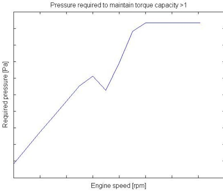
**Figure 3.1:** Example of required pressure against engine speed to maintain torque capacity > 1
