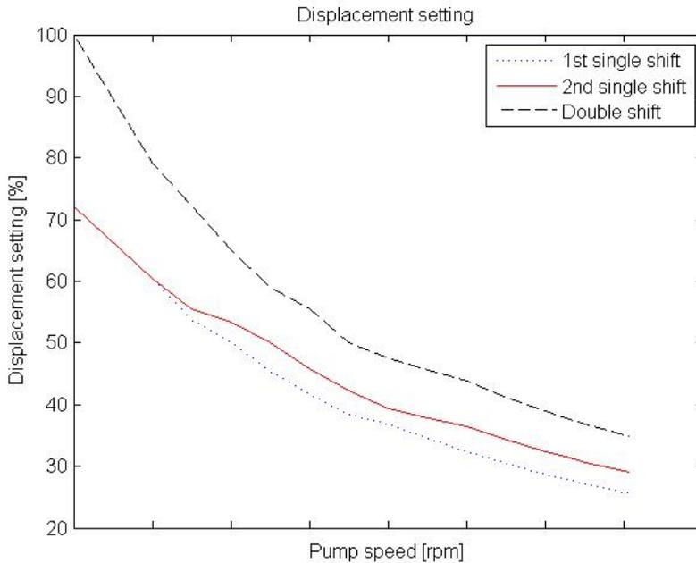
**Figure 4.6:** Displacement settings for variable displacement pump
