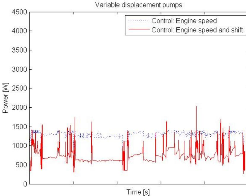
**Figure 6.3:** Power for variable displacement pumps against time during the drive cycle
