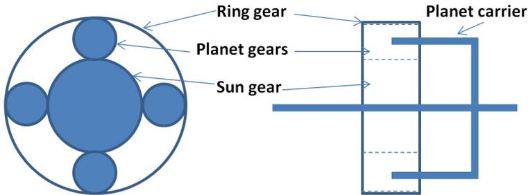
*Figure 2.1: Planetary gear set*
