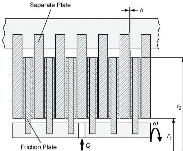
**Figure 2.3:** Schematic of a disengaged clutch
