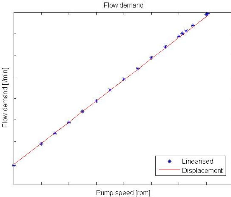
**Figure 4.3:** Demand of flow calculated either with linearisation or with displacement
