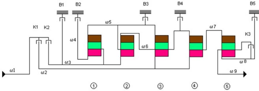
**Figure 2.2:** Powerflow for the transmission. Show which parts of each gear set that can be held stationary as well as which are input and output of the sun gear (red), the planet carrier (green) and the ring gear (brown). The brakes, B, clutches, K, and the speed,  $\omega$ , between the gear sets are shown.
