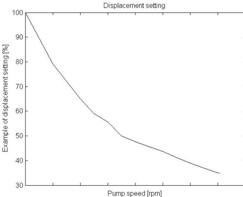
**Figure 5.1:** Example of displacement setting for a variable displacement vane pump
