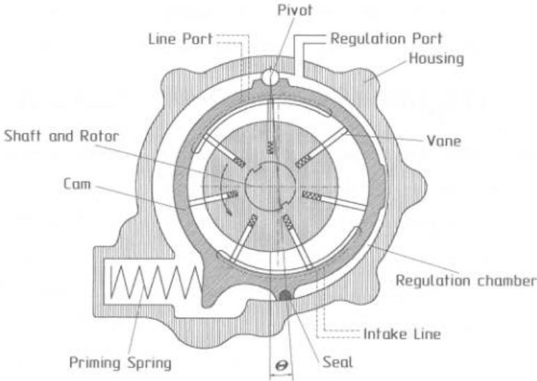
**Figure 4.5:** Example of variable displacement vane pump [Andriychuk et al., 2011]
