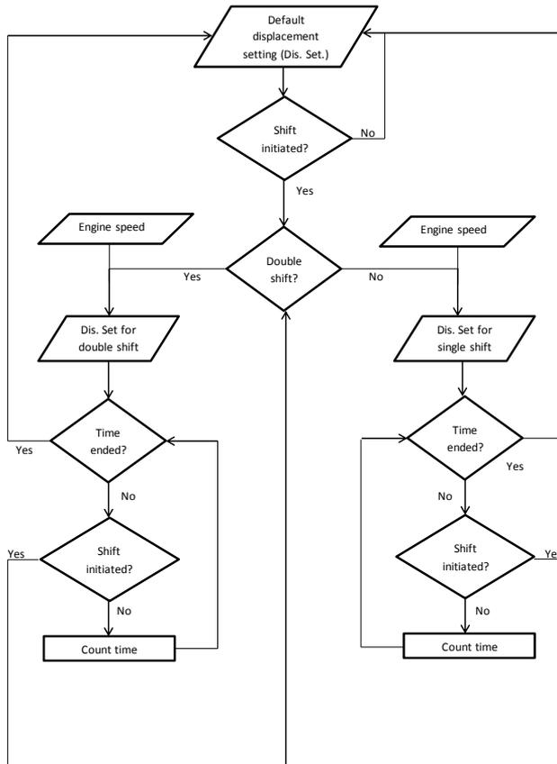
**Figure 5.2:** Control strategy variable displacement pump
