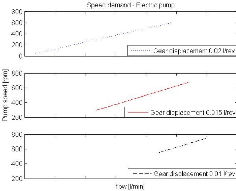
**Figure 4.10:** Speed demands on electric pump when the gear pumps have displacement of 0.02, 0.015 and 0.01 l/rev. The electric pump has a displacement of 0.04 l/rev
