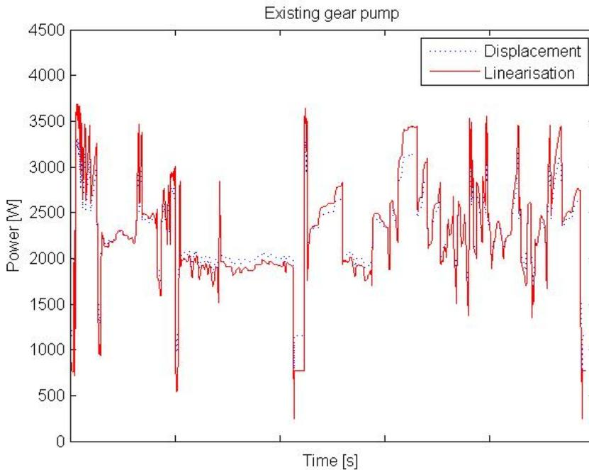
**Figure 6.2:** Power for existing gear pump against time during the drive cycle. The power is based on flow calculated using either displacement or linearisation.
