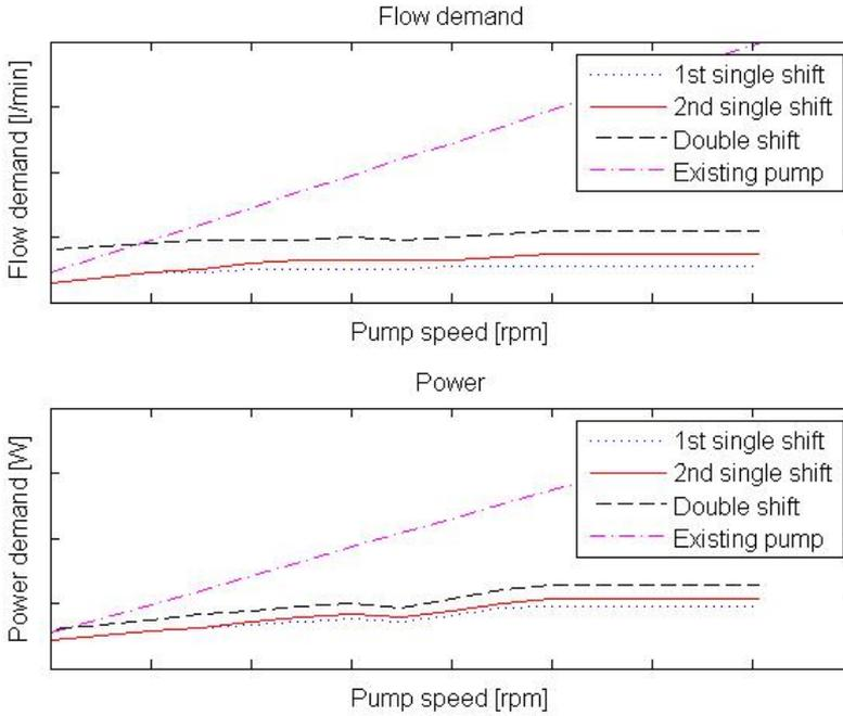
**Figure 4.2:** Demands of flow and power compared with existing pump
