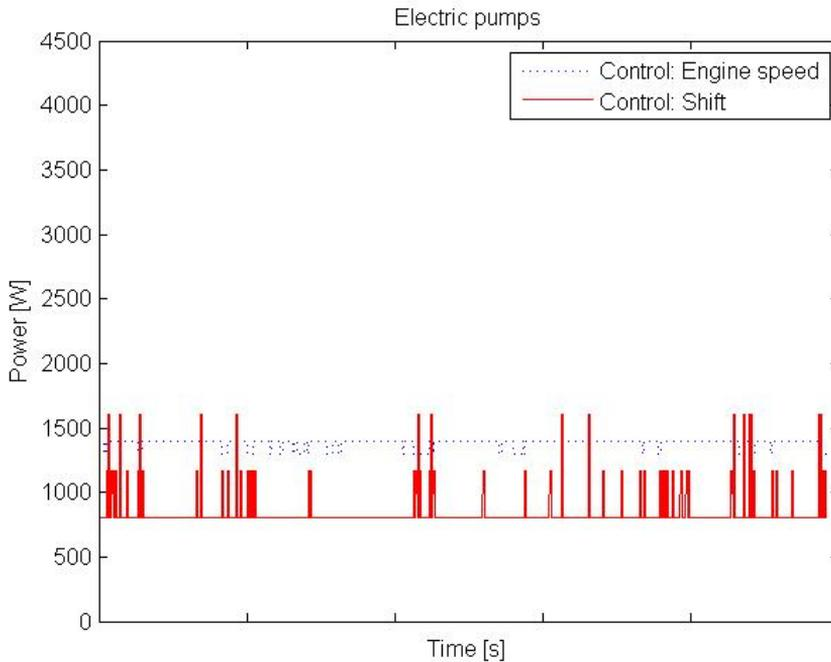
**Figure 6.4:** Power for electric pumps against time during the drive cycle
