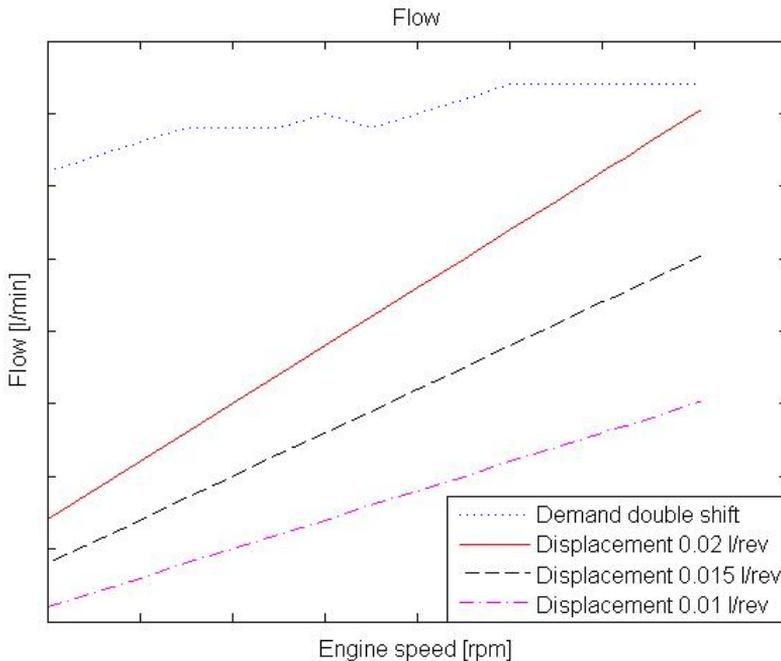
**Figure 4.8:** Flow from gear pumps with displacement 0.02, 0.015 and 0.01 l/rev and the double shifts flow demand
