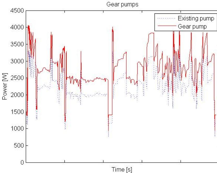
**Figure 6.1:** Power for gear pumps against time during the drive cycle
