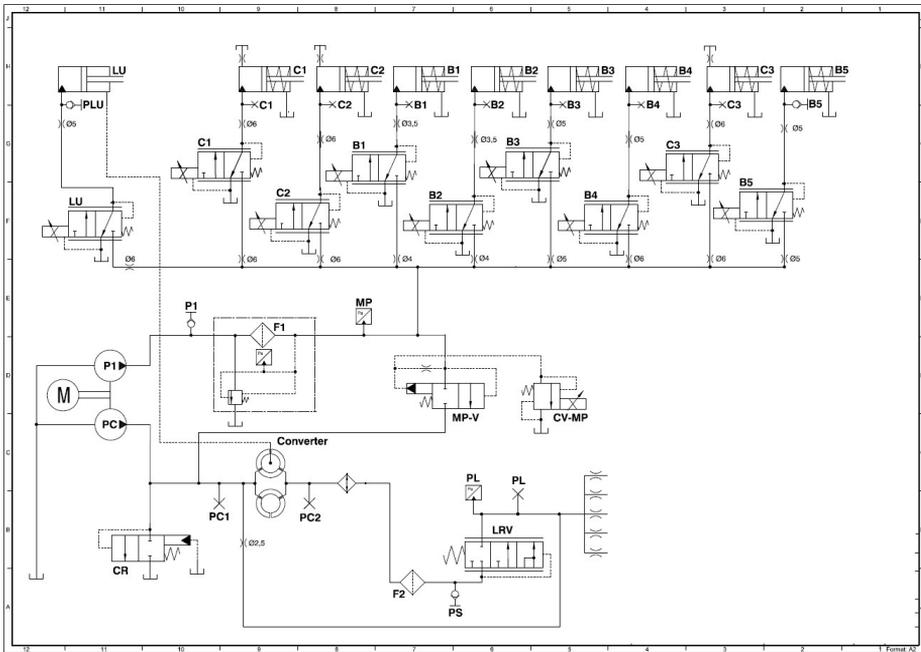
**Figure 2.4:** Hydraulic circuit of the transmission. In the upper part the pistons and valves connected to the gear sets are shown. In the lower part is the converter and the valves used for lubrication of the transmission.
