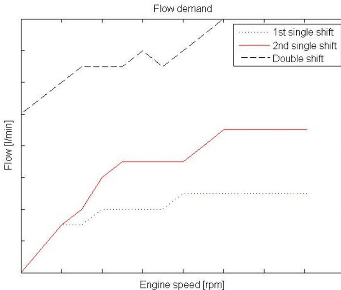
**Figure 3.2:** Example of flow demand for three different shifts against engine speed
