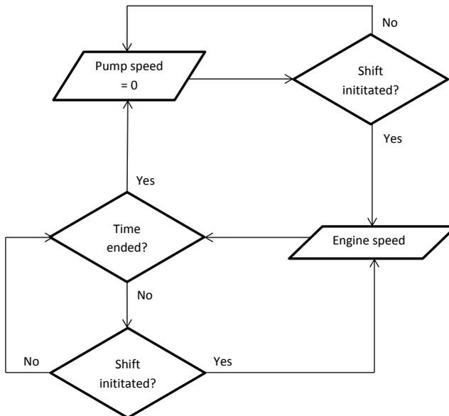
*Figure 5.4: Control strategy for an electric pump when in combination with a gear pump*
