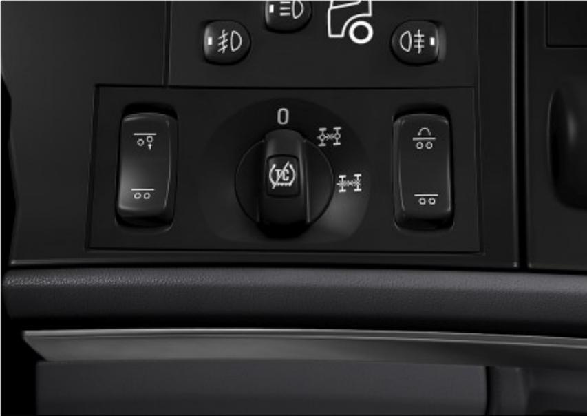
*Figure 5.1: Differential lock control.*
