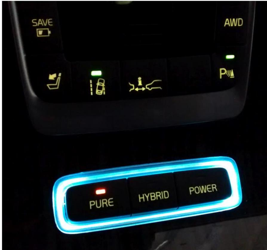
Figure 6: Driving mode buttons on the Volvo V60 PHEV.
