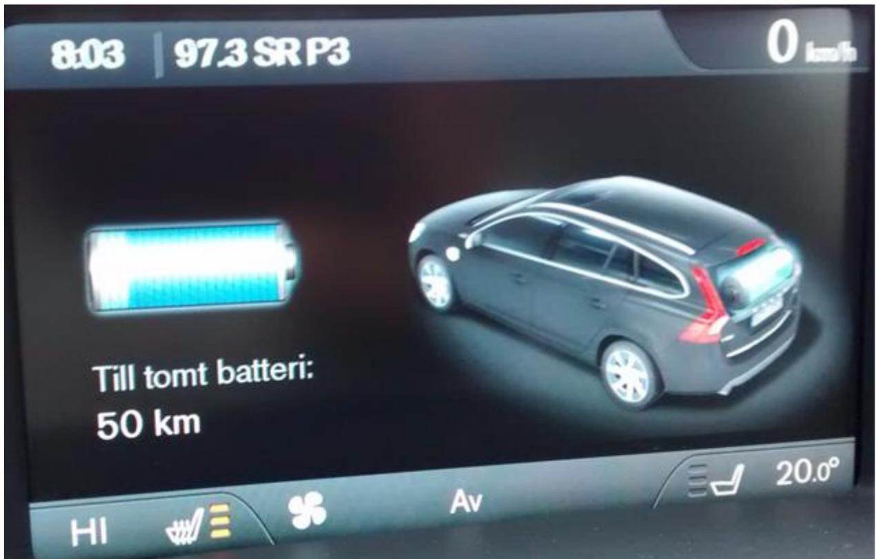
Figure 8: The infotainment display showing a fully charged battery.
