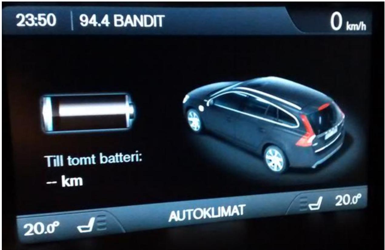
Figure 7: The infotainment display showing a totally depleted battery.
