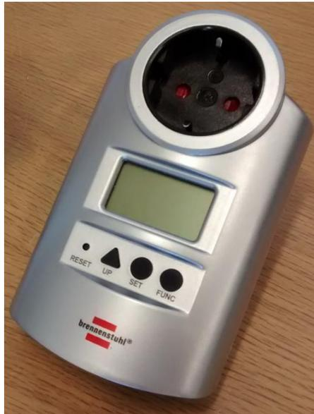
Figure 15: The Brennenstuhl PM 231 E power meter.
