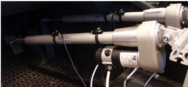
Figure 3.3: Pedal robot mounted in car
