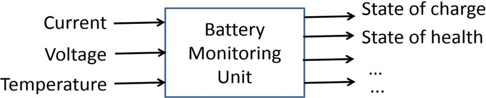
Figure 2.5: Battery monitoring unit scheme
