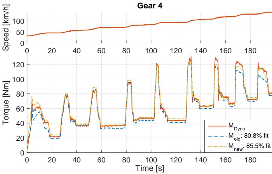
**Figure 7.4:** Powertrain model validation for the fourth gear.
