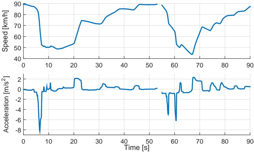
**Figure 4.3:** Example of a "High Velocity with Evasive Maneuver"-study. The figure shows speed and acceleration for a test person from study number 5. The two parts are from different evasive maneuvers performed during the test.
