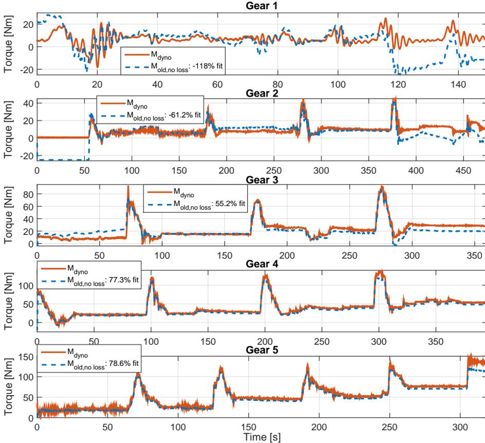
**Figure 5.5:** Comparison of measured and modeled torque, using the full powertrain model. Accelerator pedal position is used as input to the model. The engine speed is held constant at different levels between 1500 to 5000 RPM during the experiment. The torque is scaled with gear and final drive ratio to get it in the same range for all gears.
