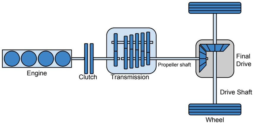
*Figure 2.2: Schematic overview of a vehicle powertrain.*
