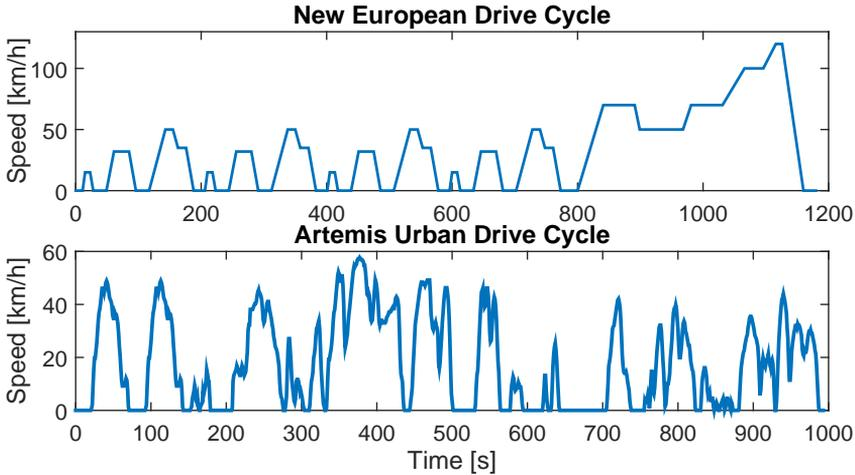
**Figure 2.1:** Two different drive cycles that show the differences between steady state and transient drive cycles. The upper figure shows the steady-state drive cycle NEDC and the lower figure shows the transient drive cycle Artemis Urban.
