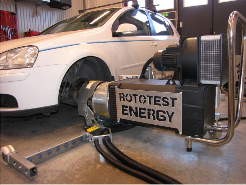
**Figure 3.1:** Dynamometer attached to one of the driven wheel hub of a VW Golf V.
