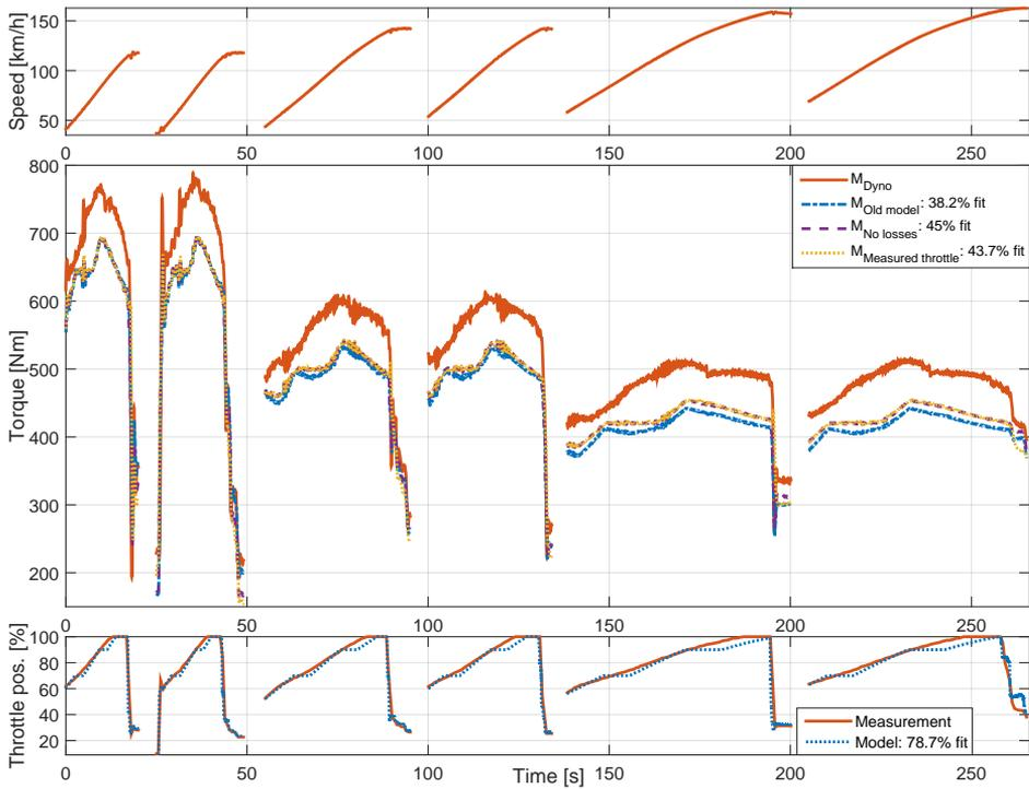
**Figure 5.6:** Dynamic test with maximum accelerator pedal position for third, fourth and fifth gear.
