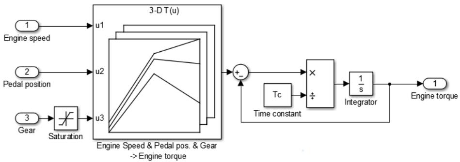
**Figure 6.2:** Simulink scheme of the three dimensional engine map. Pedal position, engine speed and gear are taken as input to the map. The gear signal is saturated between 1 and 3, since the higher gears use the same map. The output then passes through a first order lag element with time constant 0.21.
