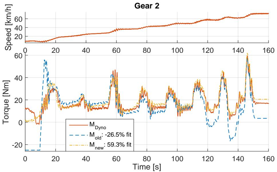
*Figure 7.2: Powertrain model validation for the second gear.*
