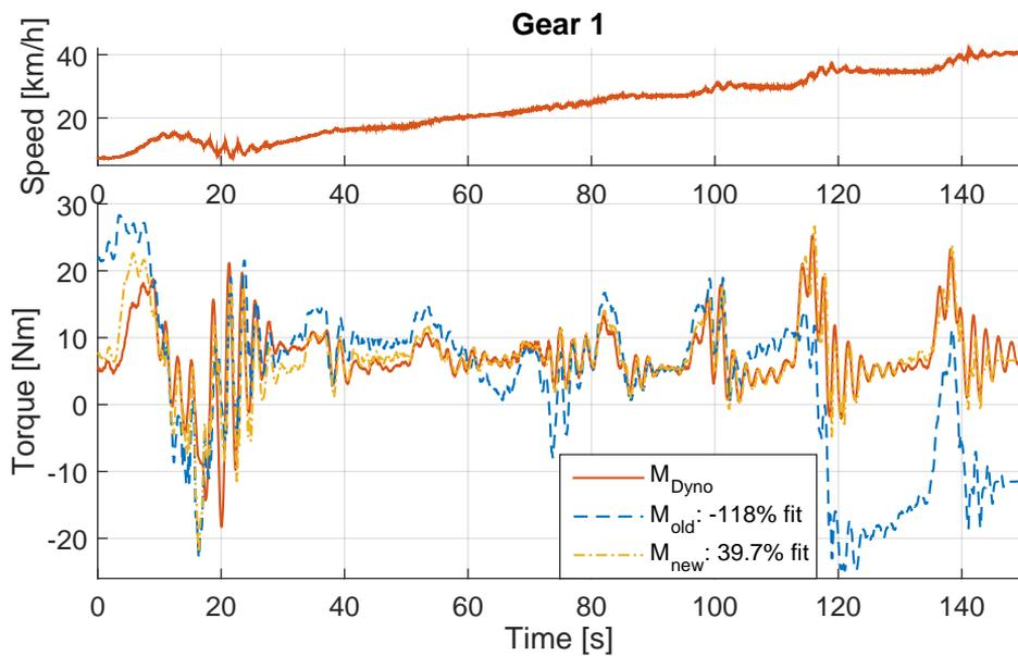
*Figure 7.1: Powertrain model validation for the first gear.*
