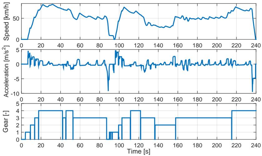
**Figure 4.4:** Example of a "Mixed Driving"-study. The figure shows speed, acceleration and gear for a test person from study number 3.
