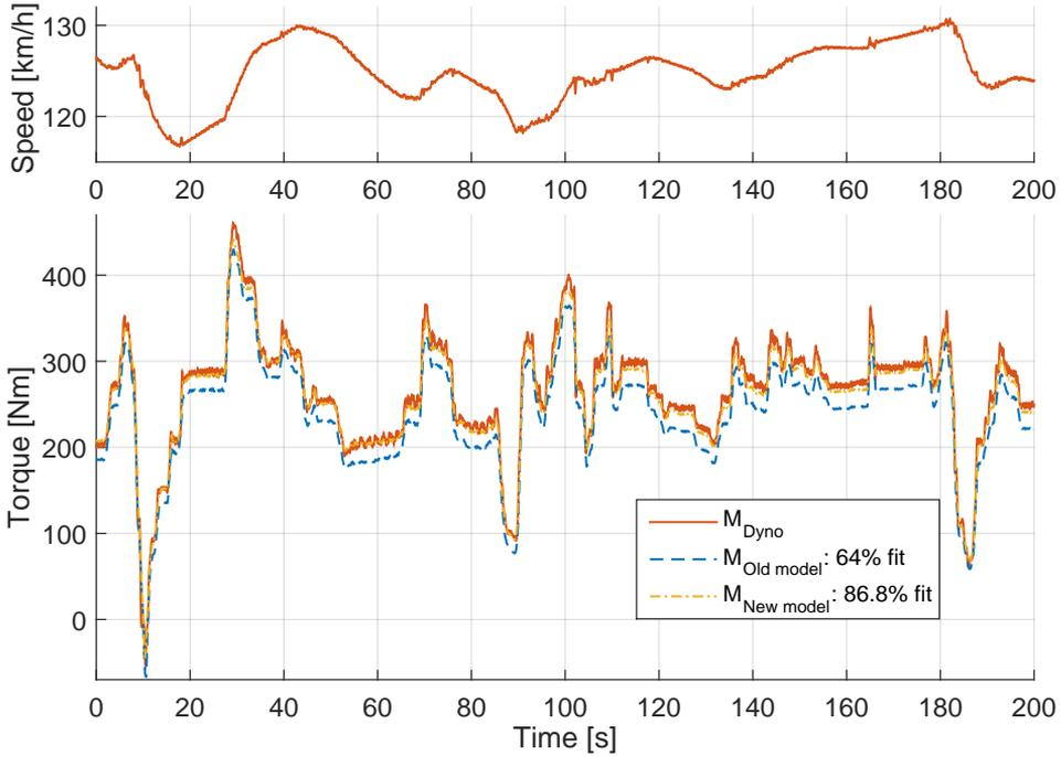
**Figure 7.6:** Comparison between measured and modeled wheel torque using a smaller data segment from data that resembles the Artemis Motorway 130 drive cycle.
