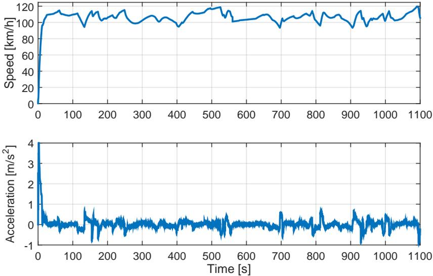
**Figure 4.2:** Example of a "High Constant Velocity"-study. The figure shows speed and acceleration for a test person from study number 6.
