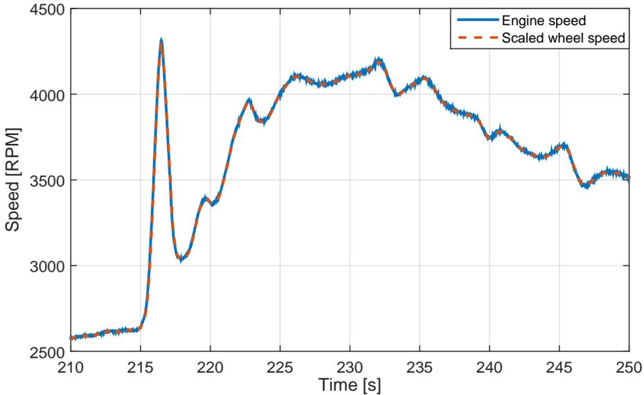
*Figure 5.8: Comparison between engine speed and wheel speed. The wheel speed is the mean value of the two driven wheels, scaled with the combined gear and final drive ratio for the first gear.*
