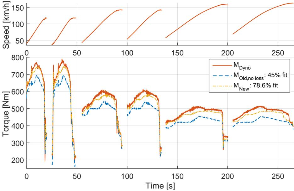
**Figure 7.7:** Comparison between measured and modeled torque. The accelerator pedal is fully pressed during the test and each gear from three and higher is tested twice.
