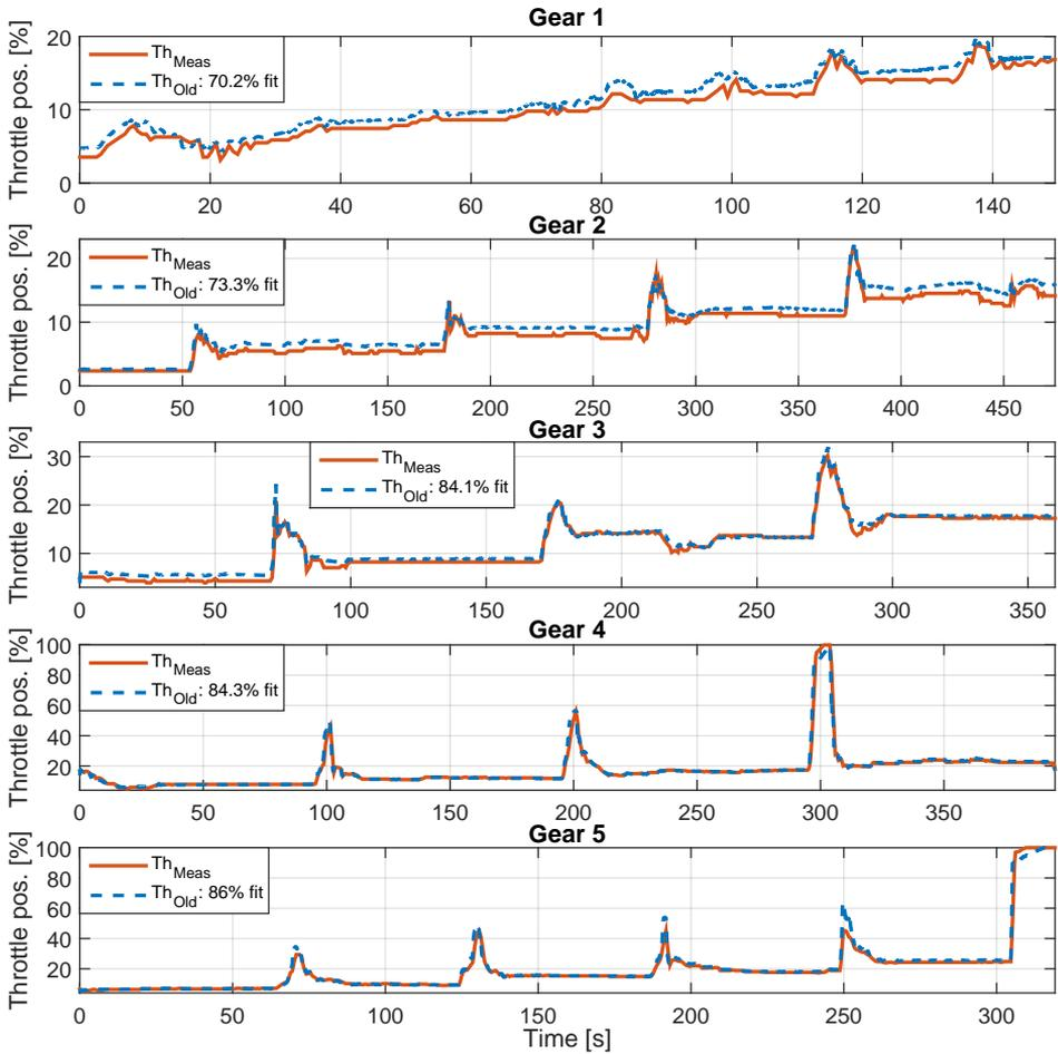
**Figure 5.3:** Comparison of measured and modeled throttle position. The figure shows throttle positions for each gear. During the experiment, the engine speed is held constant at different levels ranging from 1500 to 5000 RPM. Measured accelerator pedal position is used as input to the throttle map.
