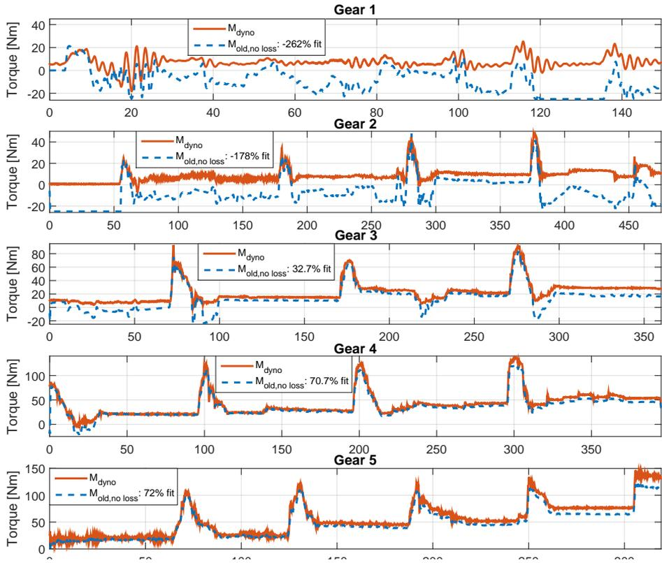
**Figure 5.4:** Comparison of modeled and measured torque at the wheels, using the engine map and the driveline model. The measured torque is scaled with the combined final drive and gearbox ratio. The engine speed is held constant at different levels between 1500 to 5000 RPM. The oscillations in the first figure come from the dynamometers when performing measurements on the first gear.
