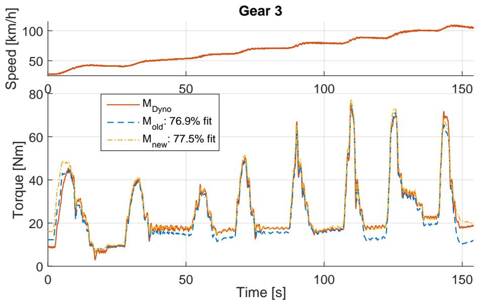
*Figure 7.3: Powertrain model validation for the third gear.*
