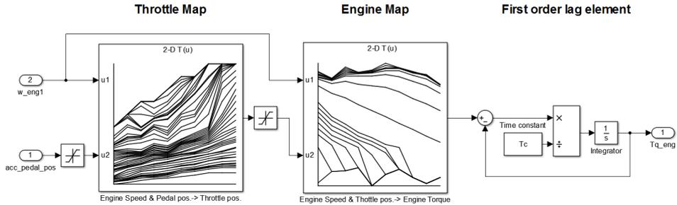
**Figure 5.1:** Simulink schematic of the former engine model. The accelerator pedal position is saturated between 0 and 1. The throttle position is saturated between 4 and 100. The time constant is 0.21.
