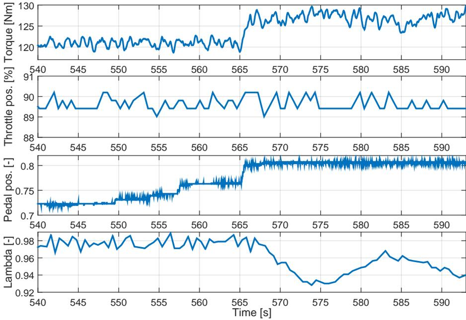
**Figure 5.7:** Extracted from data that was used to make the throttle and engine map. The engine speed is held constant at 4000 RPM.
