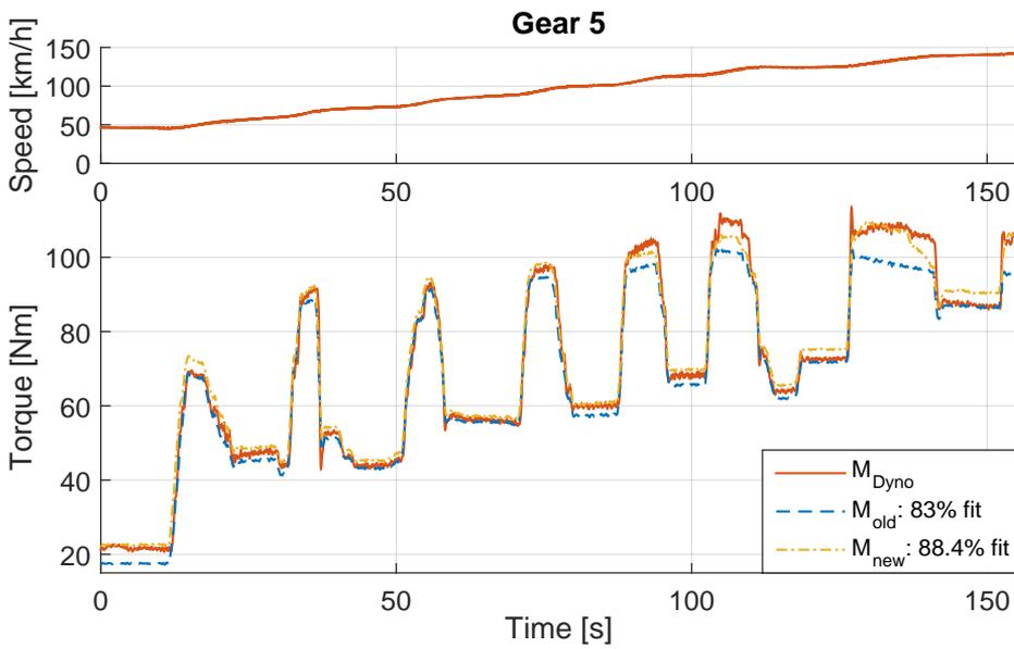
**Figure 7.5:** Powertrain model validation for the fifth gear.
