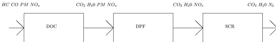
**Figure 3.2:** Aftertreatment system overview in the studied vehicle. The chemical formulas noted above the arrows defines the emissions that are present in the exhaust flow, assuming that ideal emission reduction capability is possible. After all components, the emissions are reduced to  $CO_2$ ,  $H_2O$  or  $N_2$ .
