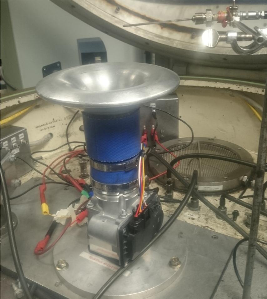
*Figure 4.2: Here a standard Volvo throttle housing is mounted with sensors in the flow bench at VCC, a loss free cone is used to reduce inlet turbulence.*
