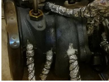
**Figure 4.3:** Thermocouples glued on the turbine housing.
