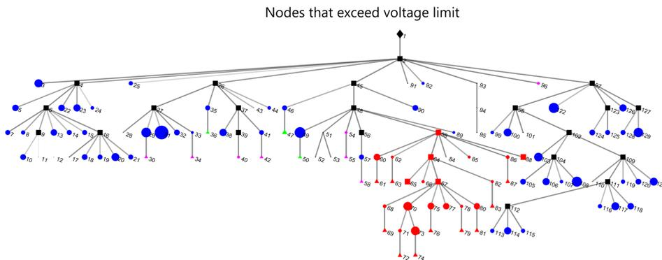
**Figure 4.3:** Shows voltages of +7% of 230 V during a year as red. These nodes are all nodes from Node 59 to Node 88. Note that out of these nodes there are 10 PV-systems, these are illustrated as red triangles.
