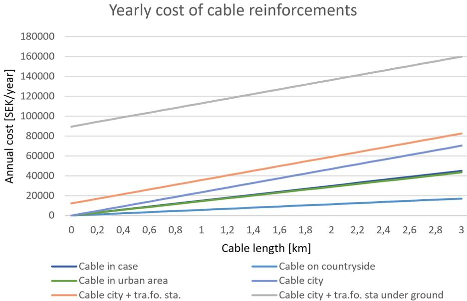
**Figure 2.4:** Graph showing the annual cost of different cable reinforcements. Calculated based on the table above, and with a life length of 40 years. These include different combinations of cables and transformers etc. in different types of landscapes.
