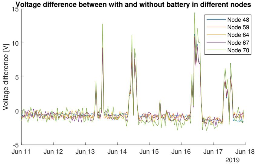
**Figure 4.12:** Graph showing the voltage difference in the battery node caused by the battery charging and discharging. Each line comes from a simulation where that node is the battery node. Note that the voltage difference peaks all have similar magnitudes no matter where the battery is placed, except when the battery is placed in the most optimal node, Node 70.
