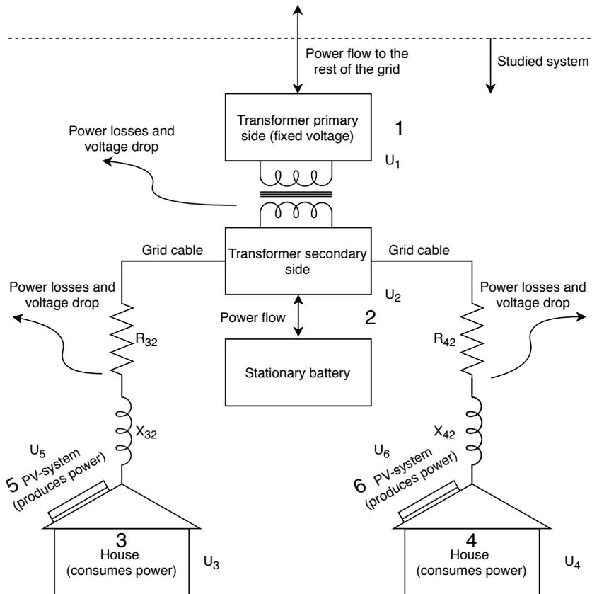
**Figure 2.1:** An example of what a simple grid could look like. This grid contains the different components/models that will be studied in this thesis. The numbers shown in the figure are the node numbers and these are the same as in Figure 2.2. Note that Node 2 is both the secondary side of the transformer and contains in this case a stationary battery.
