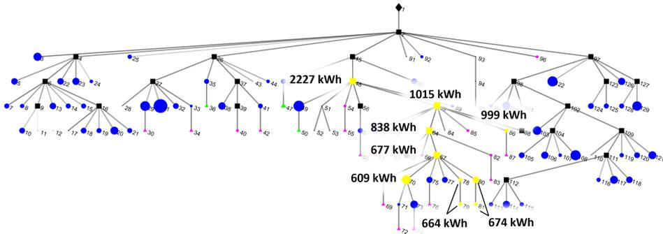
**Figure 4.8:** The grid and the different nodes where a single battery can be placed to stabilise the grid enough (marked in yellow). Next to these nodes the least amount of battery capacity needed is stated. These numbers and nodes can also be seen in Table 4.2. Note that the battery capacity needed when a battery is placed in Node 88 is slightly lower than when placed in Node 59. This can be explained with increased power losses in the additional cable, see Section 2.1.
