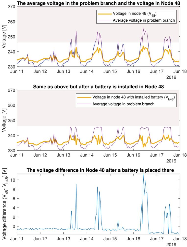
**Figure 4.11:** Illustration of the average voltage in the branch with the highest voltages (where most PV-systems are, Node 67-81) and Node 48, both before and after the battery is placed in that node. It can also be seen that the voltage difference in Node 48 (lowest graph) has similar characteristics as the peaks without a battery (voltages in the red area of the top graph). The third graph for different battery placements can be seen in Figure 4.12
