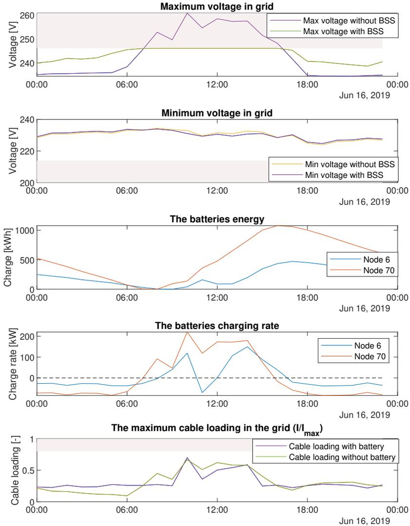
**Figure 4.20:** The grid with added PV-systems simulated with a battery in node 6 and node 70
