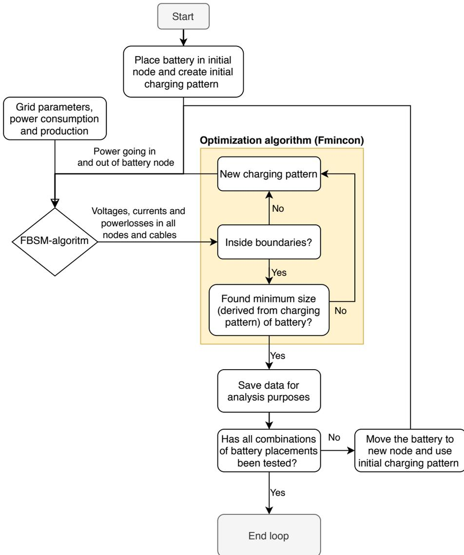
**Figure 3.4:** Figure showing how the different algorithms are used together to find the optimal placement and sizing of one or more batteries in a grid. The Optimisation algorithm is described in Section 3.2.1 Battery size optimisation algorithm and the FBSM-algorithm is described in Section 3.3 Simulation
