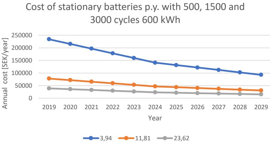
(b) Comparison done for a 600kWh sized battery above.
