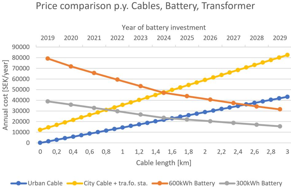
**Figure 4.24:** A comparison of the yearly cost of batteries compared to a transformer with cable reinforcements.
