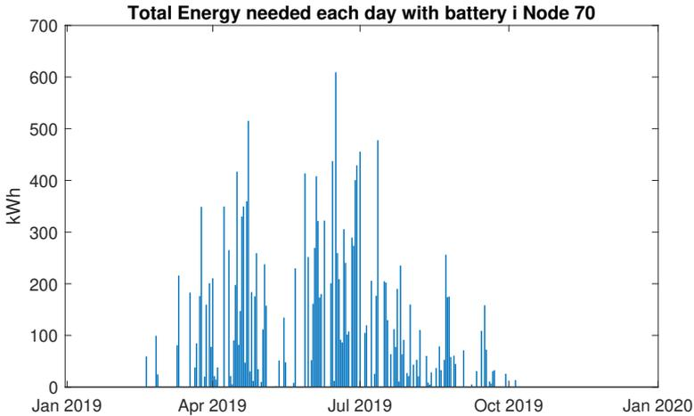
**Figure 4.18:** Histogram, showing energy needed each day in the system to keep all voltages in between  $\pm 7\%$  of 230 V and the cable loading below 80%. The total numbers of days the battery is needed is 125, which is shown in the figure as the number of bars.
