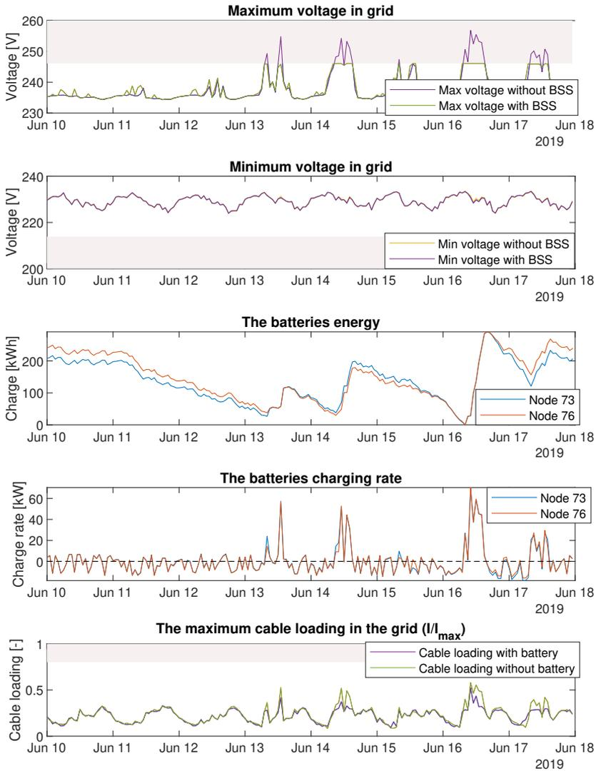
*Figure 4.15: One week simulation with batteries in node 73 and node 76.*
