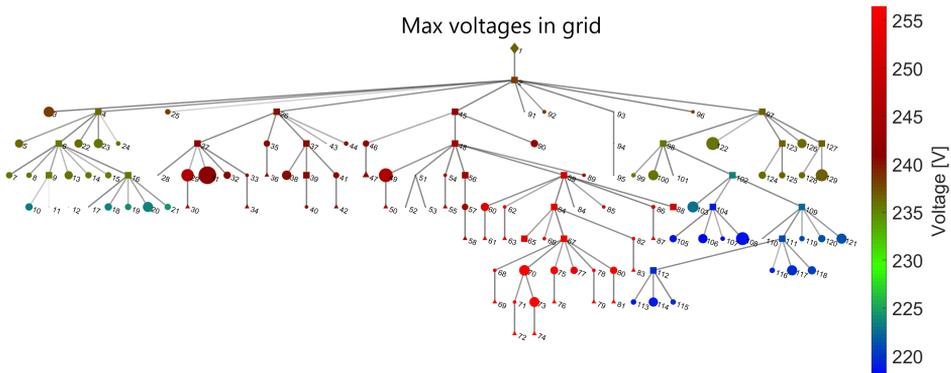
**Figure 4.2:** The grid where nodes colored according to the color bar on the right. The values are the voltages in each node that deviates the most from the nominal voltage (230 V) during one year.
