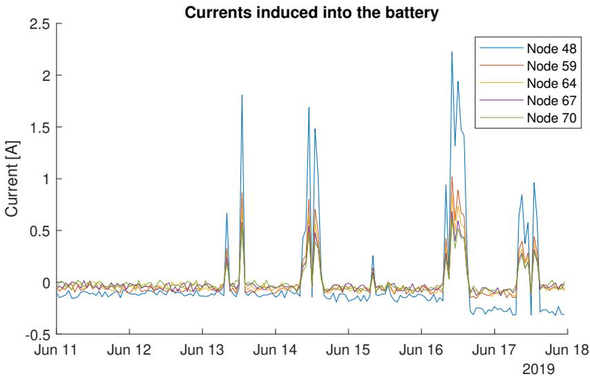
**Figure 4.13:** Graph showing the current going in and out of the battery for different battery placements. Note that the peak currents are higher when the battery is placed in a node closer to the transformer.
