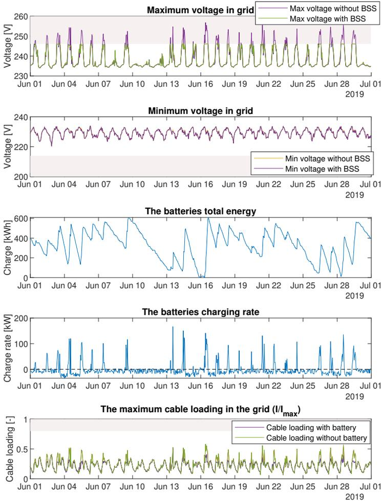
**Figure 4.17:** Illustration of maximum and minimum voltage, SoC variations and cable loading for a stationary battery in node 70. Note that the day that dimensions the size of the battery capacity is June 16 (the charge reaches both the top and the bottom during this day) and that the battery reinforced grid behaves similarly to the cable reinforced grid, in terms of cable loading as well as maximum and minimum voltage.
