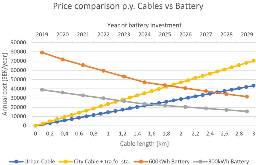
**Figure 4.23:** A per year price comparison between the cost of a cable and a 600kWh battery with a lifetime of 11.81 years. The projected price changes of the batteries are from Bloomberg, and distance of cables is in kilometers.
