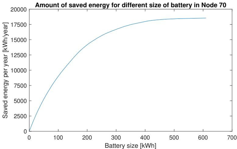
**Figure 4.19:** Graph showing how the amount of energy that can be saved per year using different battery capacity. In this simulation the battery was placed in the most optimal place, Node 70. Since this is highly non-linear a smaller battery might be a better option than a larger one. For example a battery of 300 kWh can save as much as 90% of what a battery of twice that size can. For further understanding of why this is not linear, see Figure 4.18
