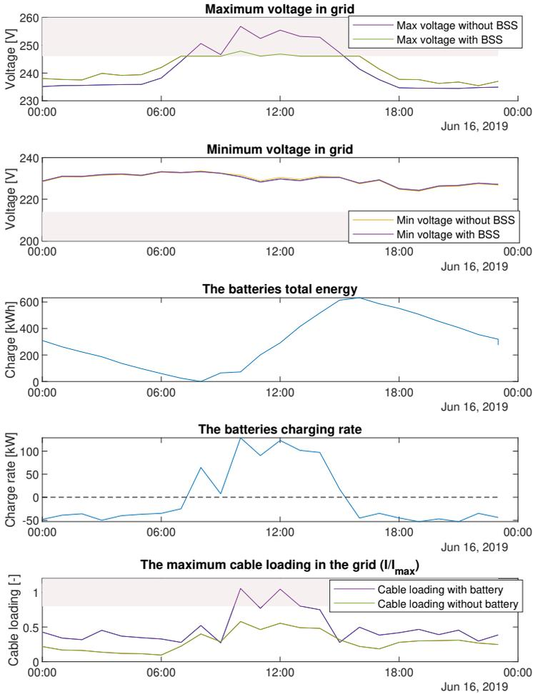
**Figure 4.10:** Illustration of maximum and minimum voltage, SoC variations and cable loading for a stationary battery in node 68. Note that the maximum voltage is almost below the maximum allowed voltage in all time steps with BSS. The reason why these voltages can not be brought down is that the cables are too weak and the maximum cable loading is exceeded in the same time steps.
