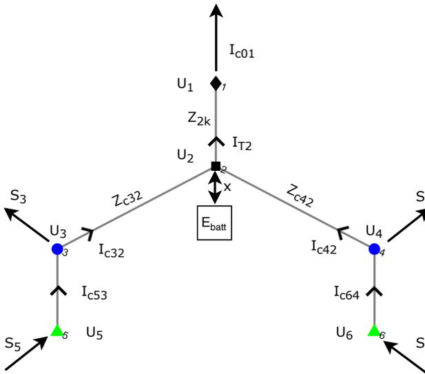
**Figure 2.3:** Another illustration of the grid shown in Figure 2.1. It is the same as 2.2 but also including the currents, voltages, powers and impedances, as well as the battery's charge and power exchange with the grid. These parameters shown are the primary parameters used in the modelling and the solver described in Chapter 3. The color scheme is also described in 4.1
