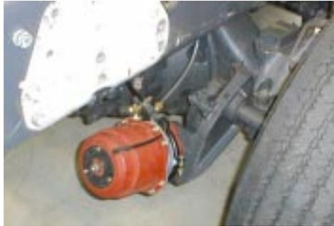
Figure 4.7: Brake cylinder fitted on vehicle (drum brake)
