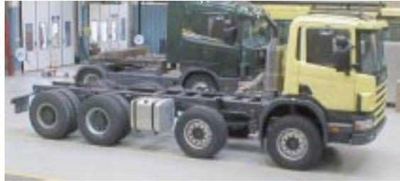
Figure 2.1: Eight-wheeled vehicle with two front axles
