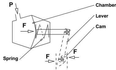
Figure 4.8: Brake cylinder schematic
