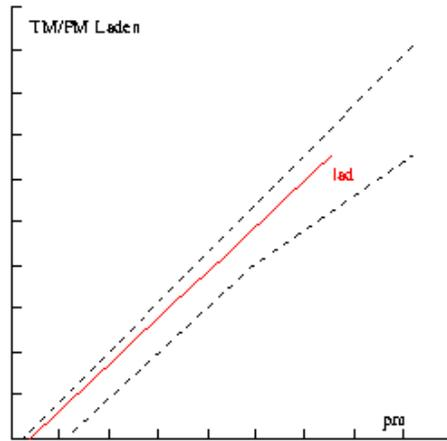
Figure 4.10: Braking rate with tolerance acc. to 71/320/EEC
