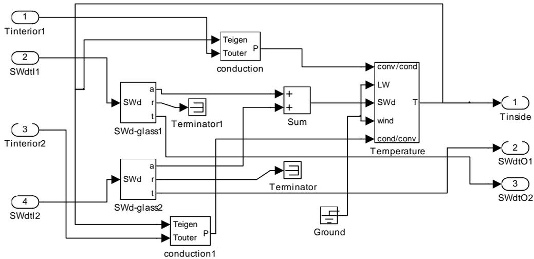
Figure 5.11 Inside the insideglass block.
