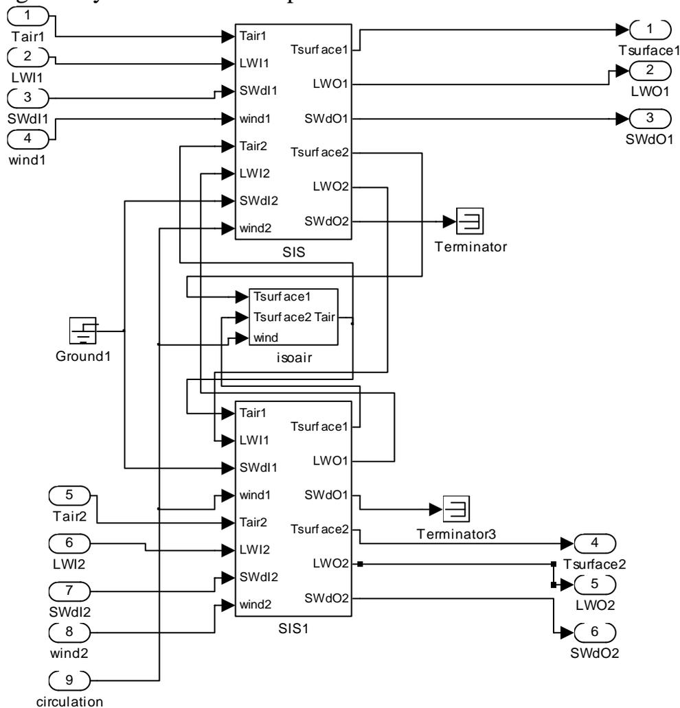
Figure 7.19 Inside the SISASIS block.
