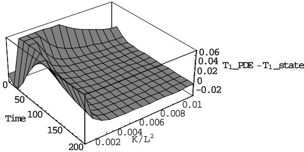
Figure 3.7 shows  $T_{PDE}(\frac{5}{6}, t) - T_{1,state}(t)$  for different values of  $\frac{\kappa}{L^2}$ .
