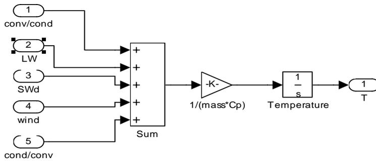
Figure 5.1 Inside the temperature block
