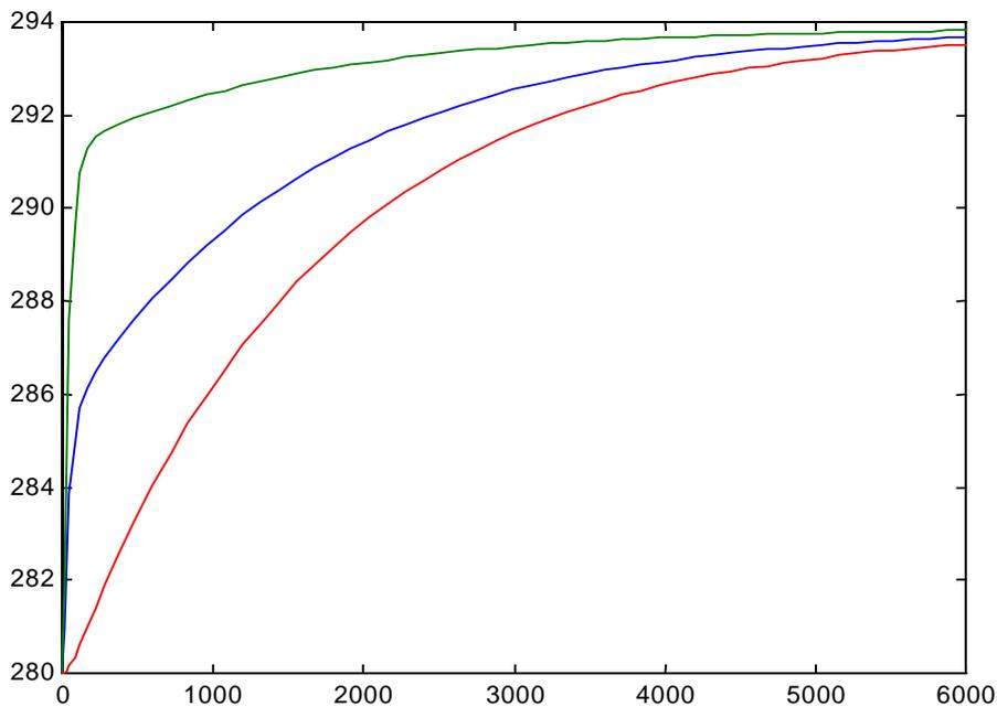
Fig 5.9 Fan speed:L, wind: L , Fan air temp: L->H (Exp 5,simulated) x-axis: time in seconds, y-axis: temperature in Kelvin
