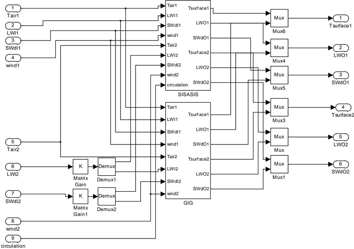
Figure 4.4 Inside the ROOF block
