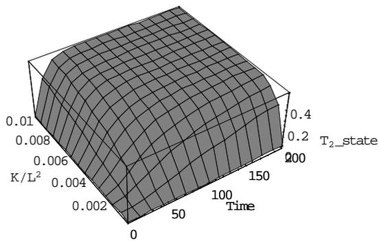
Figure 3.4 shows the step response for  $T_2$  as a function of  $\kappa/L^2$  when  $\Delta T = 1$ . The final value is  $1/2$ .
