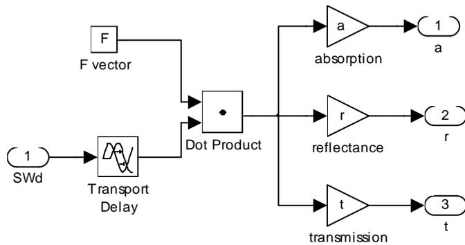
Figure 5.7 Inside the SWd\_glass block.
