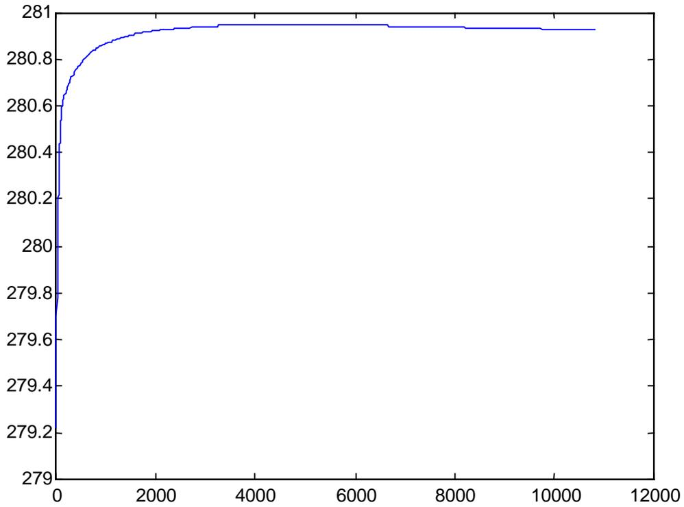
Fig 5.6 Fan speed:L-> H, wind: L , Fan air temp: L (Exp 8, simulated) x-axis: time in seconds, y-axis: temperature in Kelvin
