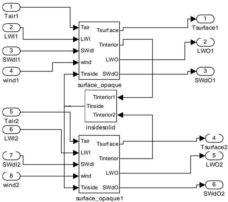
Figure 5.14 Inside the SIS block.
