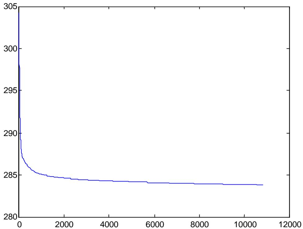
Fig 5.4 Fan speed: H, wind: H, Fan air temp: H->L (Exp 3, simulated) x-axis: time in seconds, y-axis: temperature in Kelvin
