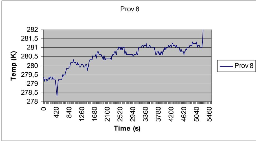
Fig 5.5 Fan speed: L->H, wind: L , Fan air temp: L (Exp 8) x-axis: time in seconds, y-axis: temperature in Kelvin
