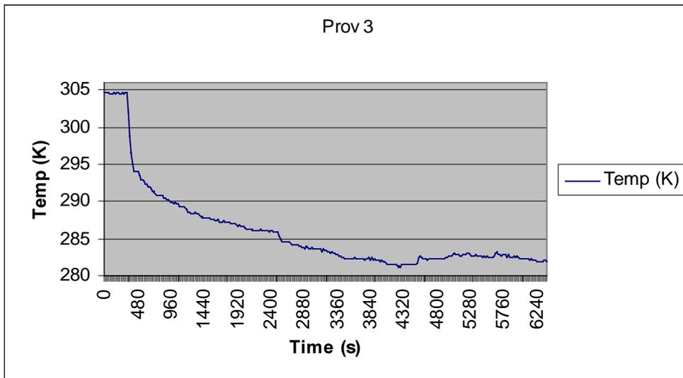
Fig 5.3 Fan speed: H, wind: H, Fan air temp: H->L (Exp 3) x-axis: time in seconds, y-axis: temperature in Kelvin
