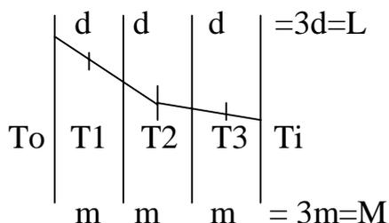
Figure 3.1 shows the temperature distribution for a homogenous wall at a non-steady state.
