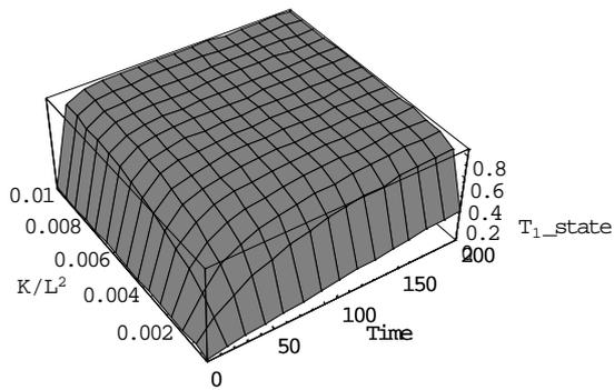
Figure 3.3 shows the step response for  $T_1$  as a function of  $\kappa/L^2$  when  $\Delta T = 1$ . The final value is  $5/6$ .
