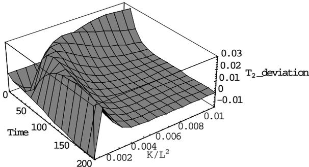
Figure 3.8 shows  $T_{PDE}(\frac{1}{2}, t) - T_{2,state}(t)$  for different values of  $\frac{\kappa}{L^2}$ .
