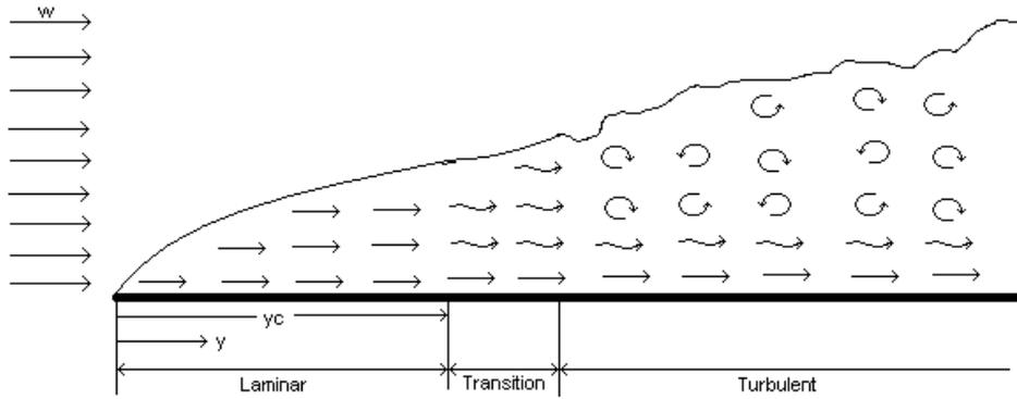
Figure 2.2 shows how the air behaves depending on the distance from the leading air.
