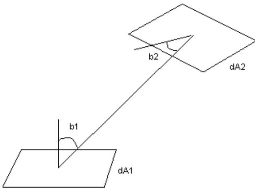
Figure 3.10 shows the radiative exchange between two surface elements.
