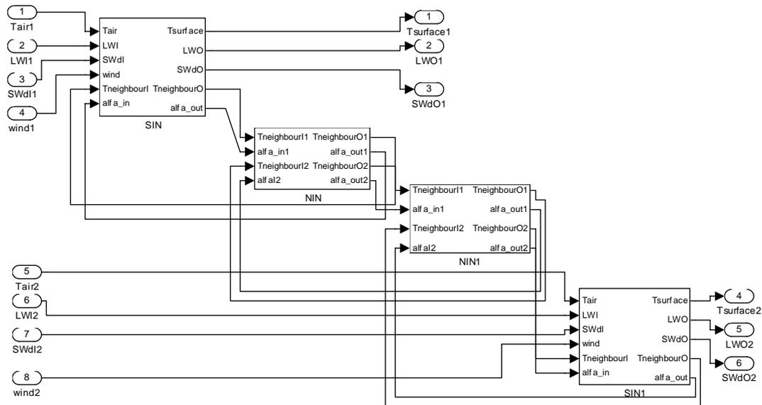
Figure 5.21 Inside the SINNINNINNIS block.
