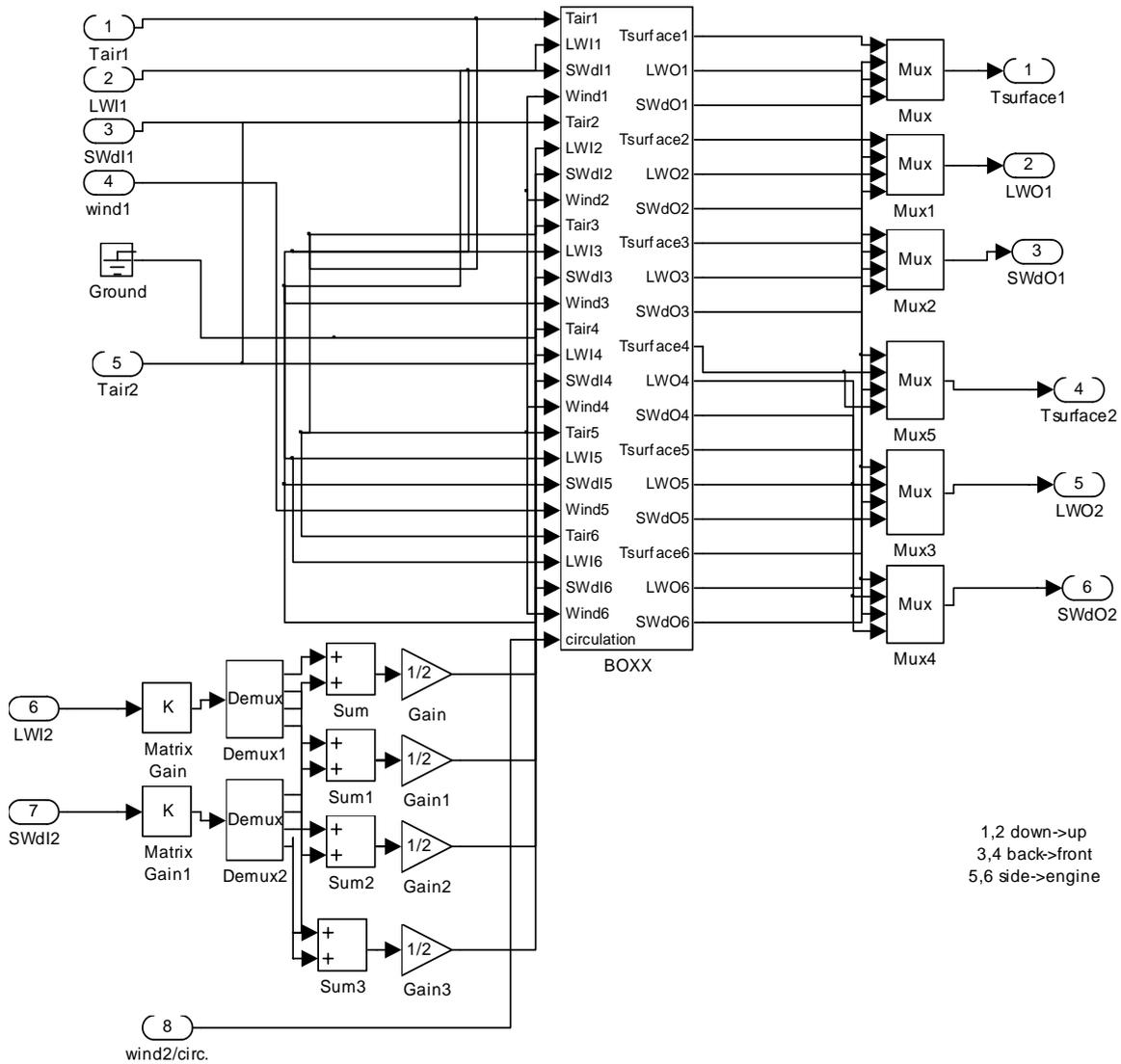
Figure 4.14 Inside the box right /left block
