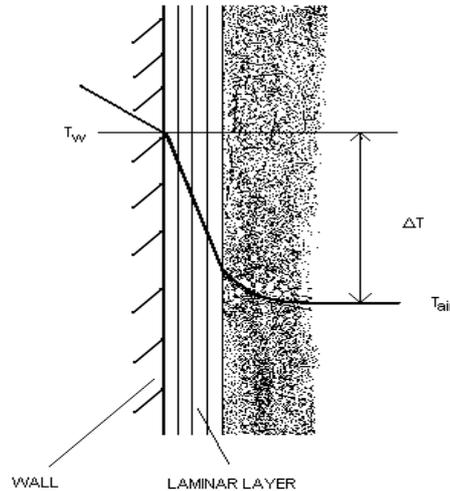
Figure 2.1 shows the temperature distribution for forced convection
