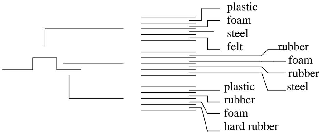
Figure 4.7 The floor structure.
