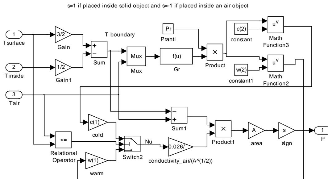
Figure 5.2 Inside the convection block.
