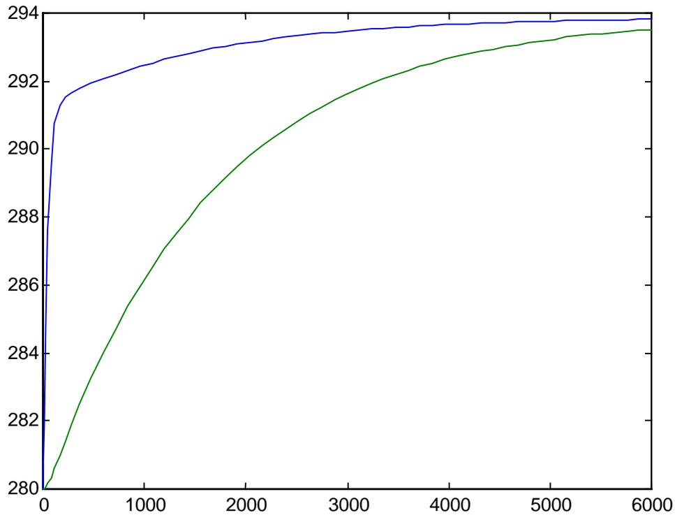
Fig 5.8 Fan speed:L, wind: L , Fan air temp: L->H (Exp 5,simulated) x-axis: time in seconds, y-axis: temperature in Kelvin
