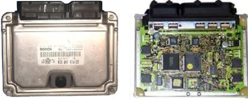
FIGURE 1.1: Outside and inside of an ECU by Bosch for an Audi personal vehicle. The ECU includes electronic components and software.
