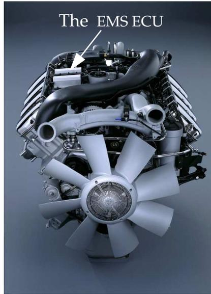
FIGURE 2.2: The figure shows a 16 liter 500 hp heavy duty truck engine from Scania (Scania, 2007). The engine management system (EMS) is attached to the upper part of the engine. This engine fulfills the Euro 5 emission restrictions using among other things a selective catalytic reduction system (SCR) for after-treatment of the exhaust gases.
