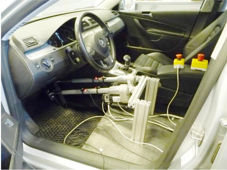
Figure 11: Pedal robot that was used to actuate the gas and brake pedal according to the input from the driver in the Sim III simulator.
