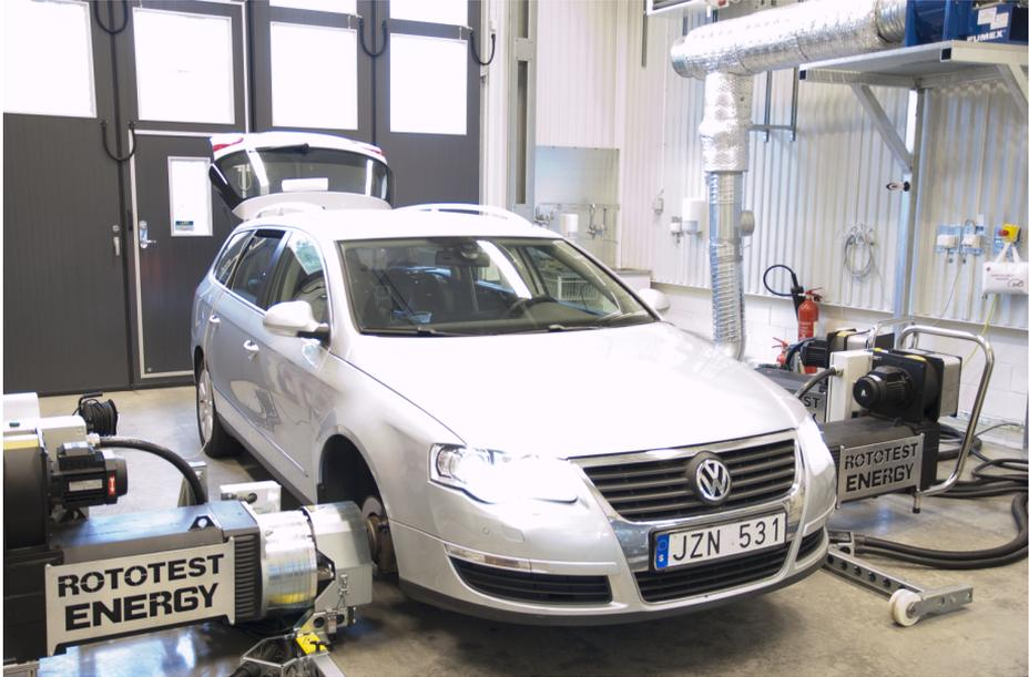
Figure 2: Volkswagen Passat that is used in the experiment mounted in the chassis dynamometer of the vehicle propulsion laboratory.
