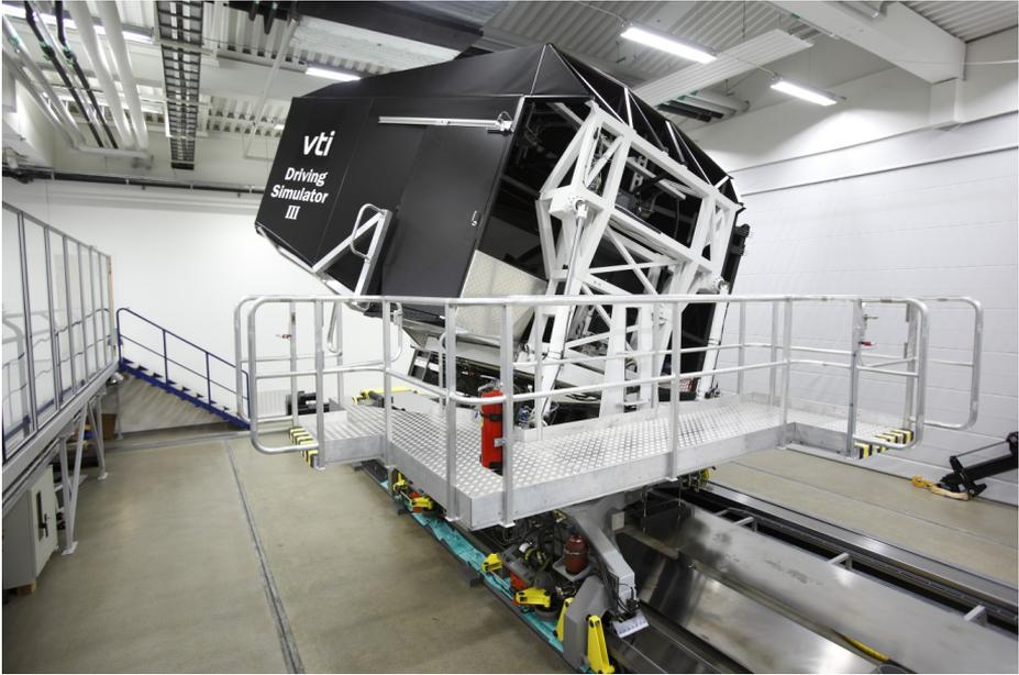
Figure 1.5: Moving base simulator Sim III.
