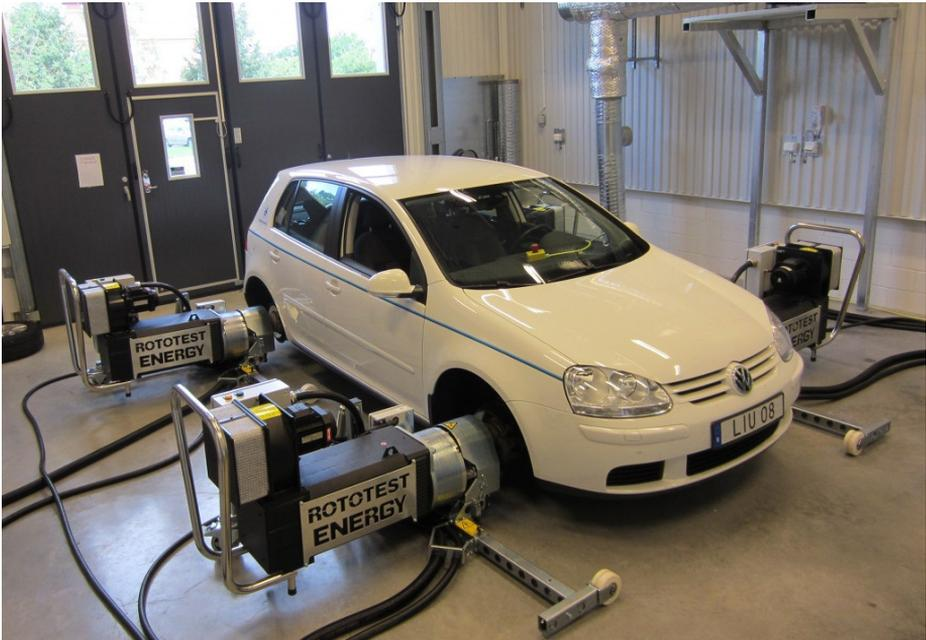
Figure 1: Glance of the new chassis dynamometer lab. A Golf V with a 1.4l multifuel engine has been mounted to the dynamometer units in a 4WD configuration.
