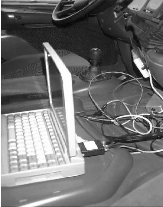
**Figure 3.7** Experiment situation. A PC with parallel-port CAN board attached to the CAN-bus in the cab of the truck.
