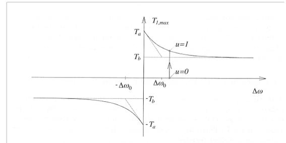
Approximation of the maximum torque in a friction clutch
