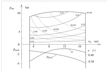
Willans line parameters:  $e(\omega_e)$   $\rho_{me,0}(\omega_e)$
