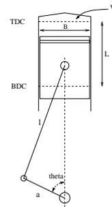
Cylinder, Piston, Connecting rod, Crank shaft
