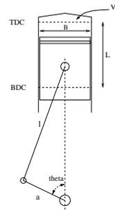
Cylinder, Piston, Connecting rod, Crank shaft
