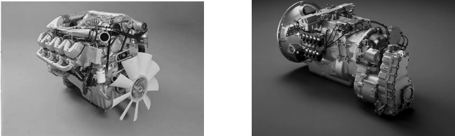
Scania 14 liter V8 DSC14 engine. Scania transmission with retarder and OptiCruise automatic gear-shifting system.
