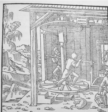
Human muscles remained indispensable prime movers until the widespread adoption of engines and motors. In the first illustration two men on a cleated treadwheel raise water buckets in a German mine in the sixteenth century. In the second eight men rotate a vertical capstan drawing a gold wire in an eighteenth-century French workshop.
