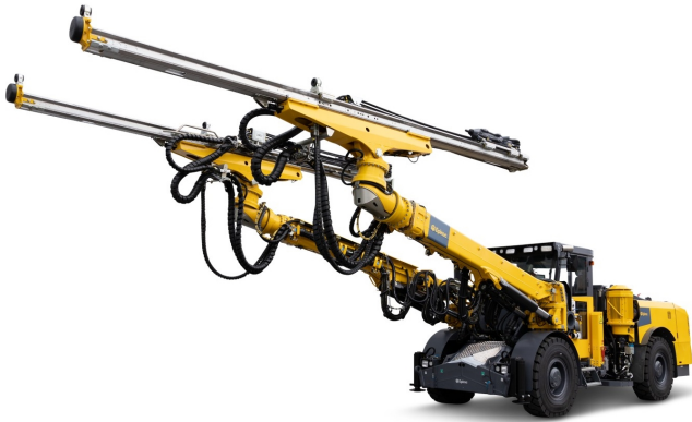
Figure 1. An underground drill rigs, typically used for the target system
