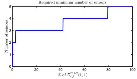
Fig. 2. The least number of sensors required to exceed a certain percentage of maximum distinguishability given the example model (1). Note that the number of sensors when required performance goes to zero is equal to the cardinality of the minimal sensor sets (2) from the structural analysis.
