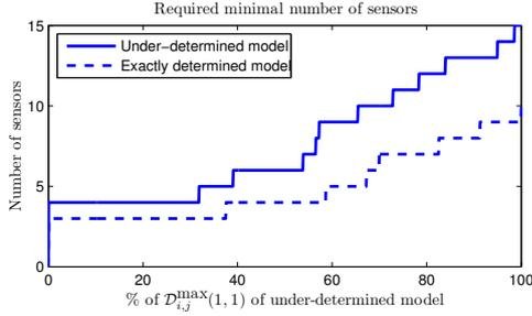
Fig. 4. The least number of sensors required to exceed a certain percentage of maximum distinguishability given the underdetermined model described in Figure 3, for the underdetermined case and the exactly determined case, given a global search.
