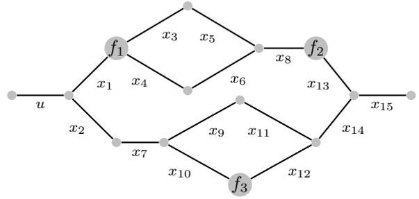
Fig. 3. A schematic overview of a model describing a static flow through a number of nodes. The input  $u$  is known and the flows through the branches  $x_i, i = 1, 2, \dots, 15$ , are unknown, and  $f_1, f_2, f_3$  are three additive faults.
