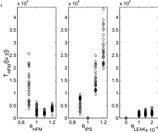
**Figure 5.15** Test quantities calculated according to (4.1) where  $\hat{y}$  is determined by simulation of the  $LEAK$  fault model and  $\theta_{LEAK}$  is estimated by the pole placement observer.
