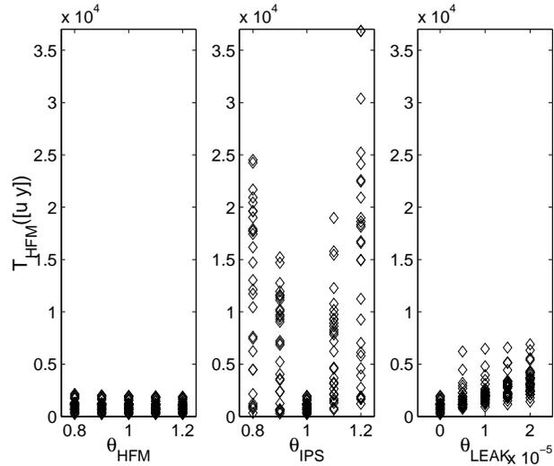
**Figure 5.13** Test quantities calculated according to (4.1) where  $\hat{y}$  is determined by simulation of the *HFM* fault model and  $\theta_{HFM}$  is estimated by the pole placement observer.
