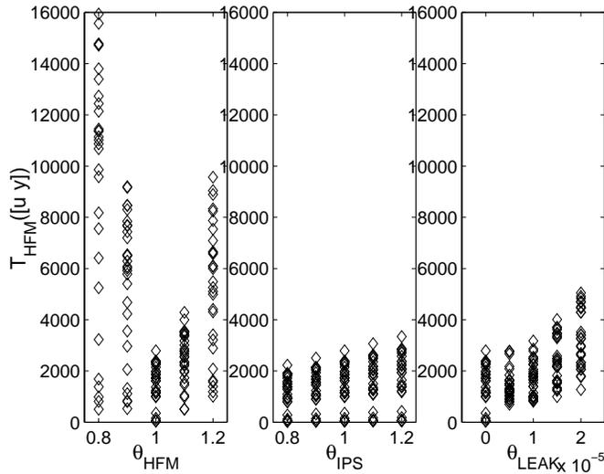
**Figure 5.8** Test quantities calculated according to (4.1) where  $\hat{y}$  is determined by simulation of the IPS fault model and  $\theta_{IPS}$  is estimated by feedback on the fault state only observer.
