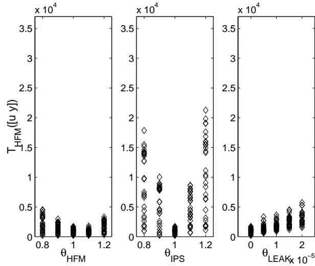
**Figure 5.7** Test quantities calculated according to (4.1) where  $\hat{y}$  is determined by simulation of the HFM fault model and  $\theta_{HFM}$  is estimated by feedback on the fault state only observer.
