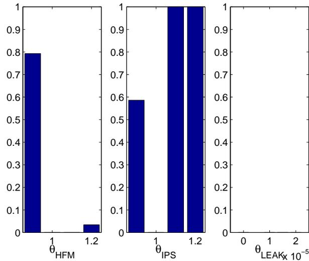
**Figure 5.6** Power function for the hypothesis test  $H_0 : F_p \in \{NF, LEAK\}$  when  $\theta_{LEAK}$  is estimated with feedback on the fault state only observer and  $\hat{y}$  used in (4.1) is obtained by simulating the LEAK fault model.
