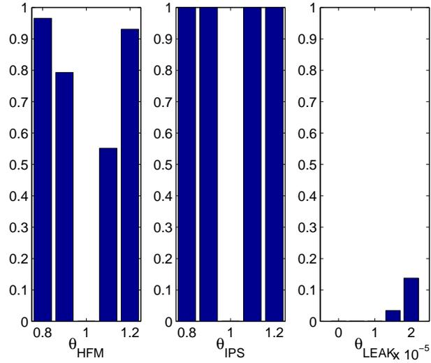
**Figure 5.2** Power function  $\beta_{NF}(\theta_i)$  when the null hypothesis is  $H_0 : F_p = NF$  and the  $NF$  fault model is simulated to obtain  $\hat{y}$  used in (4.1).
