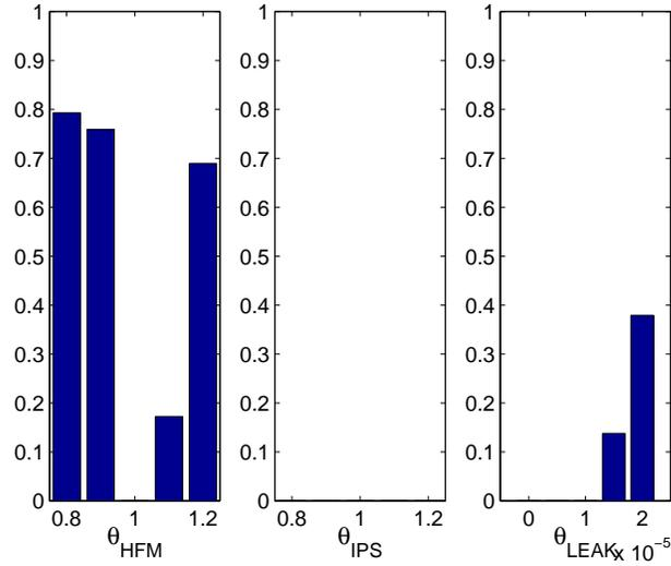
**Figure 5.5** Power function for the hypothesis test  $H_0 : F_p \in \{NF, IPS\}$  when  $\theta_{IPS}$  is estimated with feedback on the fault state only observer and  $\hat{y}$  used in (4.1) is obtained by simulating the IPS fault model.
