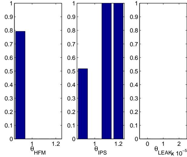
**Figure 5.12** Power function for the hypothesis test  $H_0 : F_p \in \{NF, LEAK\}$  when  $\theta_{LEAK}$  is estimated with pole placement observer and  $\hat{y}$  used in (4.1) is obtained by simulating the *LEAK* fault model.
