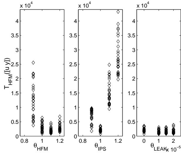
**Figure 5.9** Test quantities calculated according to (4.1) where  $\hat{y}$  is determined by simulation of the LEAK fault model and  $\theta_{LEAK}$  is estimated by feedback on the fault state only observer.
