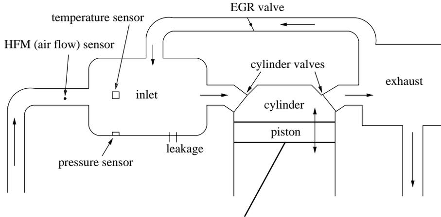
**Figure 3.1** Schematic view of the air intake and exhaust system of a modern diesel engine
