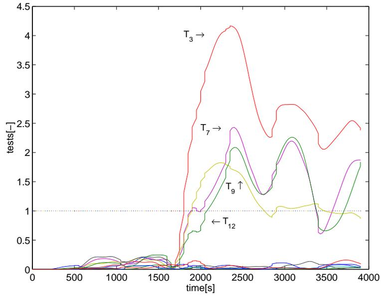
Figure 5.7: Tests for fault in sensor  $y_5$ .
