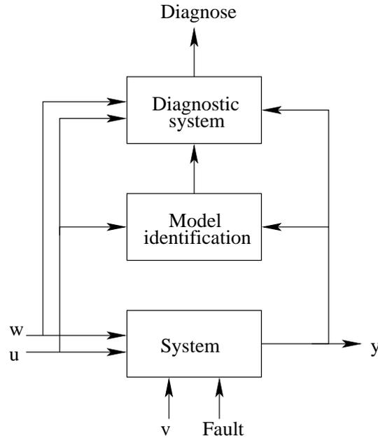
Figure 2.1: Schematic picture of a model based diagnostic system.
