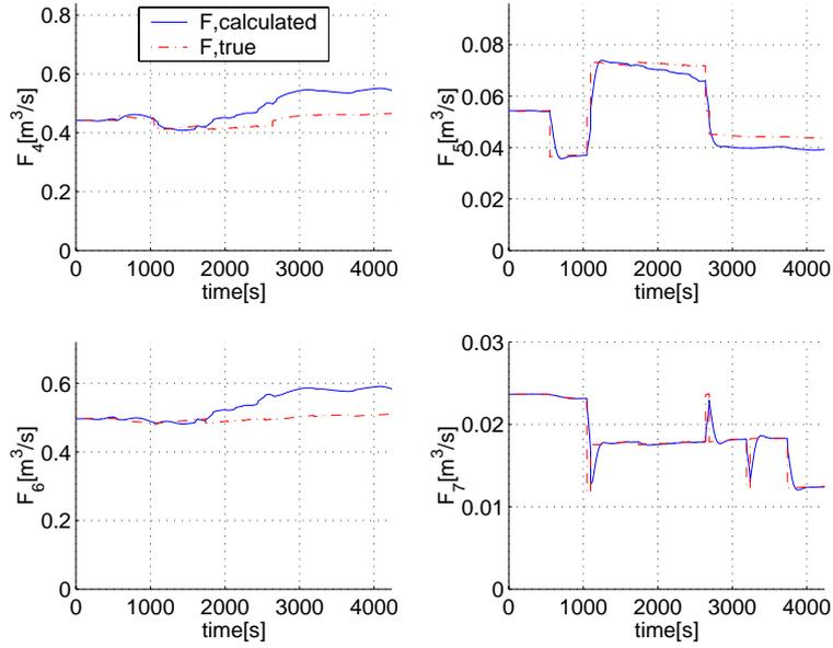
Figure 5.3: Flow in pipe 4, 5, 6 and 7 for clogging in pipe 4. (Solid for calculated and dashed for true flow).
