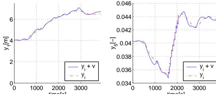
Figure 5.6: Sensor values for  $y_1$  and  $y_5$  for fault in sensor  $y_5$ .
