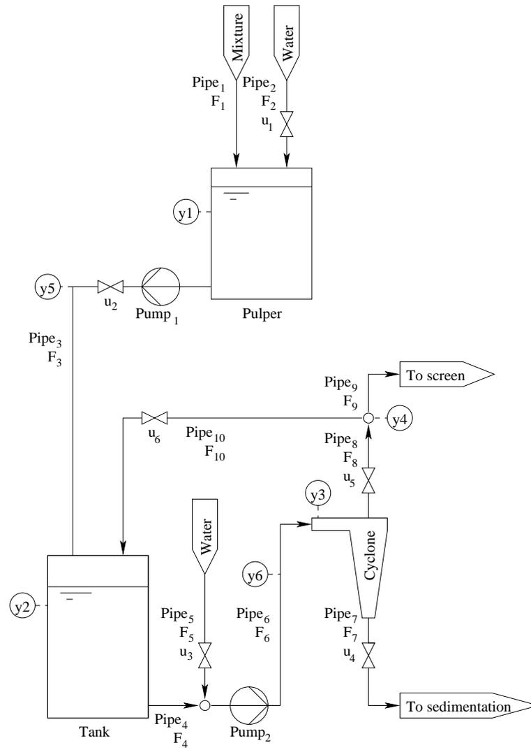
Figure 5.1: Schematic picture of stock preparation and broke treatment system.
