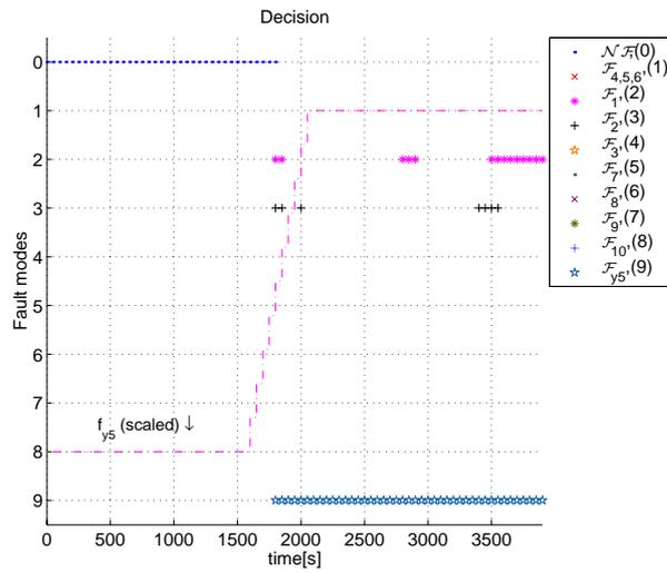
Figure 5.8: Decision for fault in sensor  $y_5$ .
