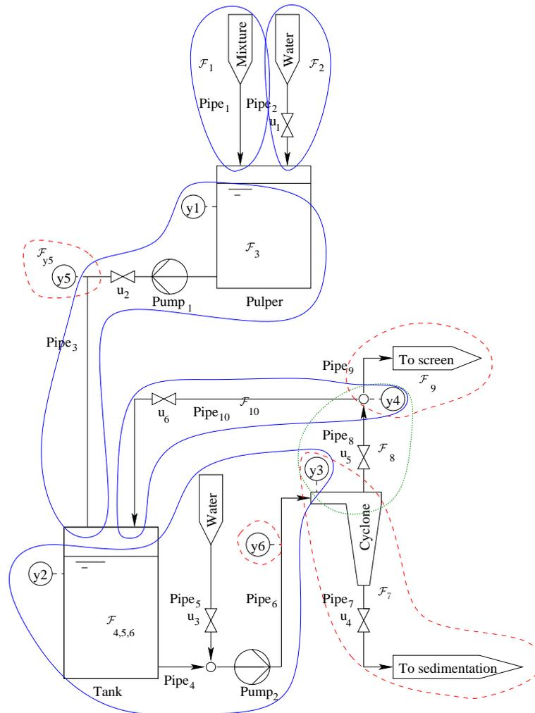
Figure 5.2: Fault modes for stock preparation and broke treatment system.
