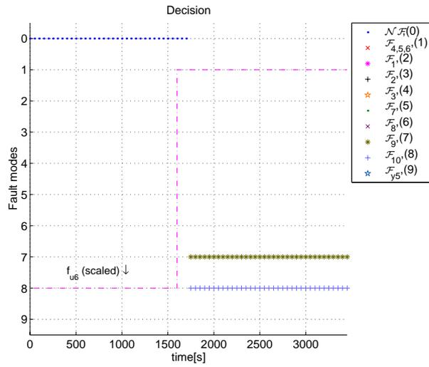
Figure 5.11: Decision for fault in actuator  $u_6$ .
