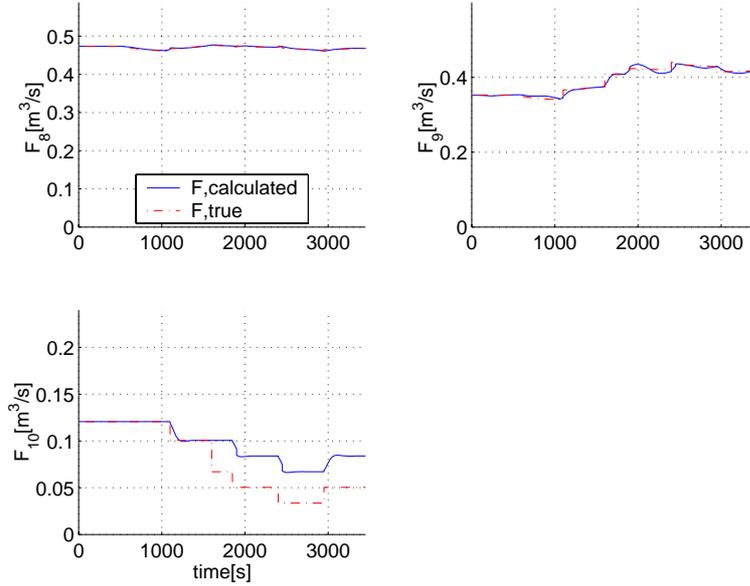
Figure 5.9: Flow in pipe 8,9 and 10 for fault in actuator  $u_6$ . (Solid for calculated and dashed for true flow).
