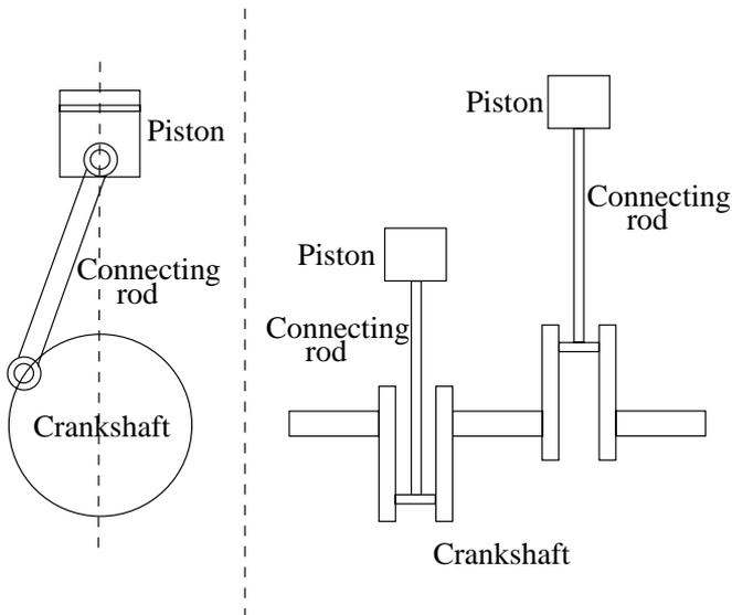
Figure 2.1: Description of the crankshaft and piston.
