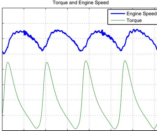
Figure 2.2: Engine Speed and Torque to illustrate the similarities between the two signals. The engine speed variations is greatly affected by the variations of the torque.
