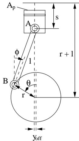
Figure 3.1: The crank-slider mechanism
