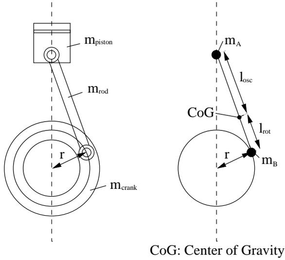
Figure 3.2: Two-mass model for oscillating and rotating masses
