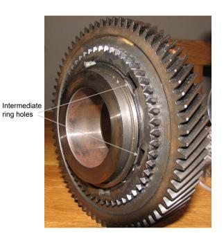
Figure 2.6. A gear wheel. Gear wheels are placed at the ends of the parts in figure 2.5. The intermediate ring hooks in figure 2.5 are hooked into the holes marked in this figure.
