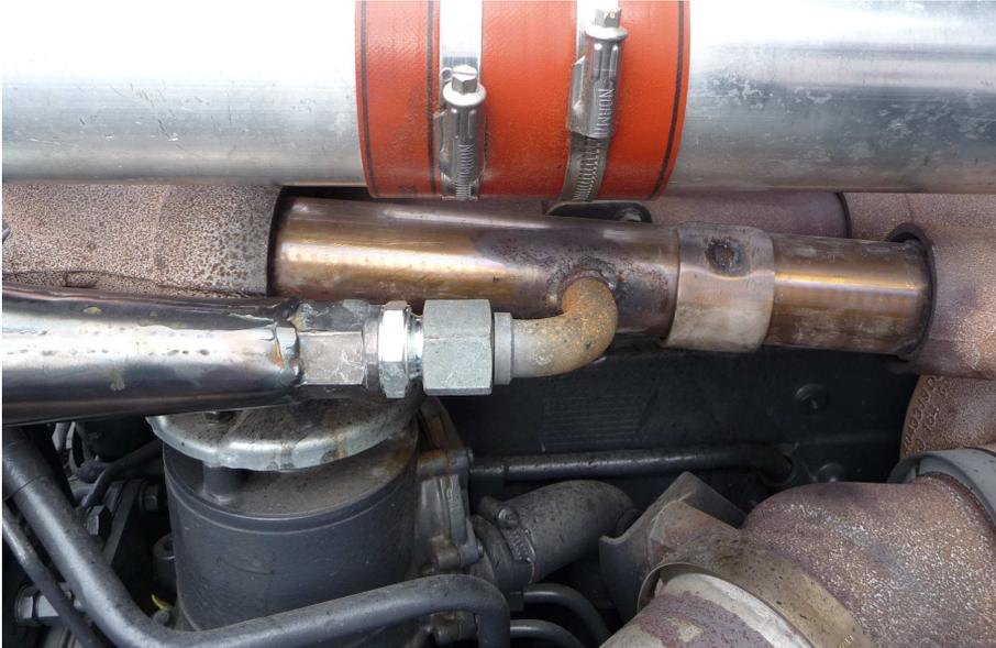
**Figure 4.5.** Closer view of the EGR leakage implementation. The bent pipe in the middle of the photo leads to the leakage bolt that is the splice between the two big screw nuts right after the bend.
