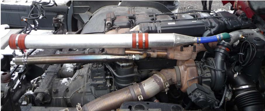
**Figure 4.3.** Overview of the new hardware for the leakage implementation in a truck. The upper of the two tubes in the middle of the photo is the tube for the gas from the boost-side leakage, and the lower is the tube for the gas from the exhaust-side leakage. For closeups of the holes, see Figure 4.4 for the boost-side, located to the right in the photo, and Figure 4.5 for the exhaust-side, located in the middle of the photo.
