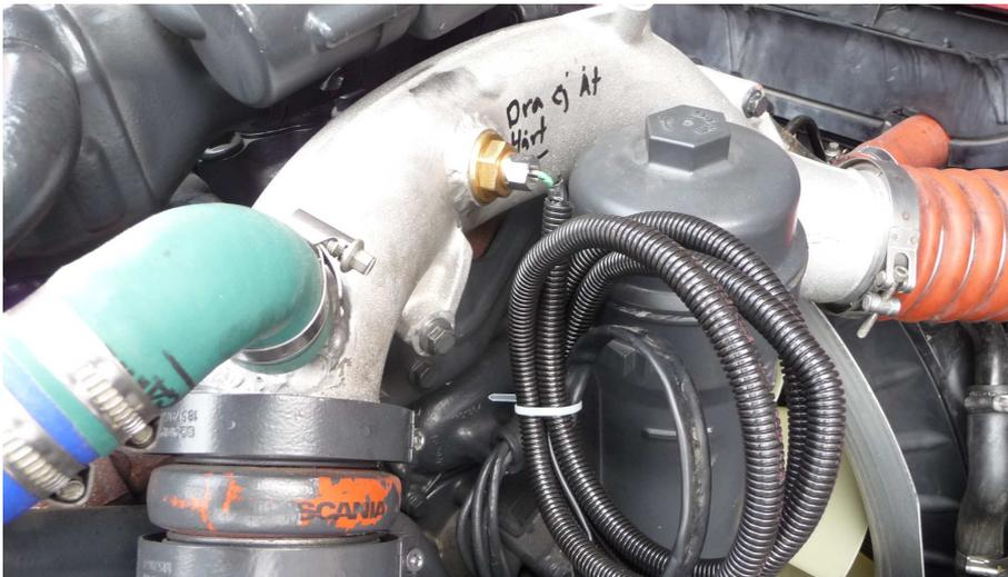
**Figure 4.4.** Closer view of the boost-side leakage implementation. The tube disappearing to the left encloses the leakage bolt. The extra pressure sensor can be seen in the middle of the photo with its rolled-up cable.
