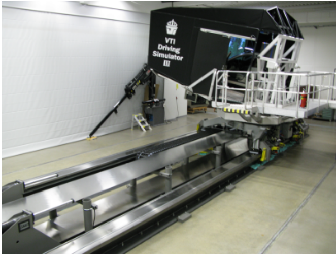
Figure 2.1. The SIM-3 lateral motion and cabin.
