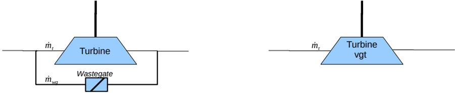
**Figure 3.2.** Turbine systems with wastegate for a gasoline engine to the left and a variable geometry turbine applied to a diesel engine to the right.
