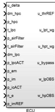
**Figure 6.1:** The input and output of the engine control unit. The signal nomenclature is explained in appendix B.
