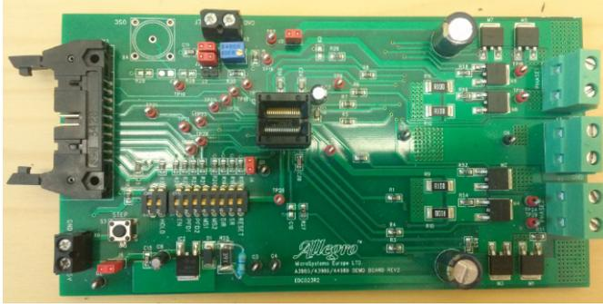
**Figure 4.2:** Allegro demo board used to drive the motor with desired settings.
