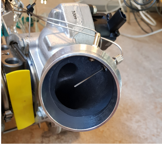
Figure 5.5: Compressor outlet where the gas temperature sensor, 23 is shown to be centred in the gas flow.
