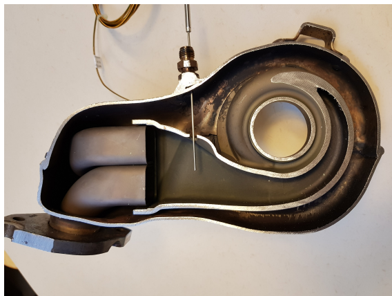
Figure 5.6: Turbine inlet cross-section showing how the gas temperature sensor is centred in the gas flow.
