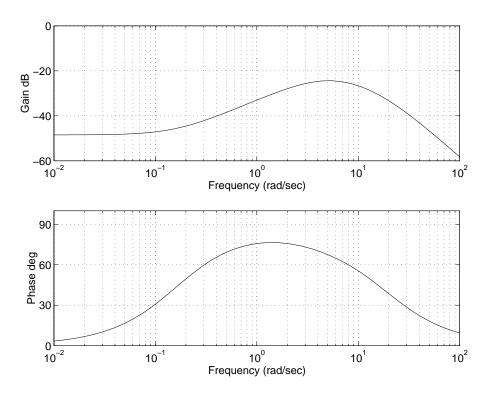
Figure 6.3. Bode plot of the inverted pendelum.
