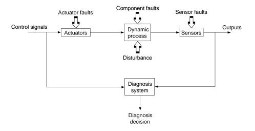
Figure 2.1. Structure of a diagnosis system.
