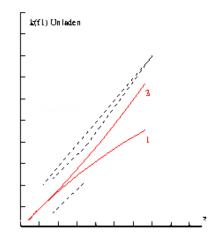
Figure 4.12: Friction utilization plot with 71/320/EEC tolerance drawn (dashed)
