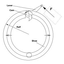
Figure 4.6: Drum brake schematic
