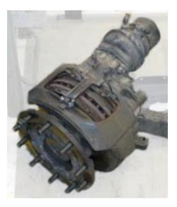
Figure 4.5: Disc brake with brake cylinder  $% \left( {{{\mathbf{F}}_{{\mathbf{F}}}} \right)$
