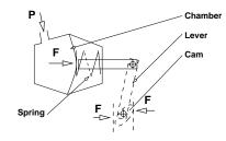
Figure 4.8: Brake cylinder schematic
