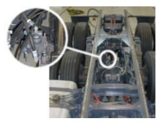
Figure 4.9: Load Sensing Valve (encircled)
