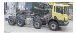
Figure 2.1: Eight-wheeled vehicle with two front axles
