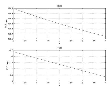
Figure 7: Bottom and top dead center as function of tilt angle
