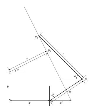
Figure 3: Definition of points and angles used in the derivation of the cylinder volume function
