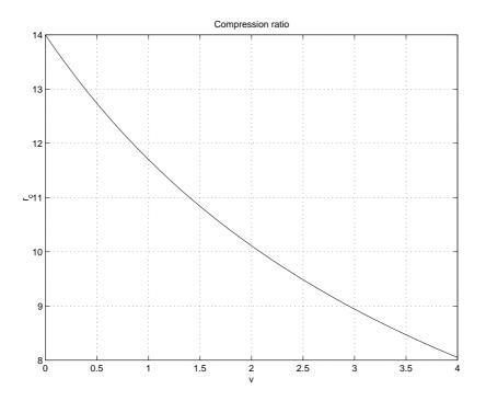
Figure 6: Compression ratio as function of tilt angle
