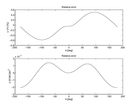
Figure 10: The crank angle degree has been adjusted to compensate for the deviation in TDC from  $\theta = 0$ , when simulating with the standard volume function. *Top:* Relative difference in volume between the standard volume function and the SVC volume function. *Bottom:* Difference in volume differential between the standard volume function and the SVC volume function.
