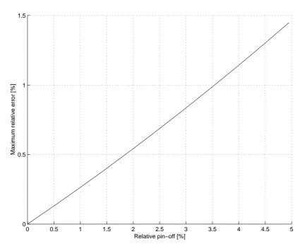
Figure 11: The relative error in volume at no tilt caused by neglecting the effect of pin-off. Relative pin-off is expressed in percentage of piston pin plus crank rod, i.e. relative pin-off =  $100 \cdot \frac{\text{pin-off}}{l+a}$ .
