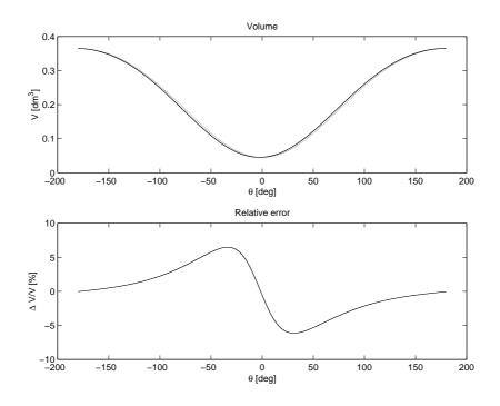
Figure 8: *Top:* Volume as function of crank angle at  $v = 4^{\circ}$ . The solid line is simulated with the SVC volume function and the dotted line simulated with a standard volume function. *Bottom:* Relative difference between the standard volume function and the SVC volume function, i.e.  $\frac{V_{std}-V_{SVC}}{V_{SVC}}$ .
