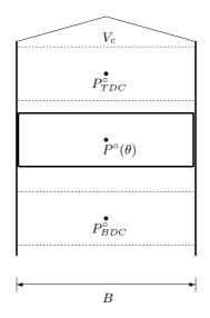
Figure 5: An engine cylinder with piston
