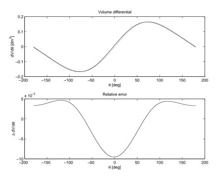
Figure 9: Top: Volume differential as function of crank angle at  $v = 4^{\circ}$ . The solid line is simulated with the SVC volume function and the dotted line simulated with a standard volume function. Bottom: Difference between the standard volume function and the SVC volume function, i.e.  $\frac{V_{std}-V_{SVC}}{V_{SVC}}$
