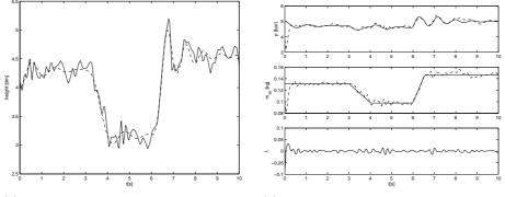
(a) Height of bellows during simulation. The solid line is the measured height and the dashed the true height.
