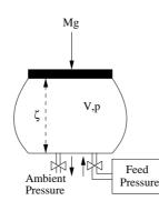
Figure 1: Principle sketch of the bellows.
