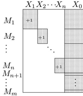
Figure 2: A structural decomposition of a PSO set.
