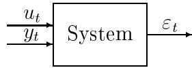
Figure 4.1: A whitening filter takes the observed input u_t and output y_t and transforms them to a sequence of residuals \varepsilon_t .
